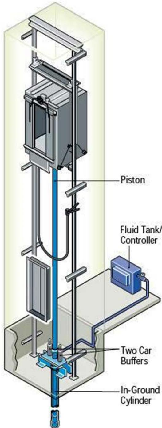
**Figure B-3 Hole-less, Dual Post, Direct Plunger Hydraulic Elevator**
