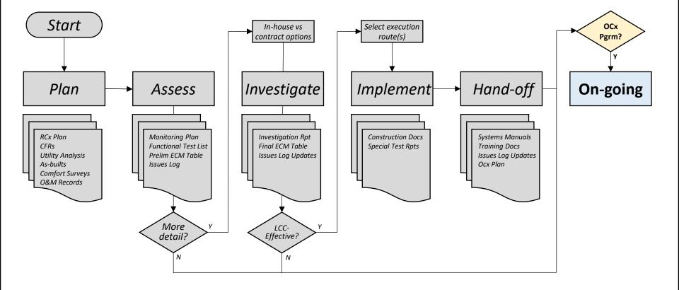
The goal of OCx is to continuously monitor specific facility performance metrics and have a plan for keeping buildings on track
