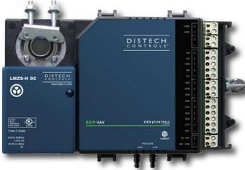
**1A-VAV:** VAV box controller with multiple analog inputs and outputs. Also incorporates dedicated actuator and pressure sensor (normally Tier 0 devices). Network is LonTalk over TP/FT-10 media at 78 Kbps.
