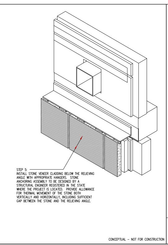
The dimensions and material relationships shown in this detail are <u>not to scale</u> and have been exaggerated for clarity. Actual dimensions will vary, and should be carefully coordinated with sequencing and construction tolerances to ensure the long-term durability and performance of this and similar exterior wall details.
