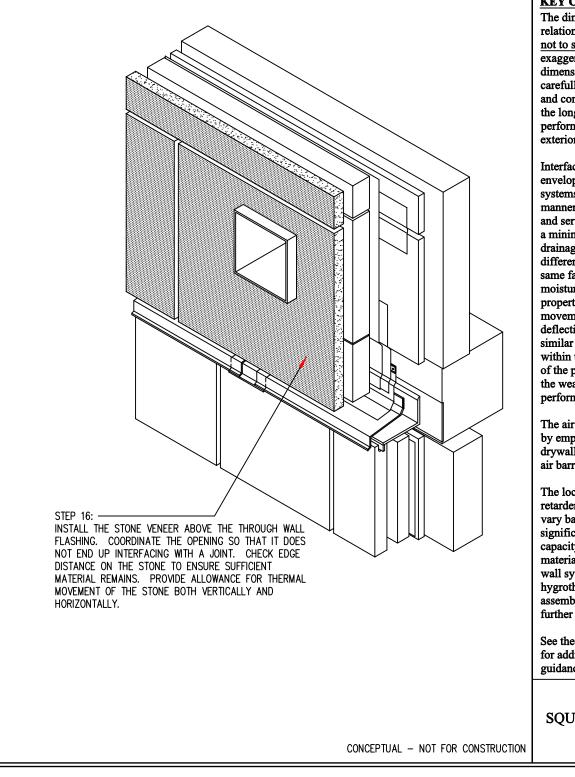
The dimensions and material relationships shown in this detail are <u>not to scale</u> and have been exaggerated for clarity. Actual dimensions will vary, and should be carefully coordinated with sequencing and construction tolerances to ensure the long-term durability and performance of this and similar exterior wall details.
