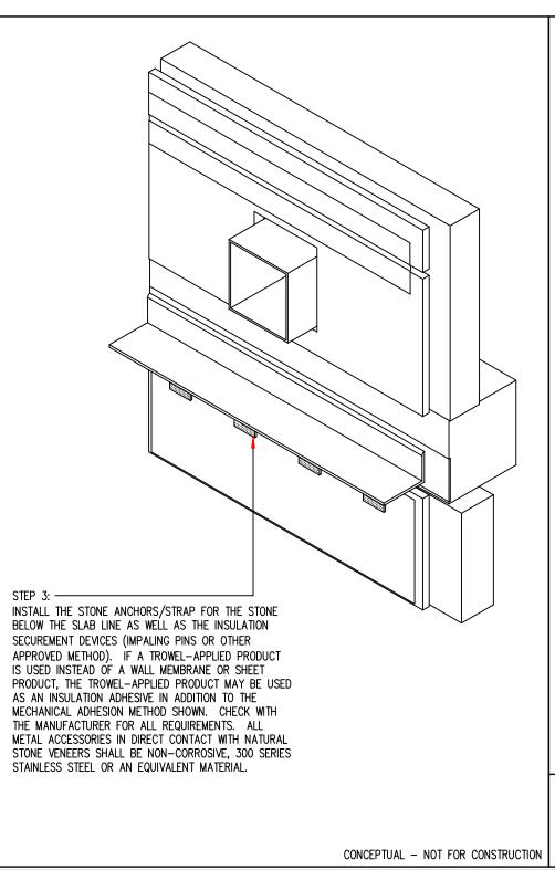
The dimensions and material relationships shown in this detail are <u>not to scale</u> and have been exaggerated for clarity. Actual dimensions will vary, and should be carefully coordinated with sequencing and construction tolerances to ensure the long-term durability and performance of this and similar exterior wall details.
