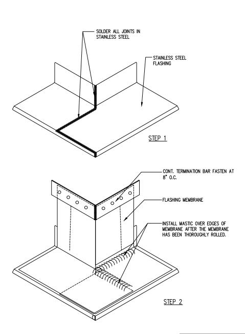
NOTE: SPLICES IN METAL FLASHING MUST BE LOCATED A MIN. OF 2'-6" FROM CORNER FLASHING PIECE.
