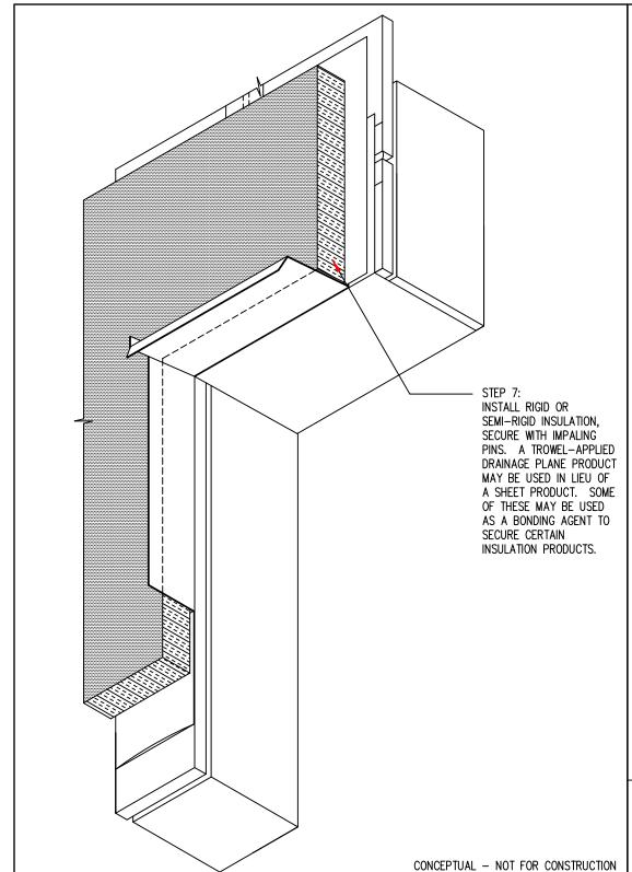
The dimensions and material relationships shown in this detail are not to scale and have been exaggerated for clarity. Actual dimensions will vary, and should be carefully coordinated with sequencing and construction tolerances to ensure the long-term durability and performance of this and similar exterior wall details.
