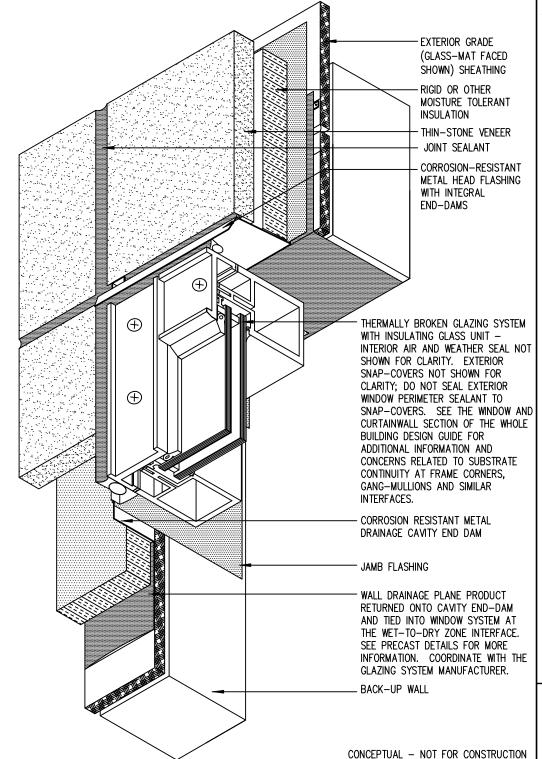
The dimensions and material relationships shown in this detail are not to scale and have been exaggerated for clarity. Actual dimensions will vary, and should be carefully coordinated with sequencing and construction tolerances to ensure the long-term durability and performance of this and similar exterior wall details.
