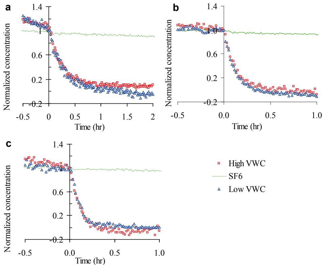
**Figure 3-5. Normalized toluene concentration at different air flow rate: (a) 250 m<sup>3</sup>/h airflow rate passing the bed, (b) 600 m<sup>3</sup>/h airflow rate, (c) 930 m<sup>3</sup>/h air flow rate. Volumetric water content (VWC) in the filter bed.**
