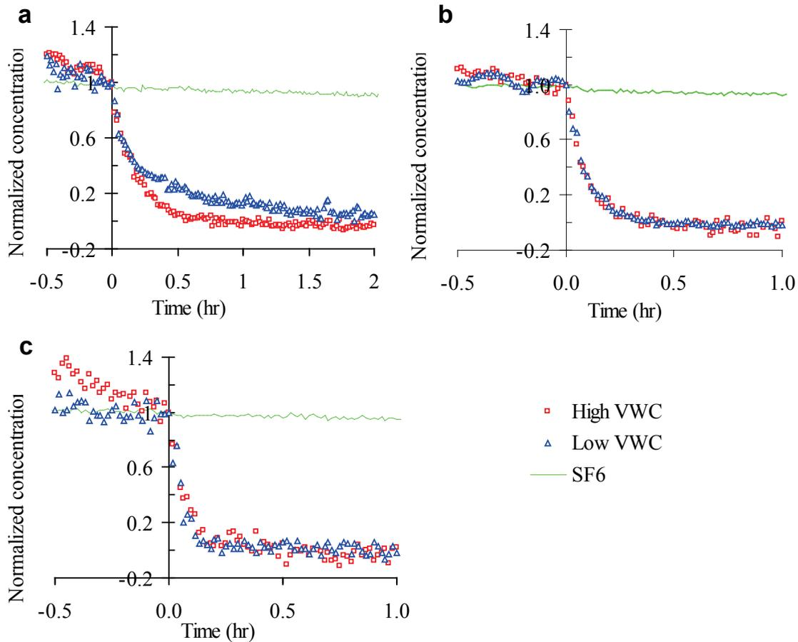
**Figure 3-4. Normalized formaldehyde concentration at different air flow rate: (a) 250 m<sup>3</sup>/h airflow rate passing the bed, (b) 600 m<sup>3</sup>/h airflow rate, (c) 930 m<sup>3</sup>/h air flow rate. Volumetric water content (VWC) in the filter bed.**
