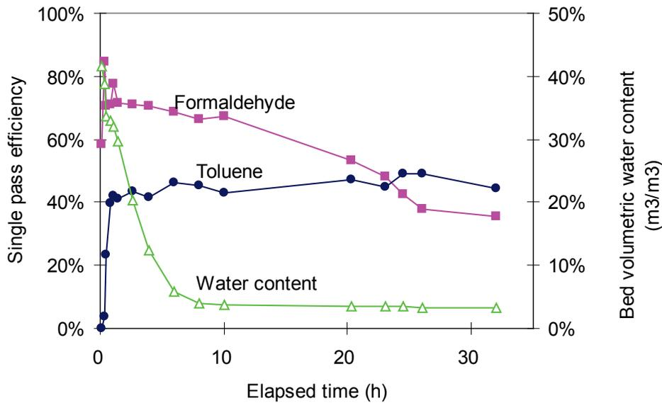
**Figure 4-4. Effect of bed water content on removal of pollutants**
