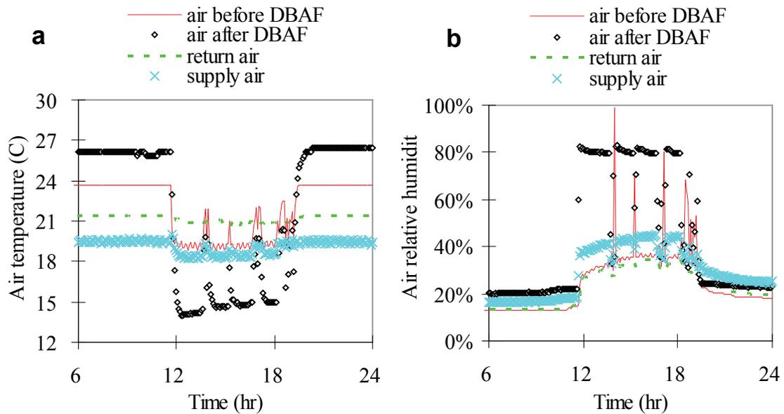
Figure 4-2 Effect of DBAF on room air temperature and RH: (a) Temperature, (b) RH.
