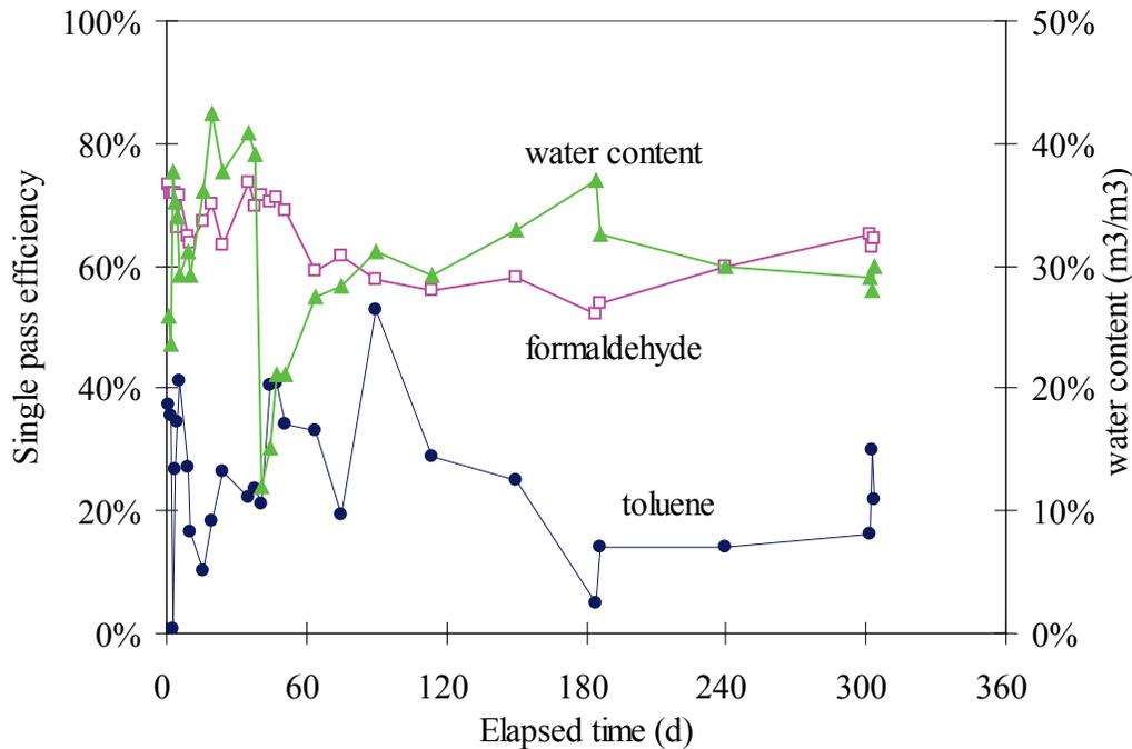
**Figure 4-5. Botanical filter single pass efficiency (SPE) over 300 days**
