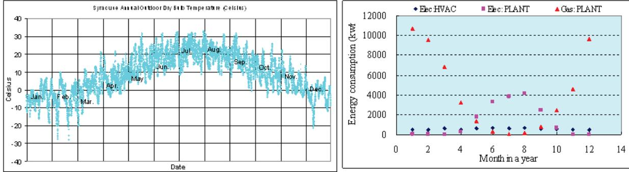
**Figure 5-2. Yearly outdoor temperature at Syracuse and building HVAC energy consumption**
