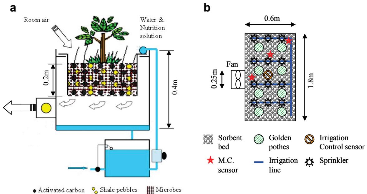
**Figure 3-2. Schematic of dynamic botanical air filtration system: (a) side view, (b) top view. Moisture content sensor (M.C. sensor)[22].**
