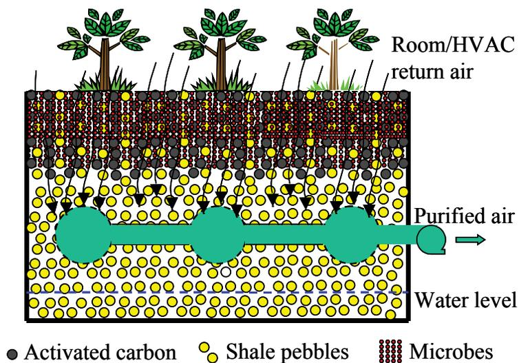
**Figure 1-1. Principle of a Wolverton filtration system**
