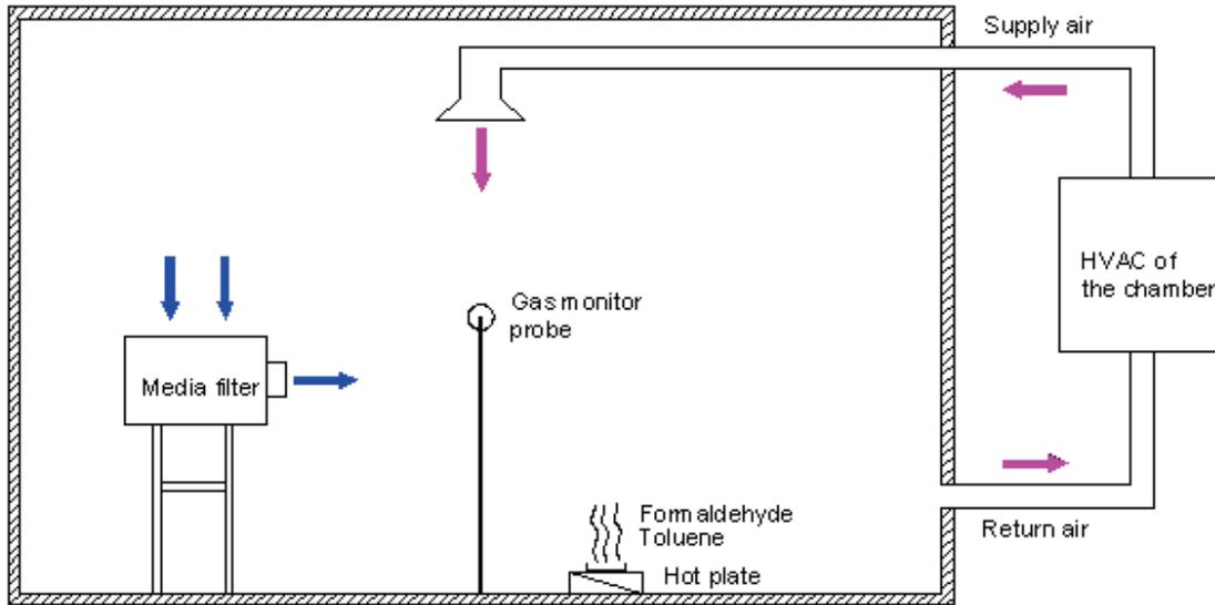
**Figure A-2. Schematics of the test chamber**
