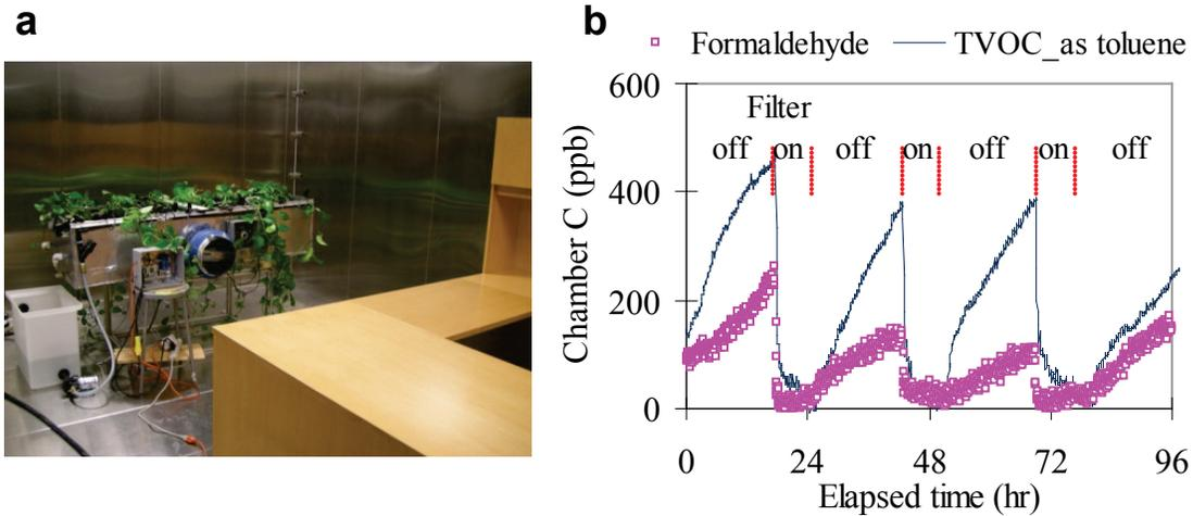
Figure 3-6. Test set-up and test chamber concentration vary with time: (a) test set-up (photo), (b) test results.
