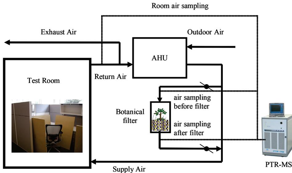
**Figure 4-1. Integration of botanical filter into an HVAC system and setup for monitoring. Air handling unit (AHU). Proton Transfer Reaction Mass Spectrometer (PTR-MS).**
