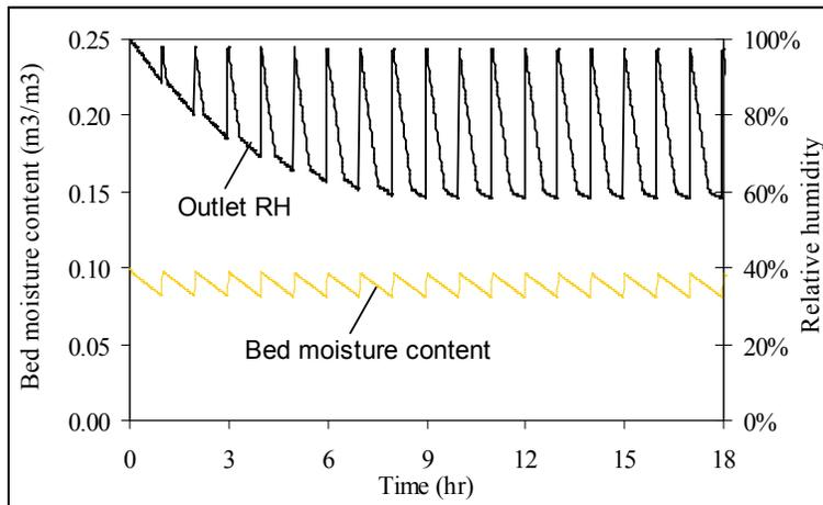
**Figure 6-2. Bed average moisture content and outlet air relative humidity**
