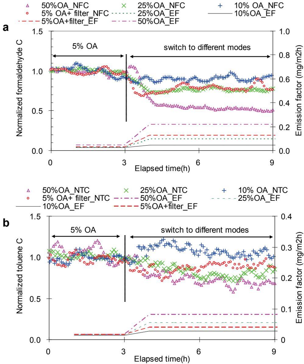
**Figure 4-3. Comparison of room pollutants concentration: (a) Formaldehyde, (b) Toluene. Outdoor air (OA). Normalized formaldehyde concentration (NFC). Emission factor (EF). Normalized toluene concentration (NTC).**
