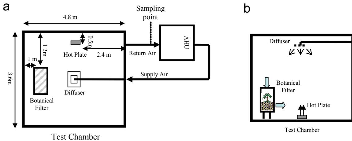
**Figure 3-3. Schematic of the environmental chamber test setup: (a) top-view, (b) side-view. Air handling unit (AHU).**
