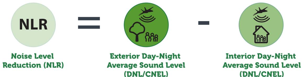
Sound travels from the exterior to the interior of a building by penetrating the building perimeter through the building's solid structural elements or via openings. Openings in the building (which provide air infiltration paths through windows, vents, and gaps) allow sound to travel directly into the building's interior. Basically, any place that air enters a home, sound will also enter.
