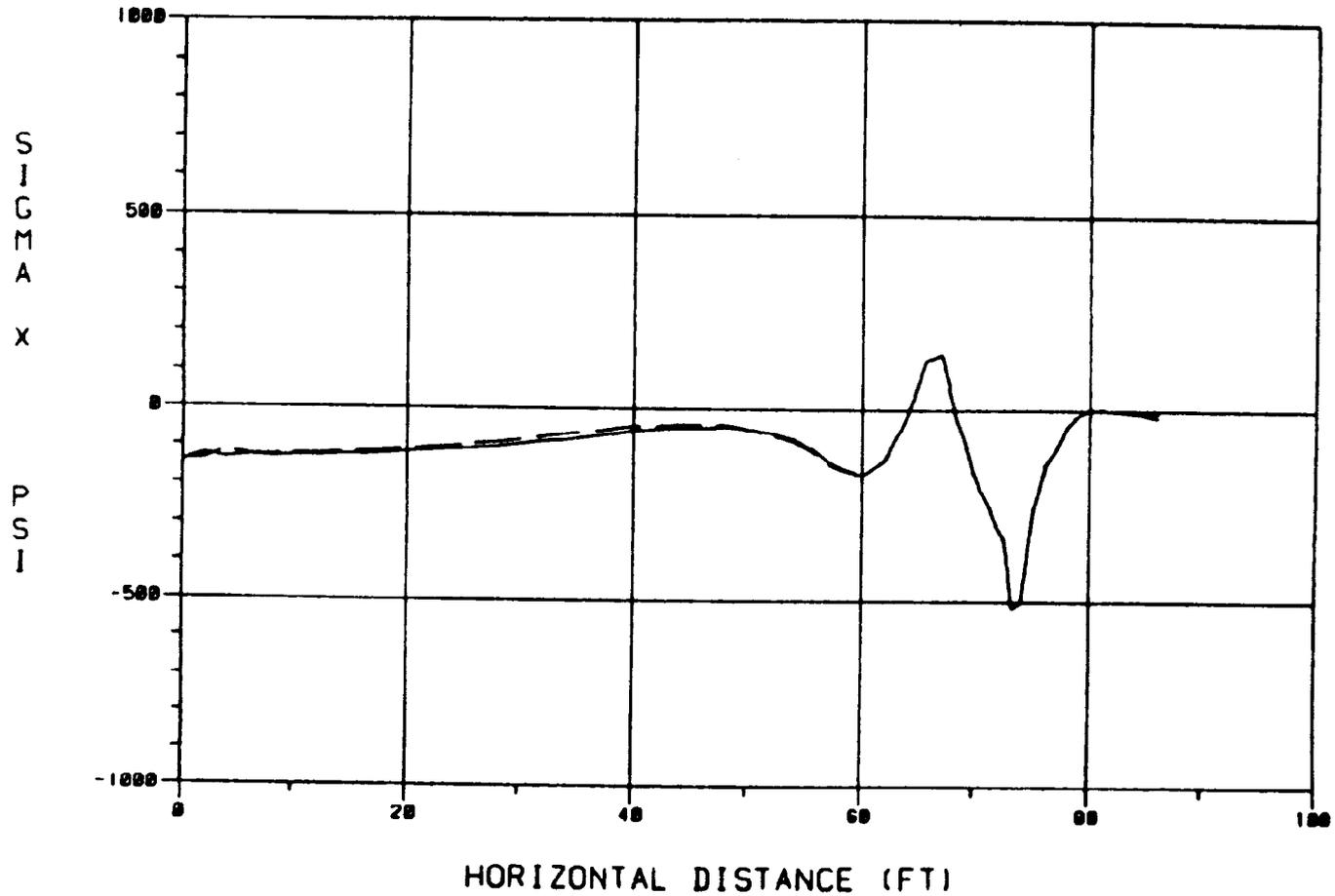
Fig. 5. Sigma-X Stresses Along the Top of the Floor Slab - Model No. 1
