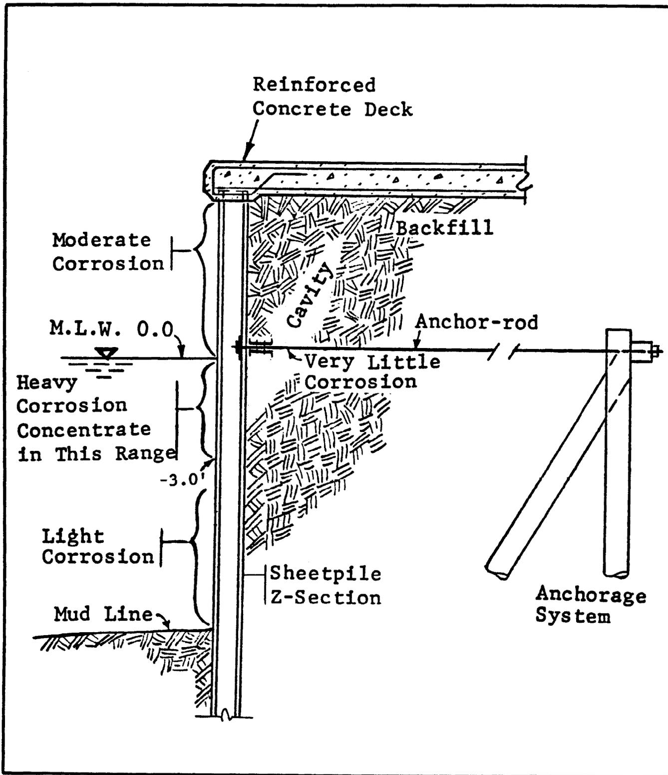
Fig. 2. Anchored Bulkhead After 25 Years in Service (Ref. 3)
