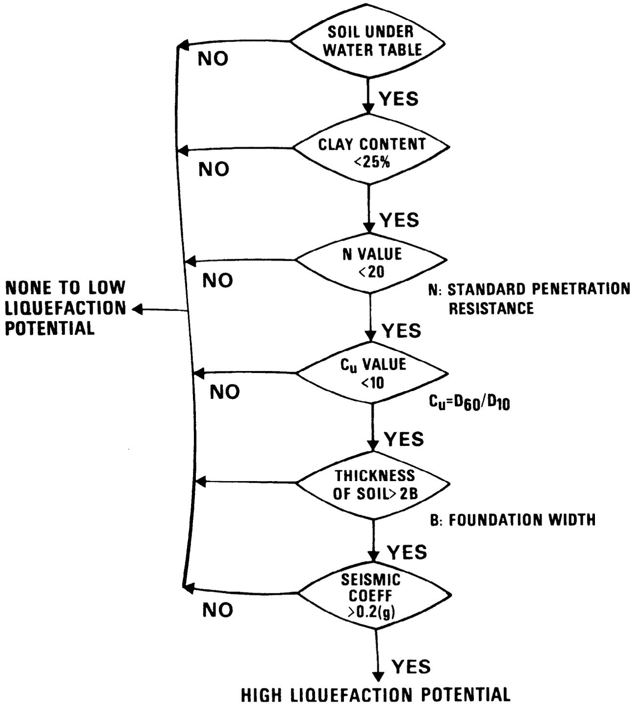
Fig. 7. Flow Chart for Checking Liquefaction Potential
