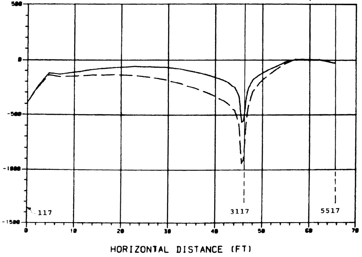
Fig. 6. Sigma-X Stresses Along the Top of the Floor Slab - FEM Model No. 2A
