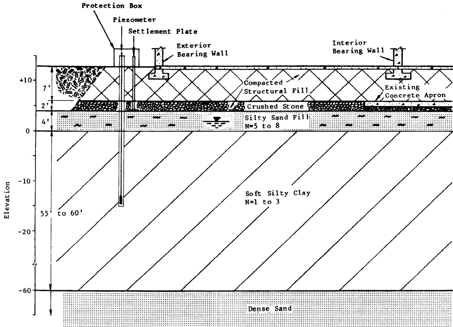
Fig. 1. Compacted fill was placed on a two feet thick layer of crushed stone. In the area where concrete apron existed, it was left in place to substitute for crushed stone base. Foundation soils are 4 feet of recent medium dense sand fill, which is underlain by 55 to 60 feet (17 to 18 m) thick, highly compressible clay.
