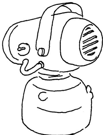
Hand-held cold foggers are used inside buildings where they fill rooms, small warehouses, etc., with aerosol droplets. These floating droplets kill flying insects as well as exposed insects on horizontal surfaces. Fogs do not enter tight spaces or cracks and crevices. While some aerosol generators are used for crack and crevice applications, they also produce aerosol droplets that float in the air.
