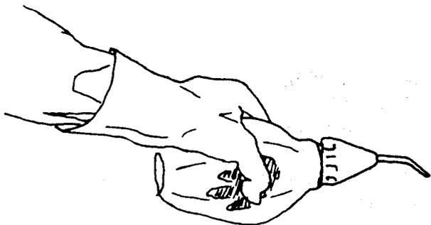
Three types of hand dusters are commonly used by pest management technicians: bulb, bellows, and plunger dusters. Dusts are also driven by gas in some formulations of canned insecticides, but with this method, dusts are applied like canned liquid pesticides.
