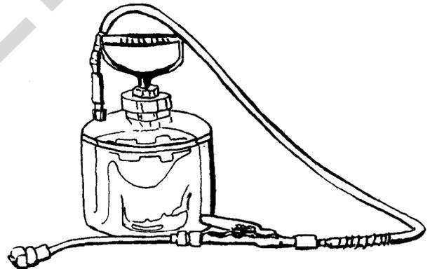
The small (one or two gallon) stainless steel spray tank is the workhorse of pest control. It is the tool most familiar to pest control technicians. It can be used in many different ways (and by many different industries). In pest management, the “spray tank” is used to apply a flushing agent, or a residual pesticide. Depending on the nozzle selection, it applies different spray patterns; and depending on the amount of pumping, it delivers the pesticide under high or low pressure.
