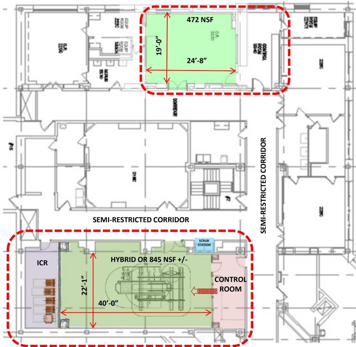
CURRENT ENDOVASCULAR PROCEDURE ROOM **INADEQUATE** IN SIZE TO MEET CRITERIA FOR HYBRID OR EVAR AND/OR TAVR PROCEDURES
