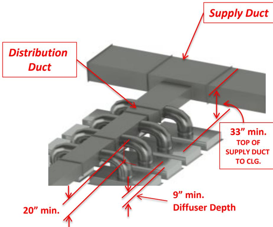
*“Traditional Laminar Array System Depth Typical Depth Utilizing 10” diameter hard duct”
