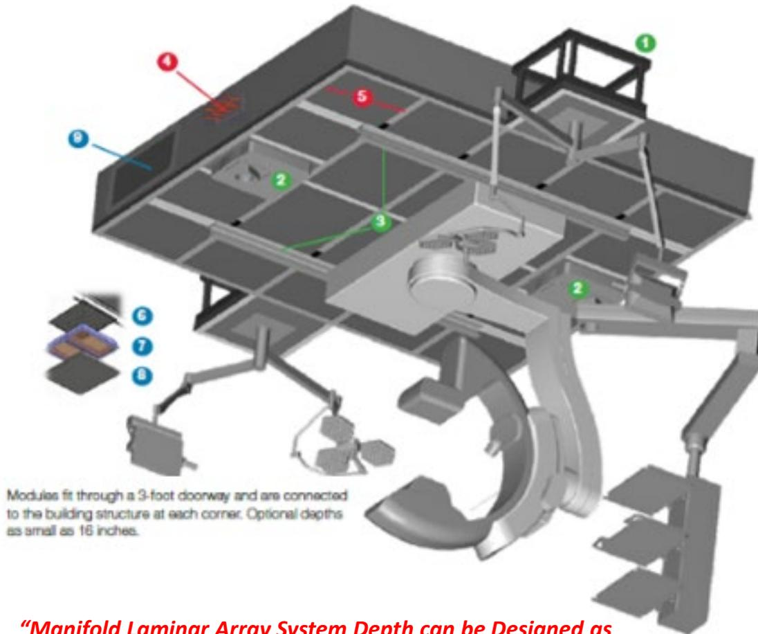
Modules fit through a 3-foot doorway and are connected to the building structure at each corner. Optional depths as small as 16 inches.
