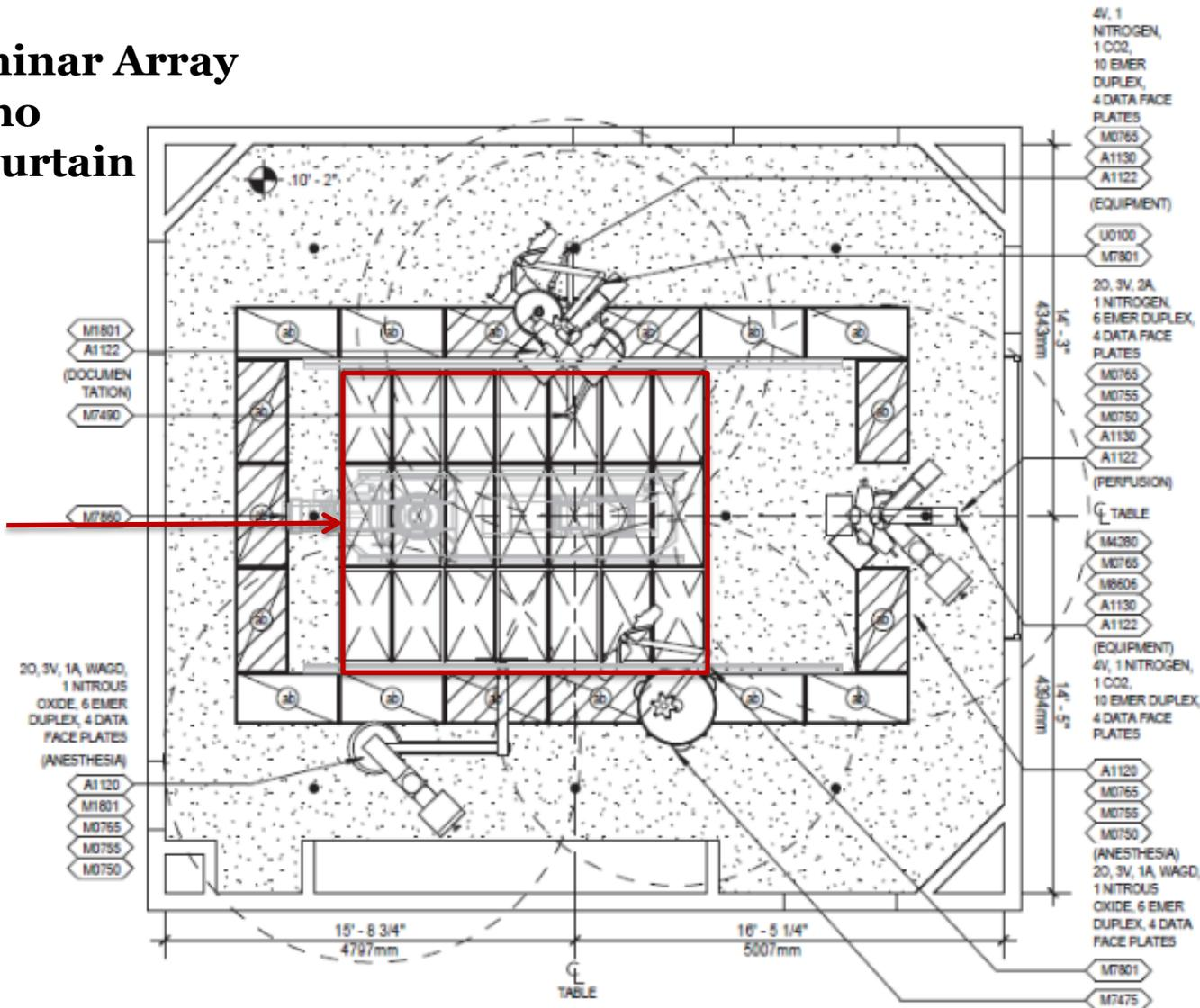
*Laminar Flow Array Over the sterile field Imaging Equipment Gantry Creates Turbulence.*
