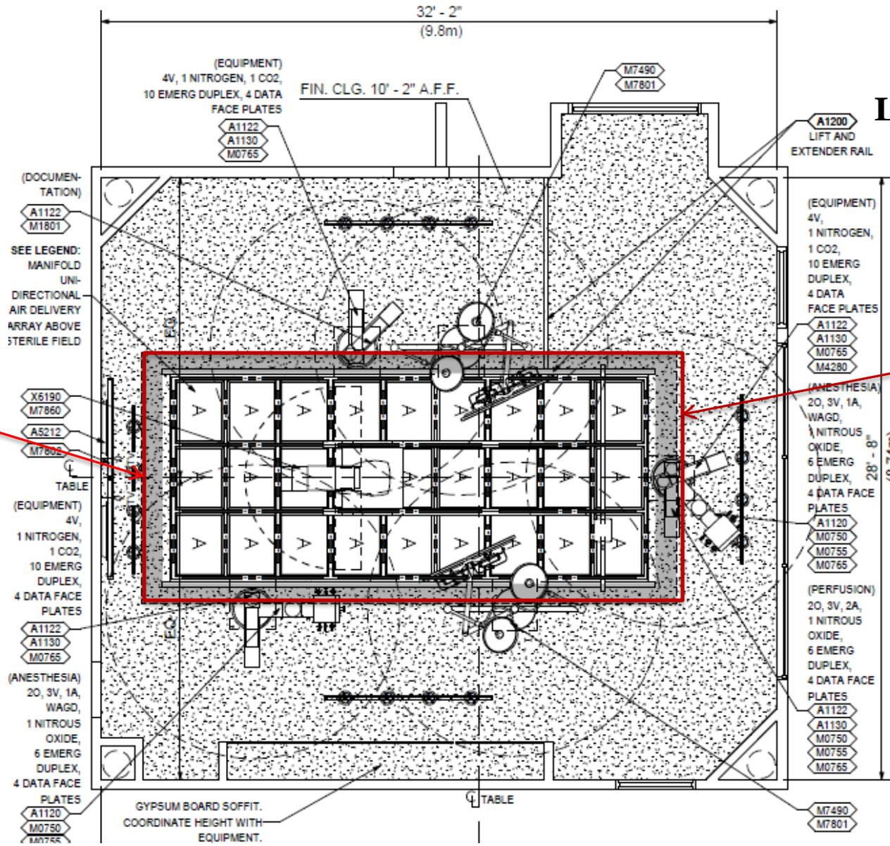
**BOUNDARY of STERILE FIELD And LAMINAR FLOW ARRAY**
