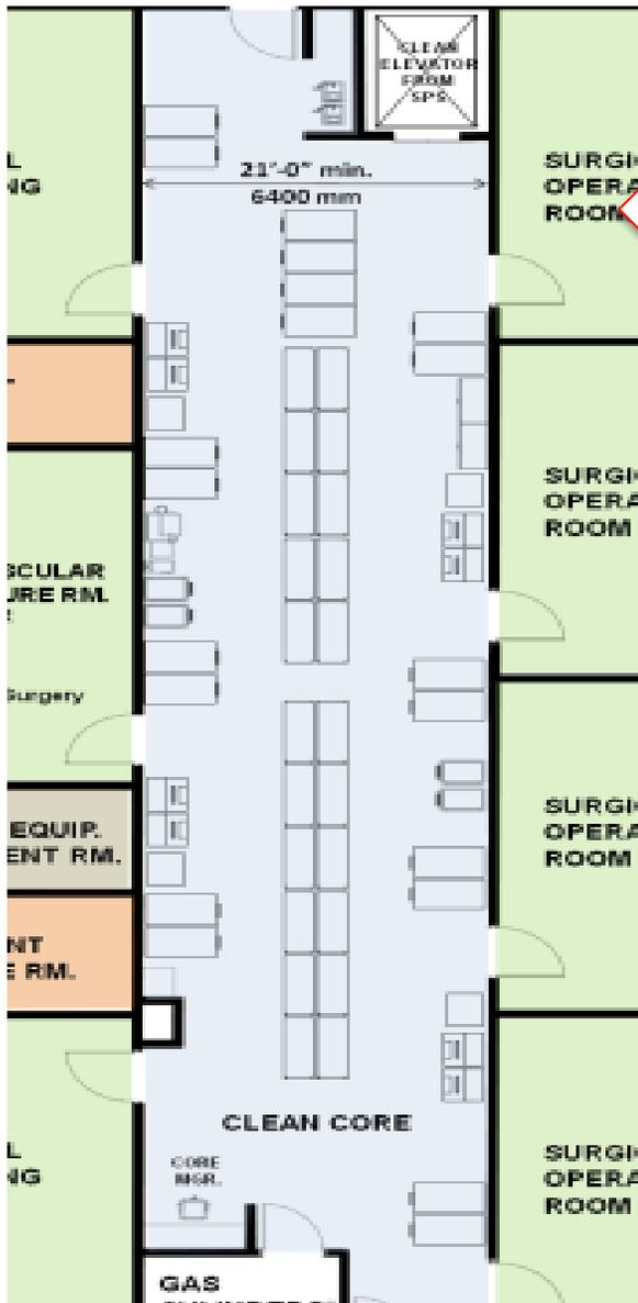
Clean core configuration utilizing a width of 21'-0" (6401 mm) servicing an integrated interventional platform consisted of both surgical and endovascular procedure rooms.
