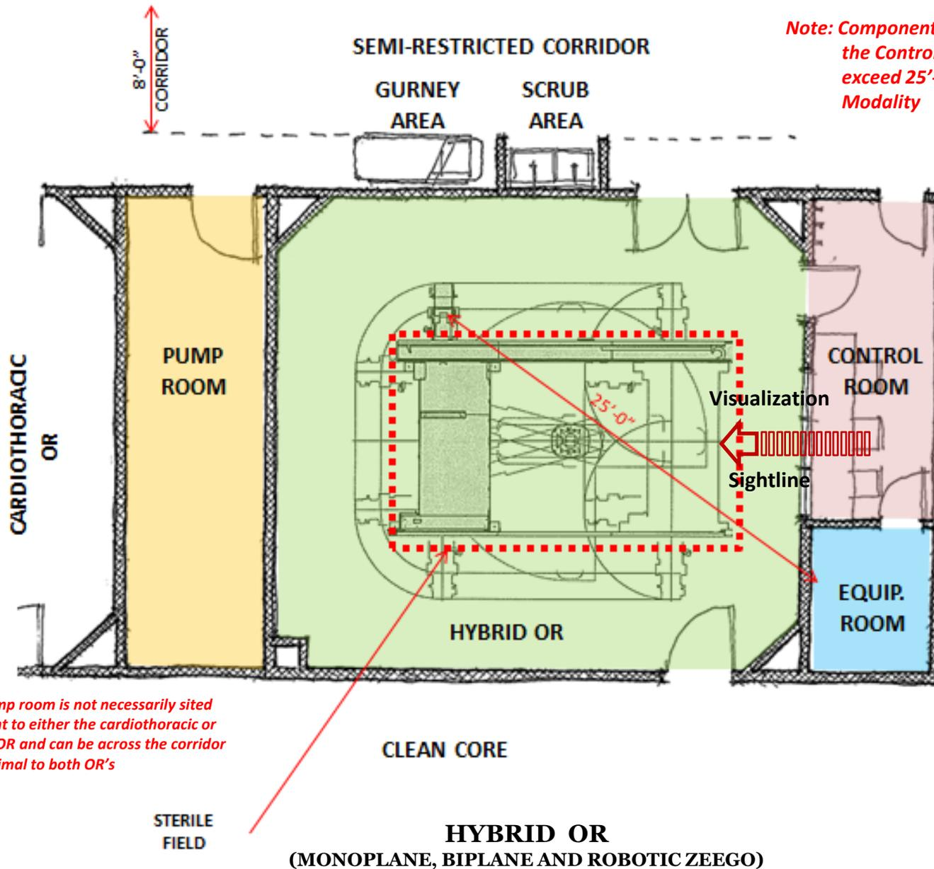
*Note: Component Equipment Room Accessible from the Control Room, Cable lengths must not exceed 25'-0" from ICR panel to the Imaging Modality*
