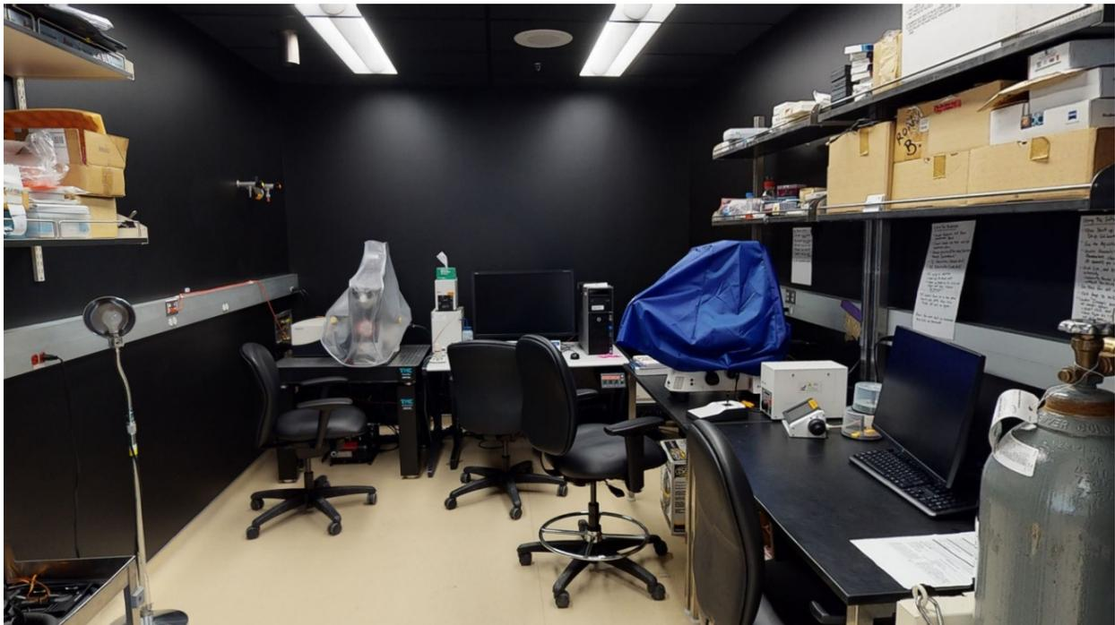
*Figure 24 The Microscopy Room at the Rocky Mountain VAMC R&D Facility provides a dark environment with no windows and black walls. A vibration-isolation table is provided for the high-resolution microscope.*
