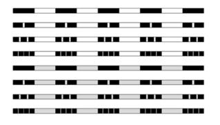
FIRE RESISTIVE RATED WALLS, 1 HOUR FIRE RESISTIVE RATED WALLS, 2 HOUR FIRE RESISTIVE RATED WALLS, 3 HOUR FIRE RESISTIVE RATED WALLS, 4 HOUR FIRE RATED, SMOKE BARRIER WALLS, 1 HOUR FIRE RATED, SMOKE BARRIER WALLS, 2 HOUR FIRE RATED, SMOKE BARRIER WALLS, 3 HOUR FIRE RATED, SMOKE BARRIER WALLS, 4 HOUR
