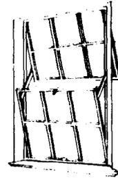
*Pivot windows* were an early type of industrial window that combined inexpensive first cost and low maintenance. Pivot windows became standard for warehouses and power plants where the lack of screens was not a problem. The window shown here is a horizontal pivot. Windows that turned about a vertical axis were also manufactured (often of iron). Such vertical pivots are rare today.
