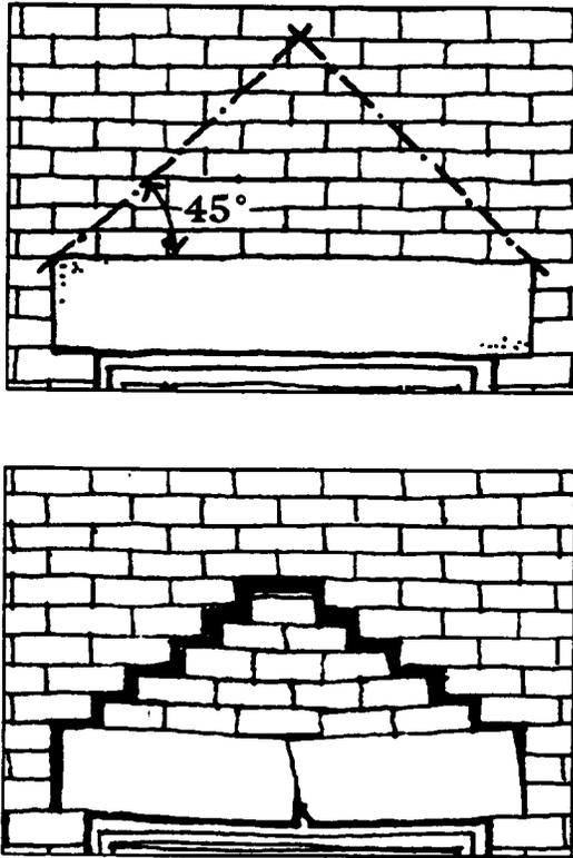
Figure 4-14. The Collapse of Masonry Lintels Indicates a Structural Fault.
