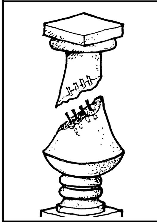
Figure 4-4. Blind Reattachment of Broken Stone.
