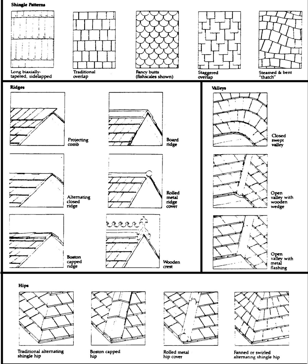
Figure 4-17. Wooden Shingles -- Historic Details and Installation Patterns.
