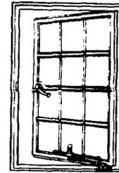
*Projecting windows*, sometimes called awning or hopper windows, were perfected in the 1920s for industrial and institutional buildings. They were often used in "combination" windows, in which upper panels opened out and lower panels opened in. Since each movable panel projected to one side of the frame only, unlike pivot windows, for example, screens could be introduced.
