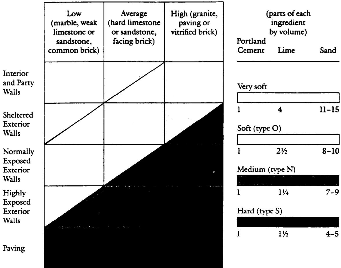
Figure 4-5. Guide to Mortar Mixes (Relative Mortar Strength) .
