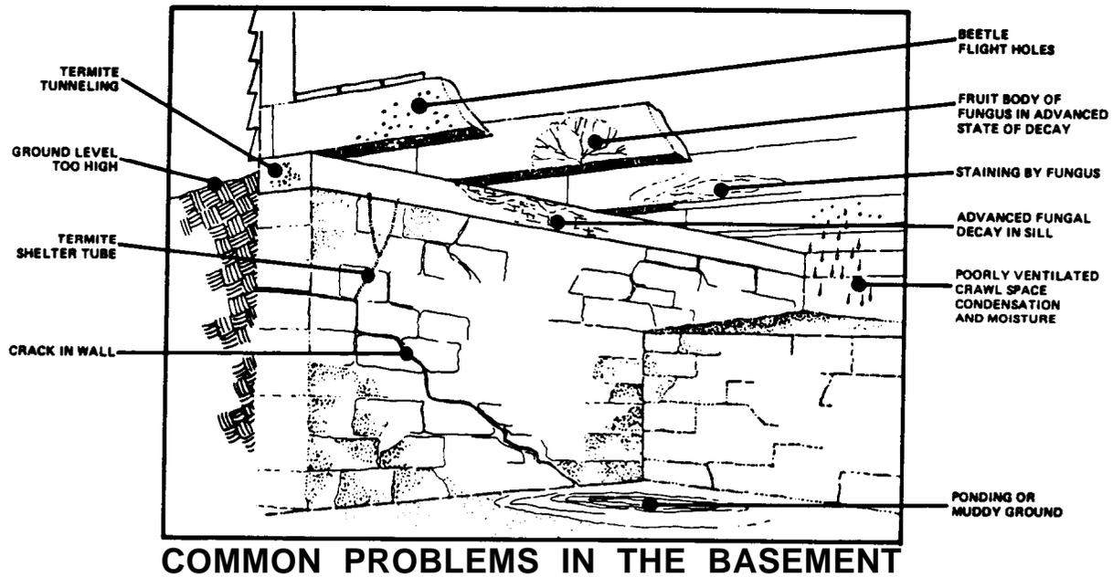
Figure 4-12. Common Problems in the Basement.
