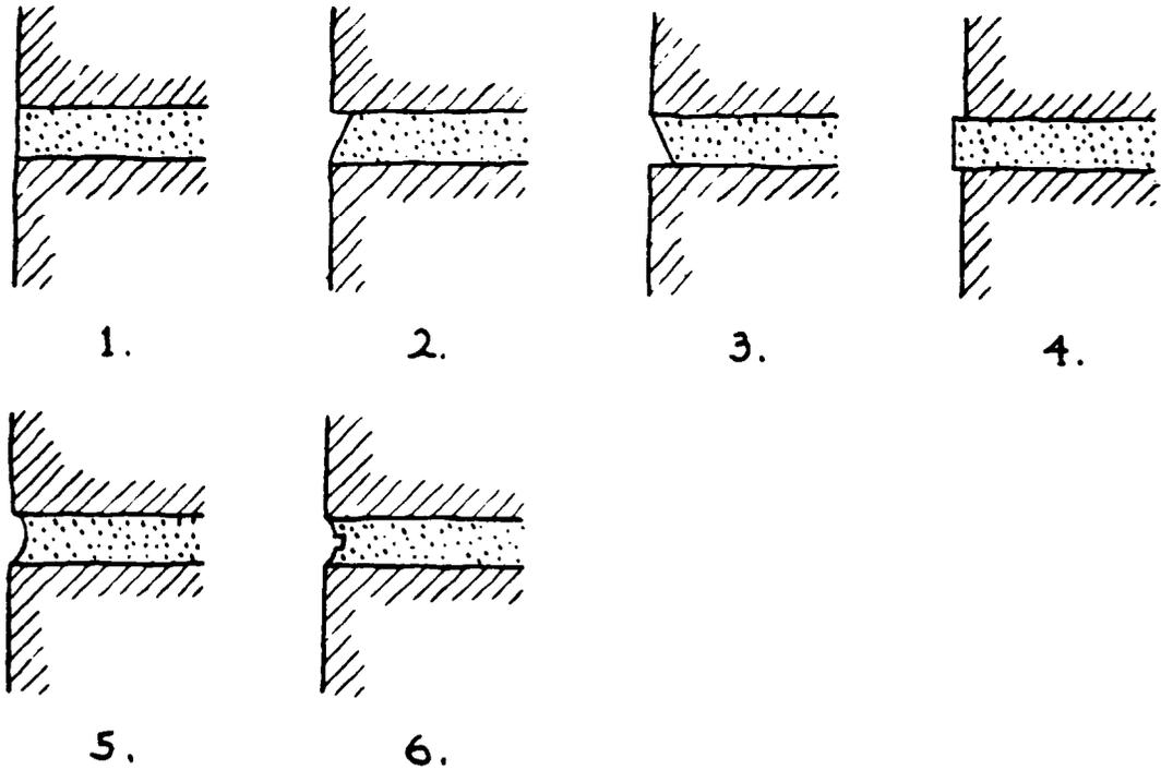
Figure 4-6. Brick Joints.
