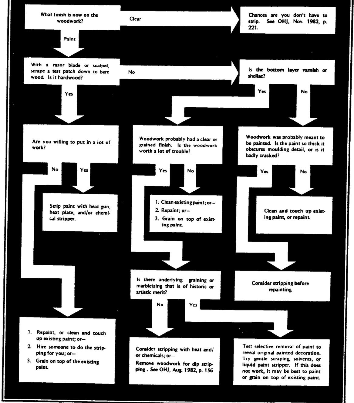
Figure 4-24. Architectural Woodwork: To Strip or Not To Strip?
