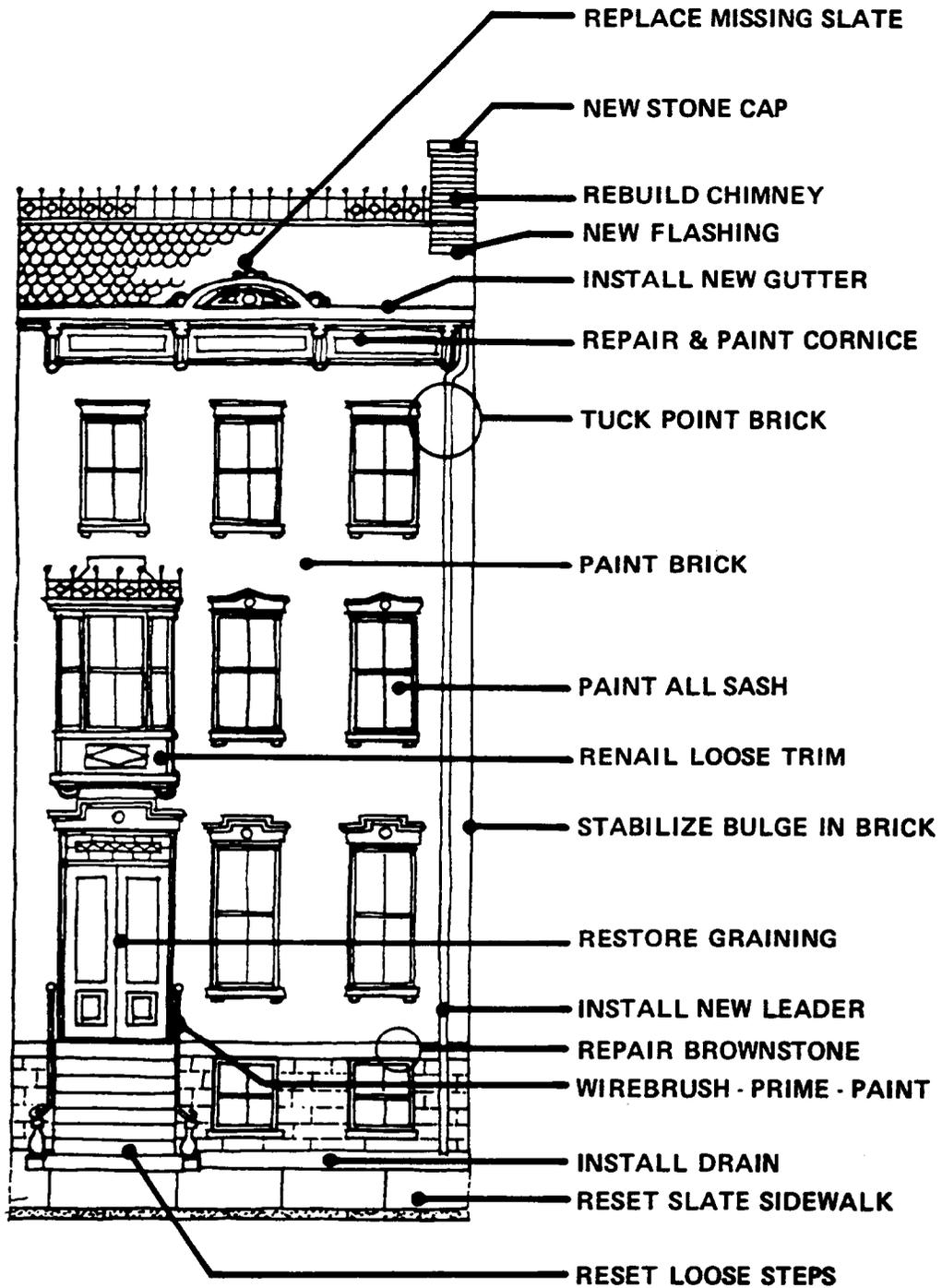
Figure 3-2. Typical Work Involved in Rehabilitating a Historic Structure.
