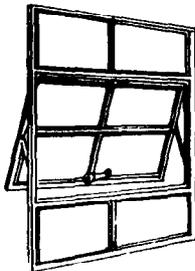
*Continuous windows* were almost exclusively used for industrial buildings requiring high overhead lighting. Long runs of clerestory windows operated by mechanical tension rod gears were typical. Long banks of continuous windows were possible because the frames for such windows were often structural elements of the building.
