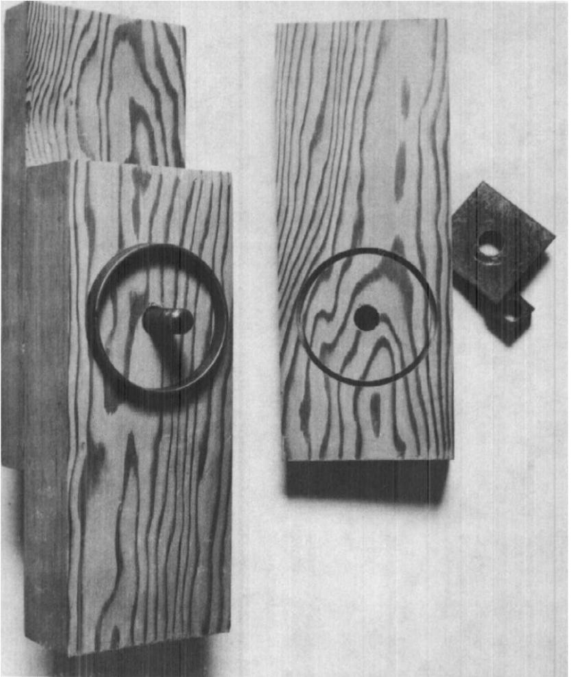
Figure 2-1. A split-ring connector installed in one member. The facing member has been drilled to receive the connector. Where the joint between facing members is not tight, probe through the connection with a thin metal to determine if the connector was installed or not.
