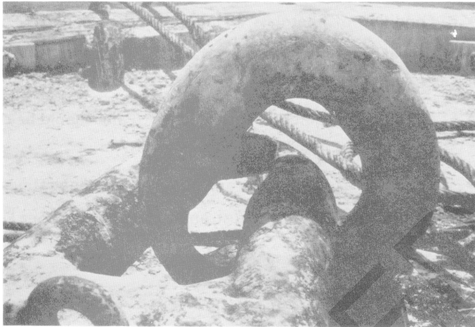
Figure 3-1. An Example of Severely Worn Top Jewelry
