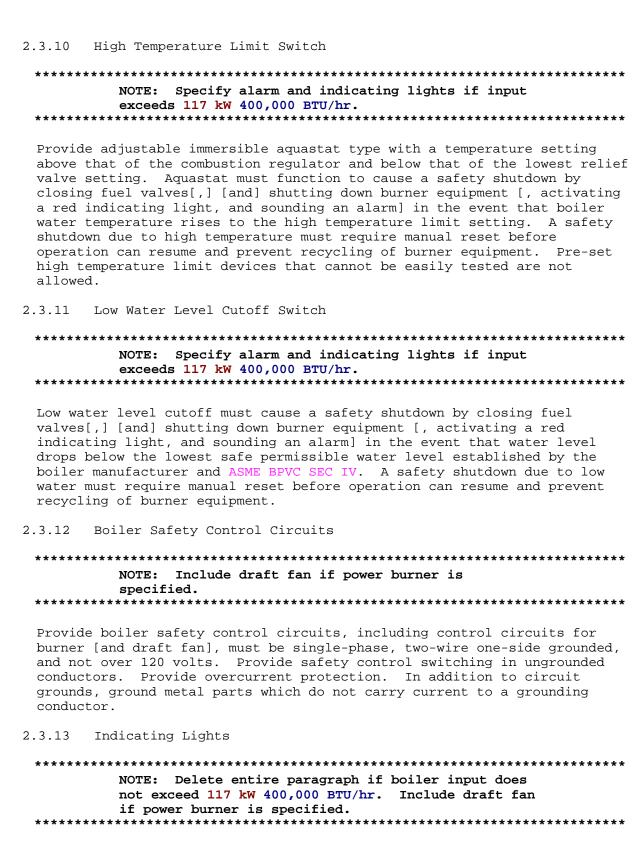
Each safety interlock requiring a manual reset must have an individually labeled red indicating light. Non-recycling control interlocks must have the reset located on the control itself. Red indicating lights on the
