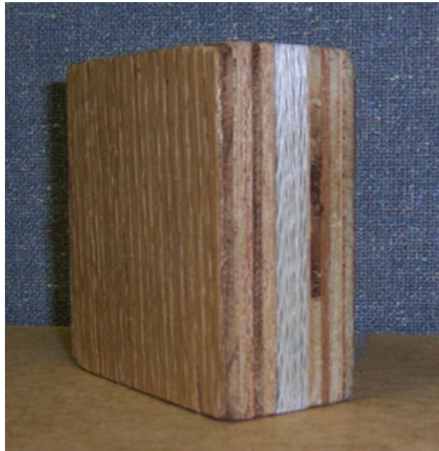
Figure 5-9. Bullet Resistant Fiberglass Door Core
