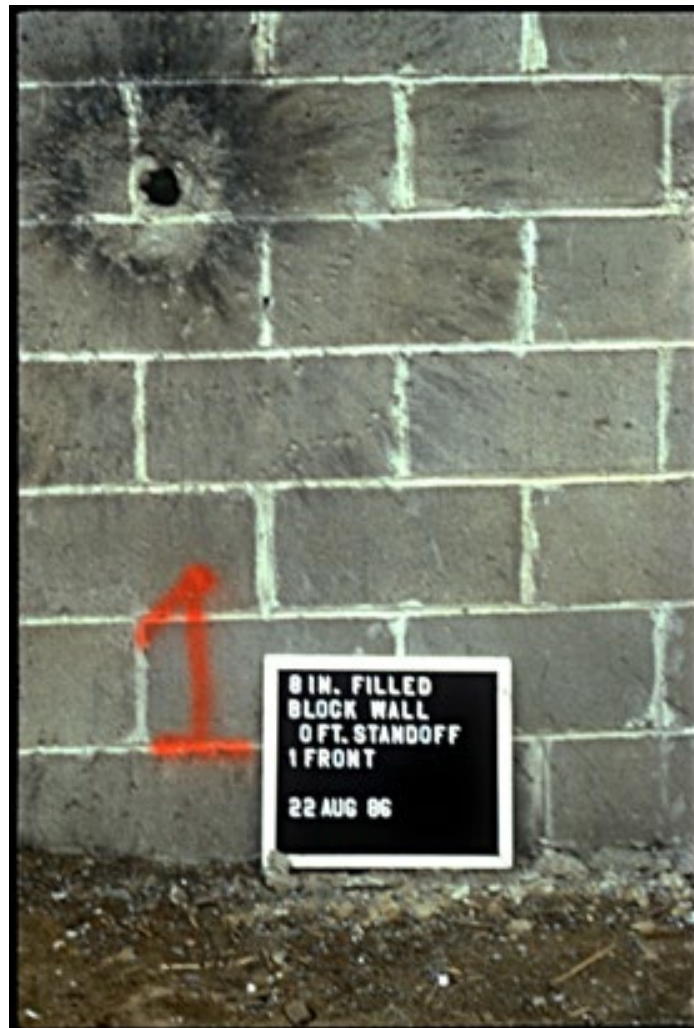
Figure 2-3. Shaped Charge Penetration of Masonry
