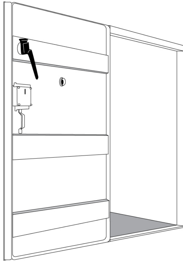
FIGURE 8-3. ROBUST INTERNAL LOCKING DOOR
