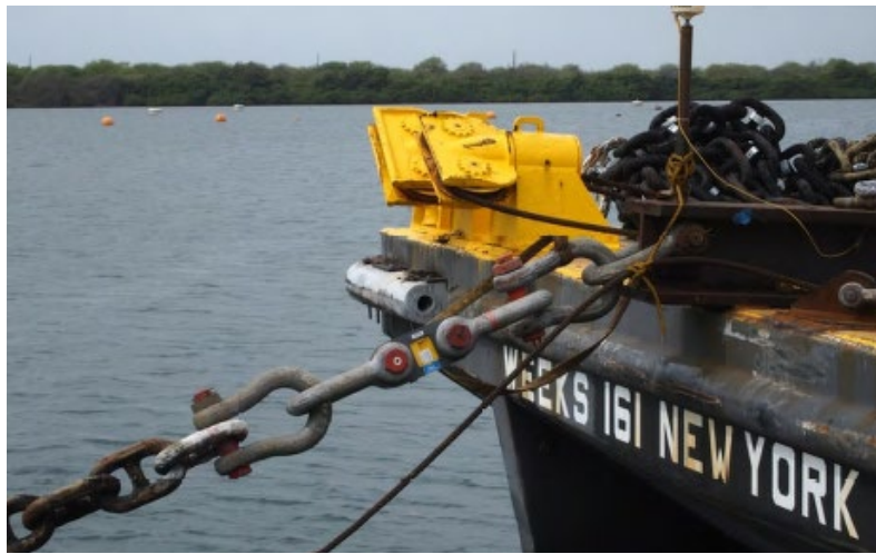
Figure 5-17 Horizontal Pull Test Load Cell Positioning
