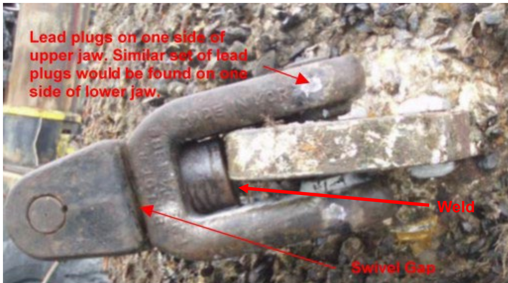
Figure 3-32 Riser Swivel Shackle Inspection Points
