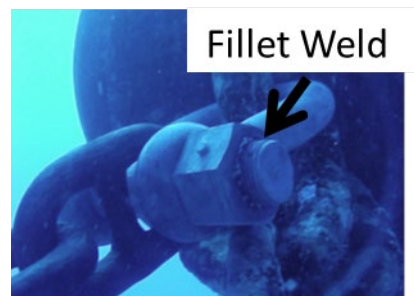
Figure 2-36 Anchor Shackle for Underwater Use
