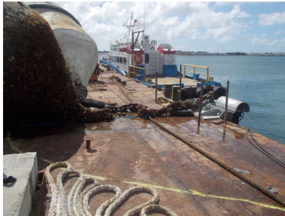
Figure 5-2 Mooring Riser Secured into a CCD
