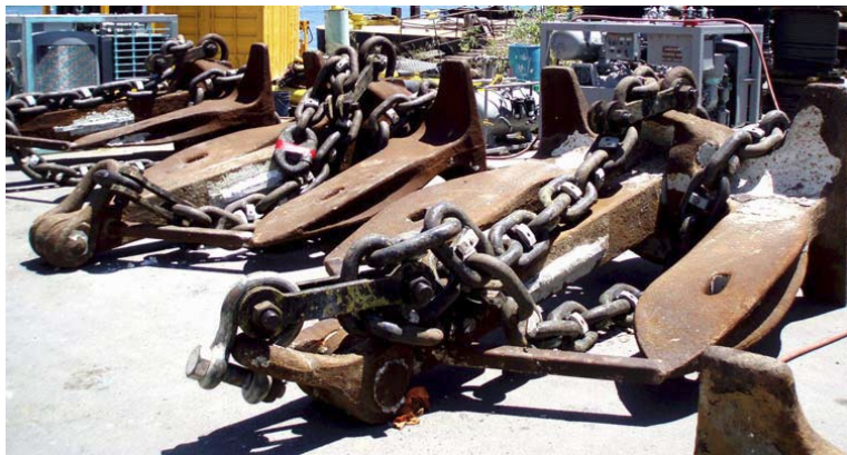
Figure 2-40 Navy Stockless Anchor Rigged as a Sinker
