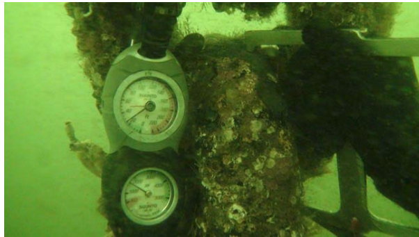
Figure 3-38 Double Link Go/No-Go Measurement
