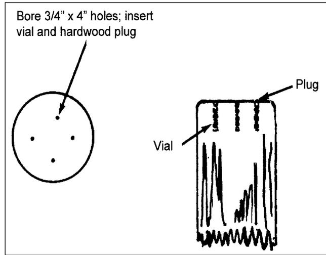
**Figure 3-3. Pile Top Bonnet for Timber Piles**
