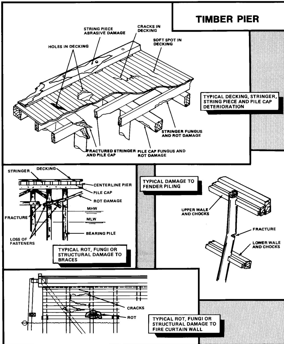
Figure 5-7 Damage to Timber Piles from Biological Sources
