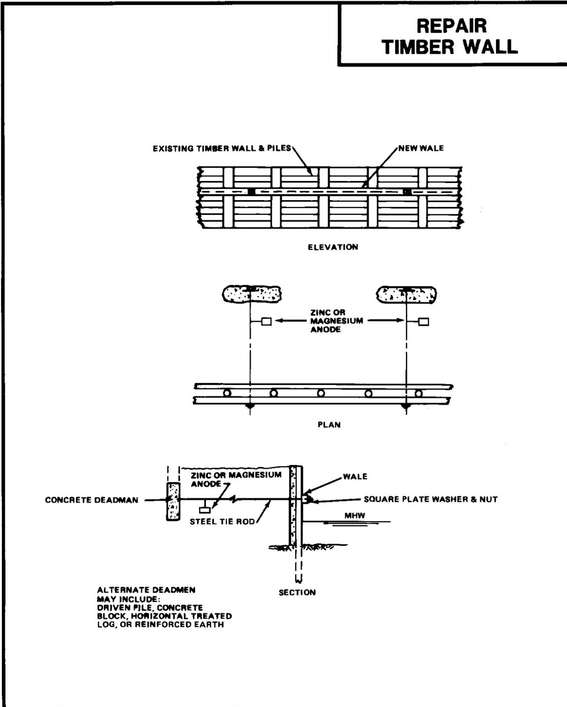
**TR-10: INSTALLING A TIE-BACK SYSTEM ON THE TOP OF A TIMBER SHEET
