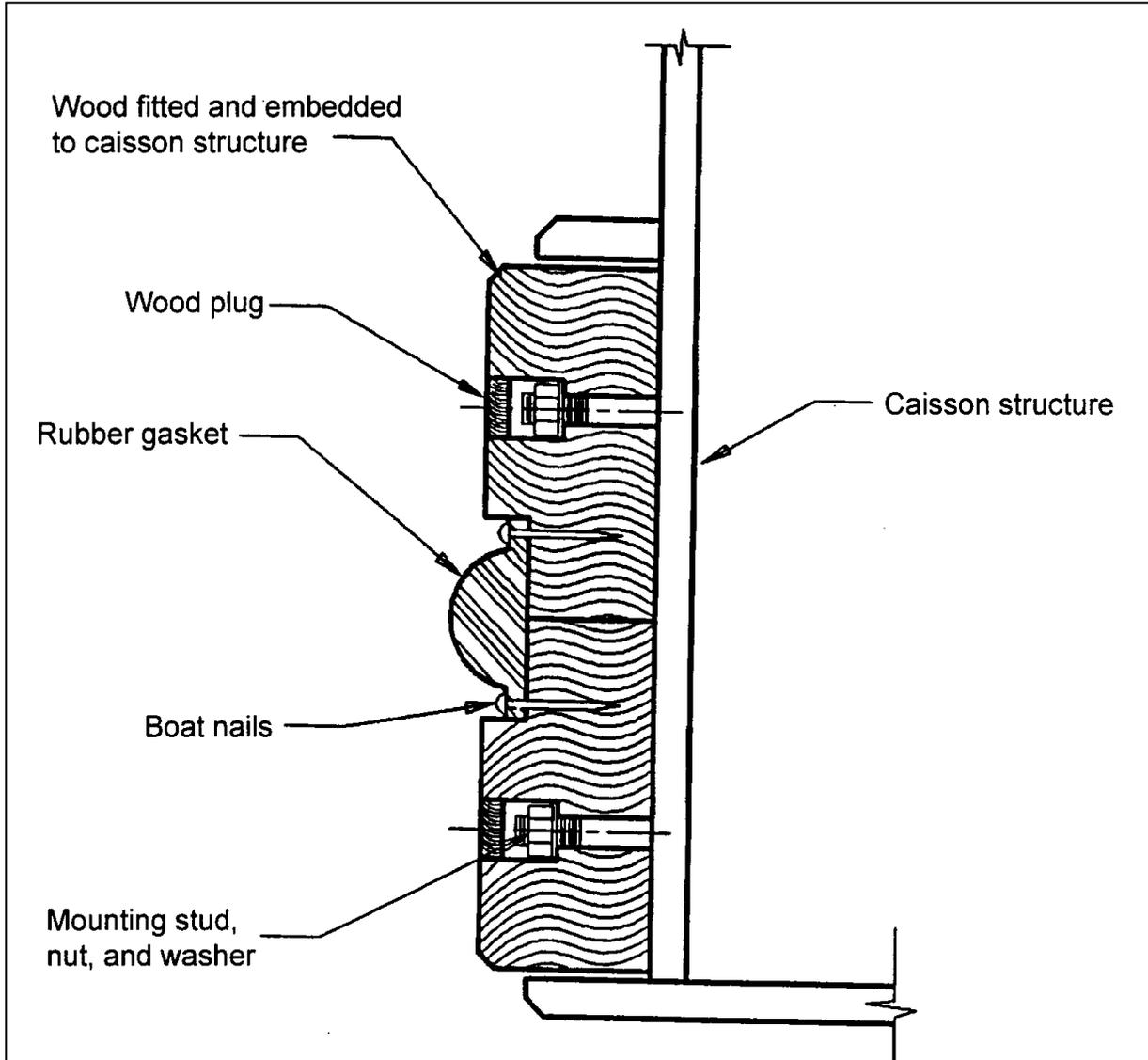
Figure 9-2 Steel Reinforced All-Rubber Caisson Seal Assembly
