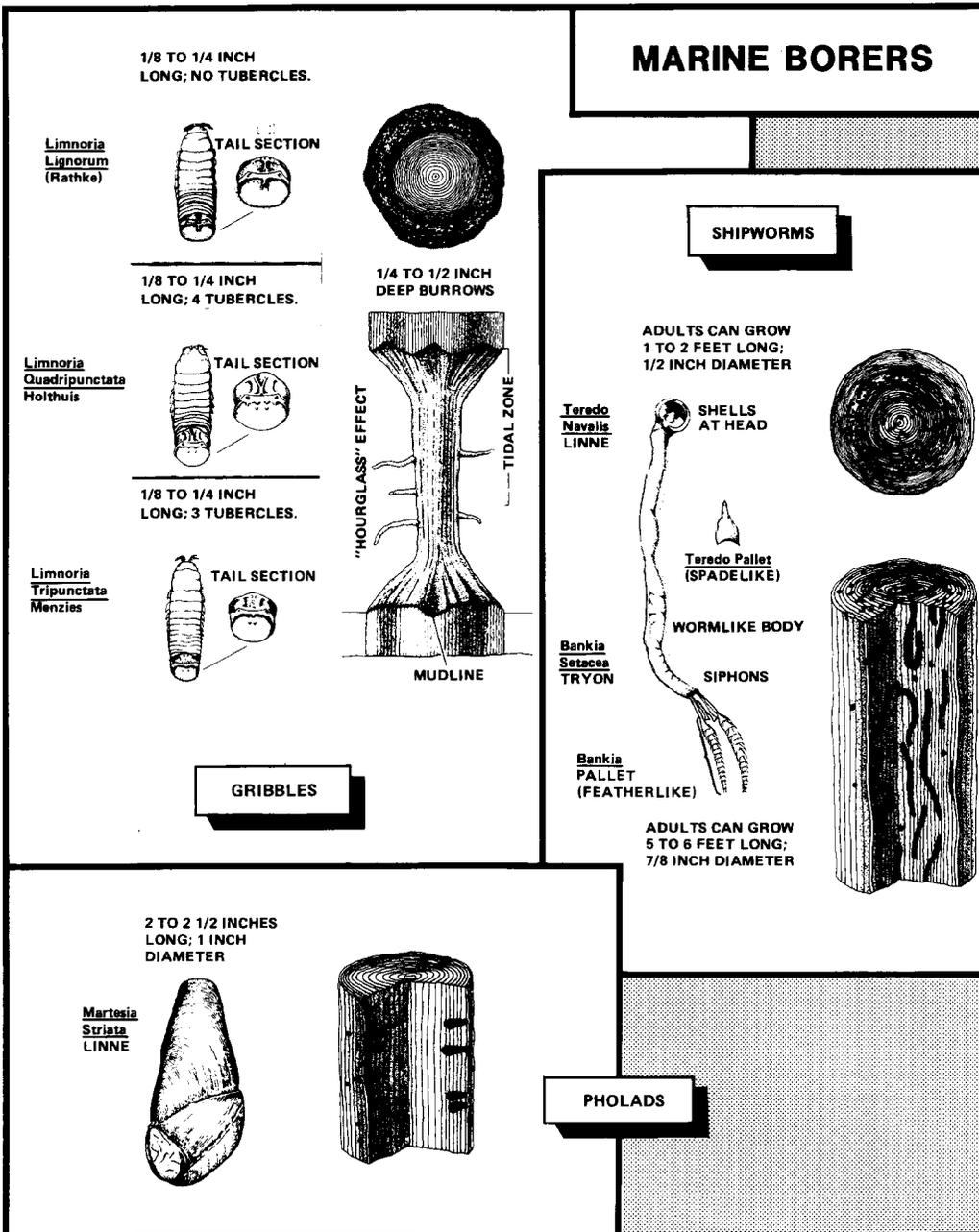
NOTE: Gribbles are 1/8 to 1/4 inch (3mm to 6mm) in length; Shipworms are 1 to 2 feet (30 to 60 cm) in length, 1/2 inch (12.7mm) in diameter; and Pholads are 2 to 2 1/2 inches (51mm to 63.5mm) in length.
