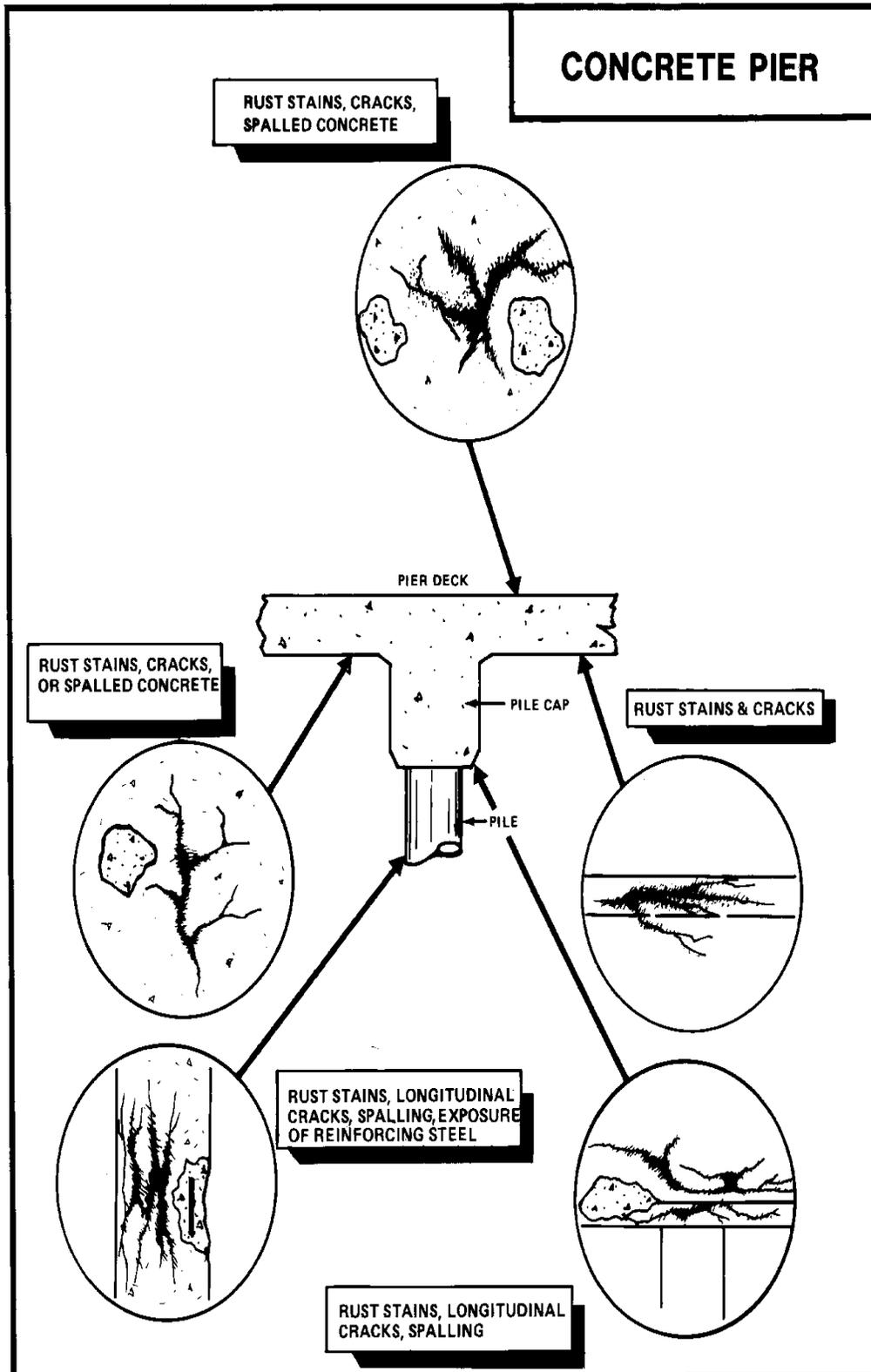
Figure 5-14 Typical Damage to Concrete Piles from Non-Biological Sources
