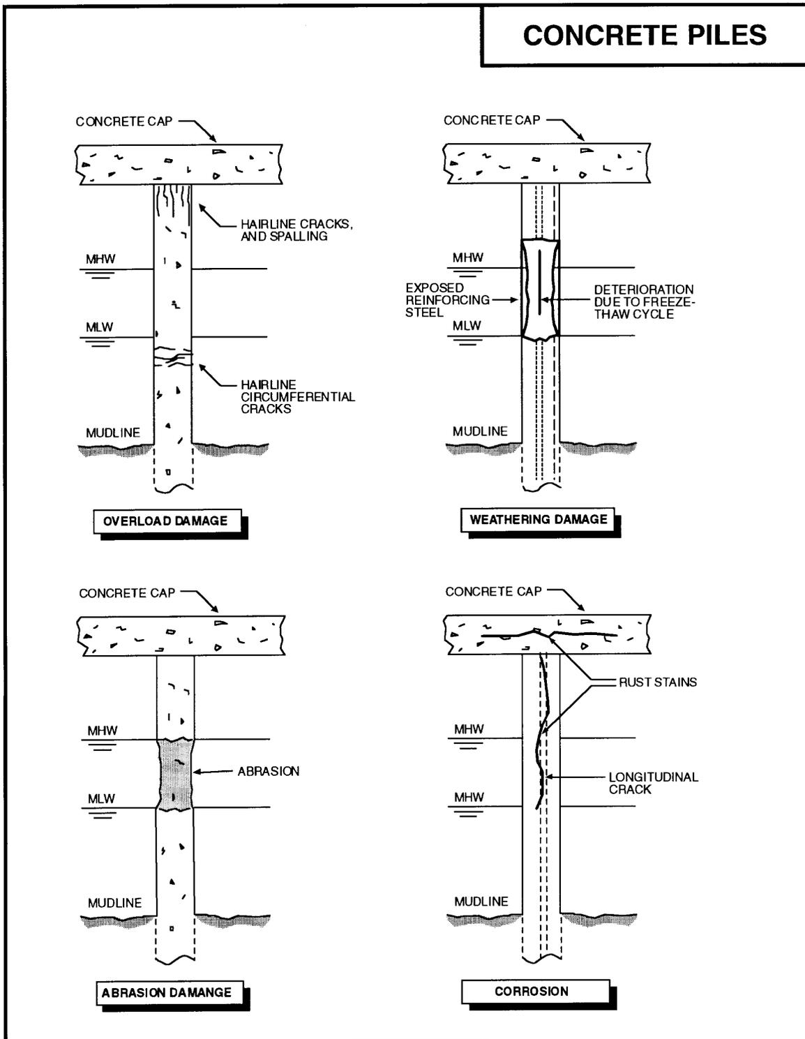
Give special attention to cracks found on the surface of a concrete structure. Make sketches that show the length and direction of the cracks. Overall cracking patterns and changes in crack length, width and direction with time are meaningful data to a structural engineer. Photographs are helpful, but only as a supplement to the sketches.
