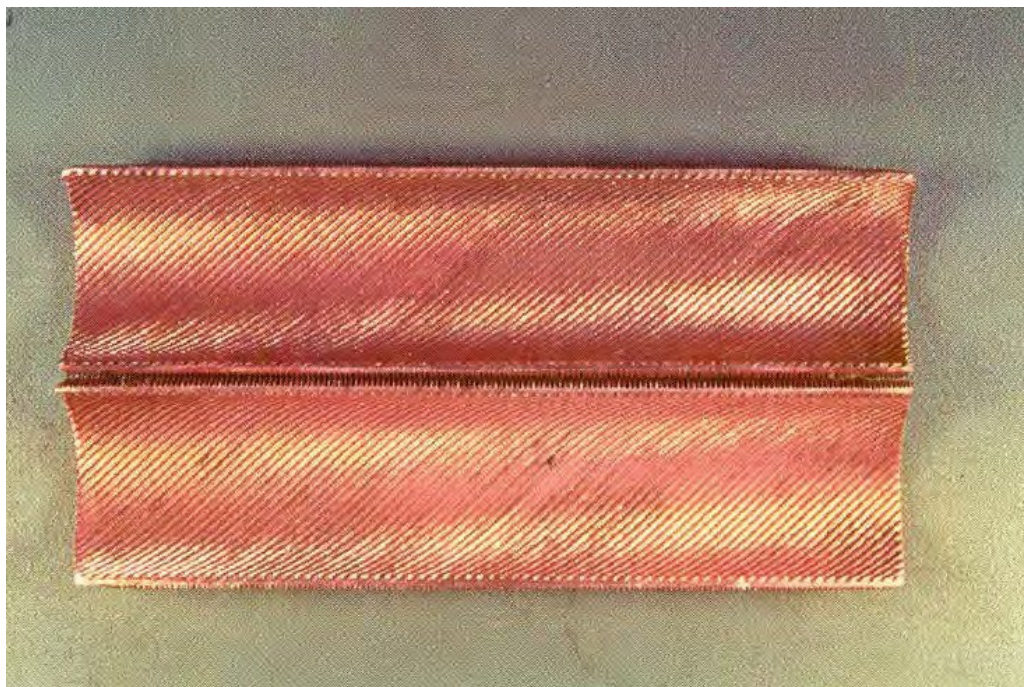
Figure 5-12 Close-Up of Corrosion Pitting on Super-Enhanced Copper Tube
