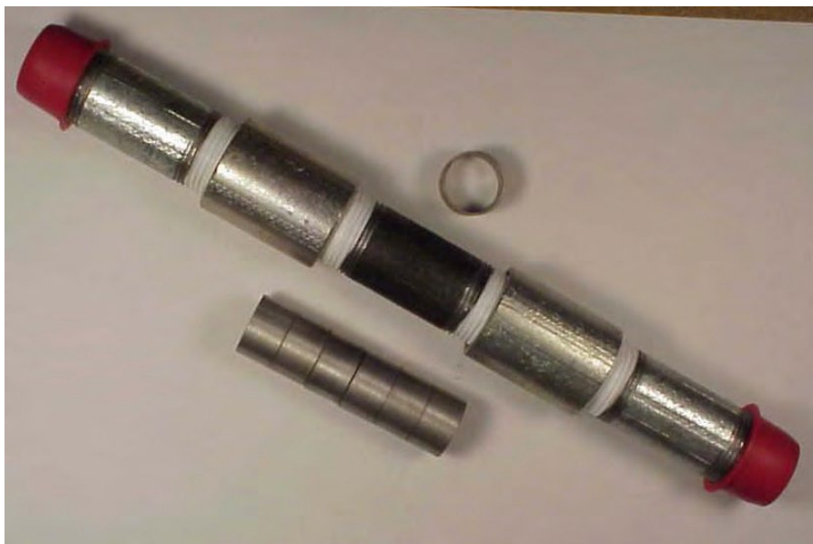
Figure C-1 Condensate Corrosion Tester
