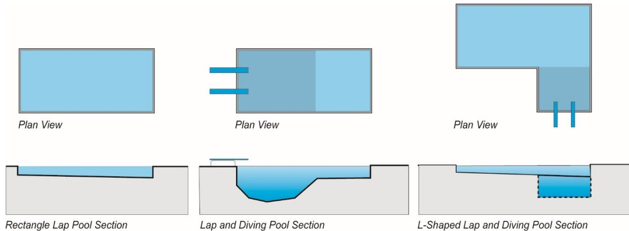
The shape of the pool is affected by the placement of the diving area, if provided. Provide a simple rectangle pool shape for free swimming area, with a diving well placed on either side of the deep end to create an overall “L” shaped pool. If the depth of water in the swimming course is held to a maximum of 5 feet (1.5 meters), the “L”-shaped plan will offer the largest-capacity pool.
