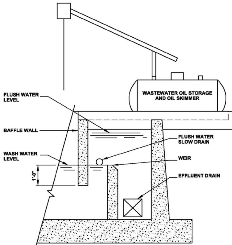
Figure 6-8 Sedimentation Basin Drain System
