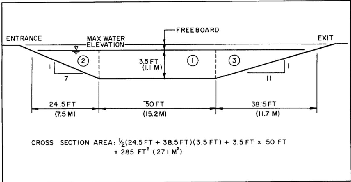
$$Q_1 = (\text{width} \times \text{cross section}) \times 7.48 \text{ gpcf/drain time}$$
