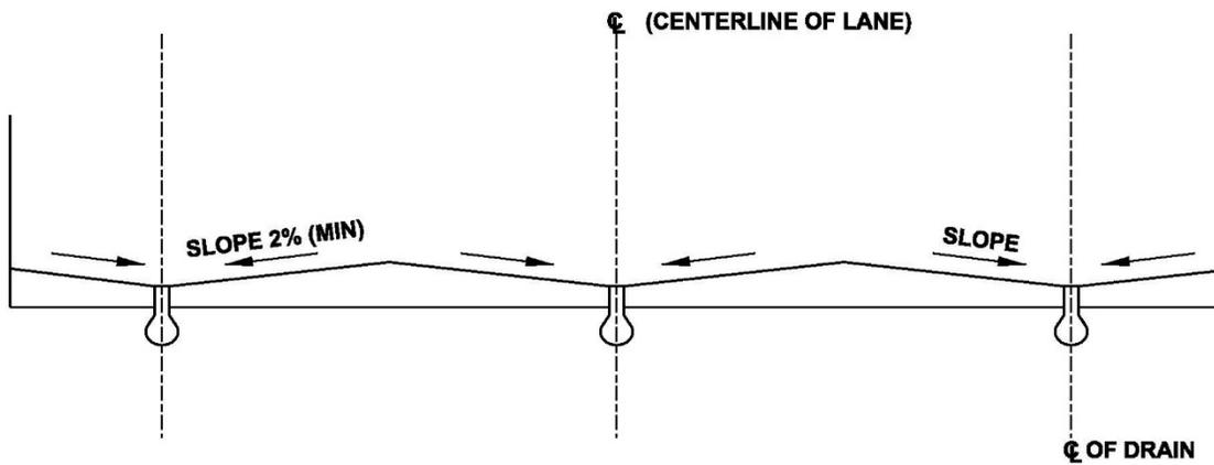
Figure 5- 10 Configuration of U-Drains in the Bath
