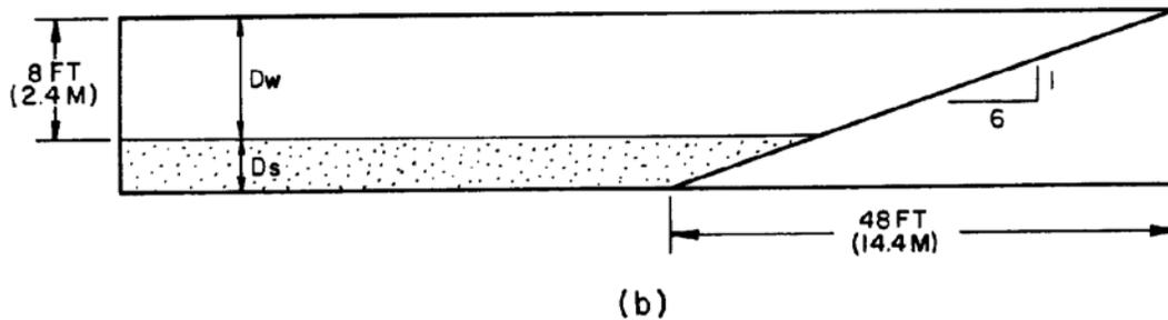
c. Sediment Volume. The designer estimates that the installation has average-to-heavy soiling conditions. By applying Stokes Law, using  $Q_{over}$  with the basin size previously calculated, and checking the soil particle size
