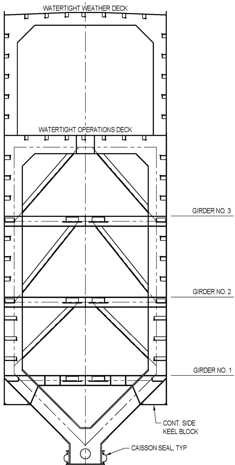
Figure 9-4 Typical Horizontal Girder for Welded Caisson
