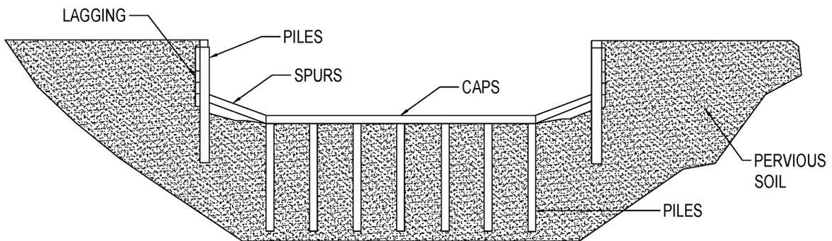
b) TEMPORARY, ALL TIMBER DRY DOCK, CONSTRUCTED IN OPEN CUT FOR BUILDING FLOATING STRUCTURES
