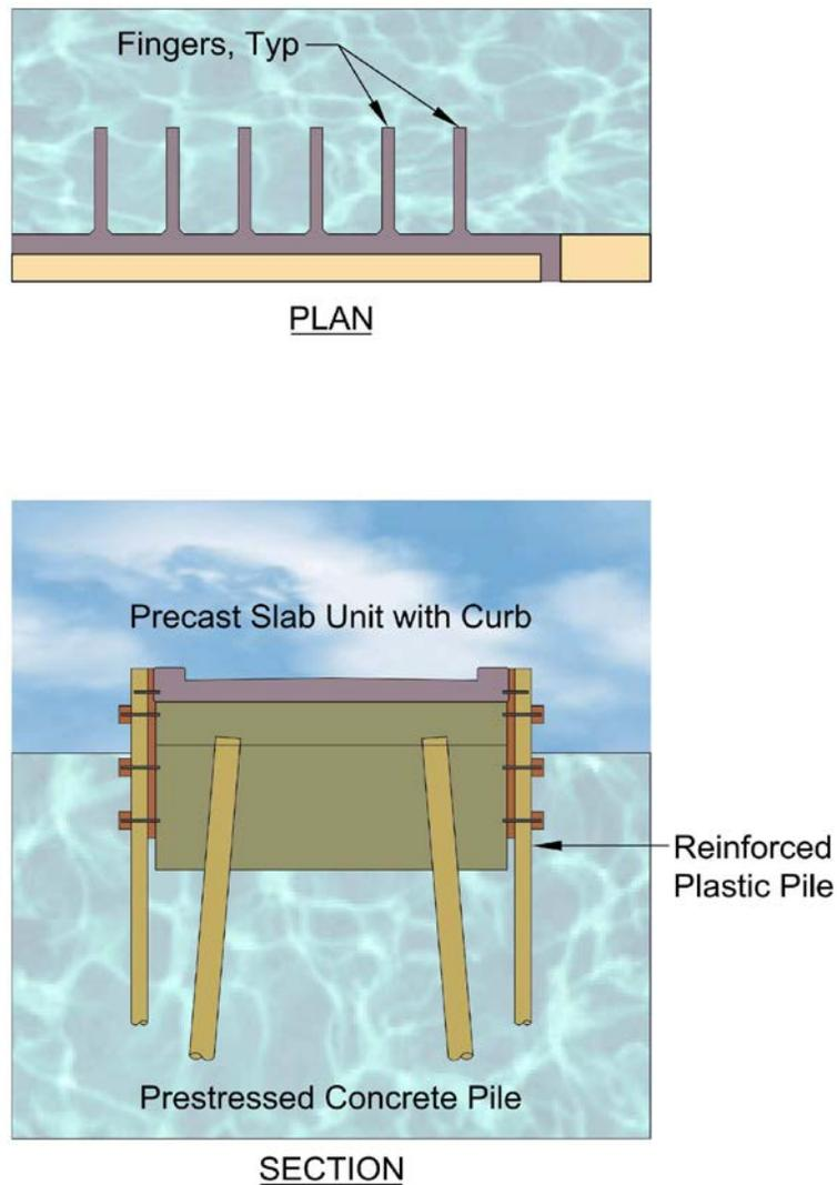
6-1.1.2 **Floating systems.** Floating systems are generally preferred where the tidal range or seasonal water level range is 3 feet (0.91m) or more. Figure 6-2 shows a typical floating pier system.
