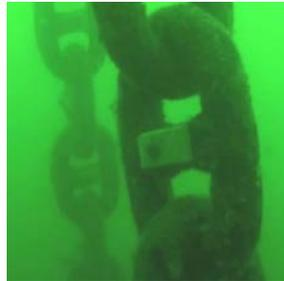
**Figure 2-51 Chain Stud Anode on Buoy Tension Bar**
