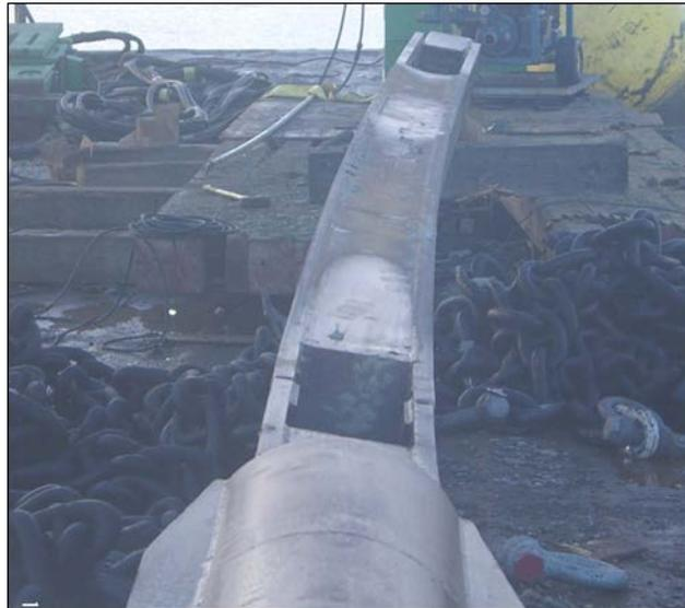
Once the follower is extracted, a suitable sea water pump will be needed to remove the plug of soil that normally forms within the flanges of the follower at cohesive soil conditions. As the extracted follower will form a vertical plug below the seabed, sometimes steel plate is welded between the flanges to stiffen the follower at the bottom end. However, this adds additional cost and weight to the follower.
