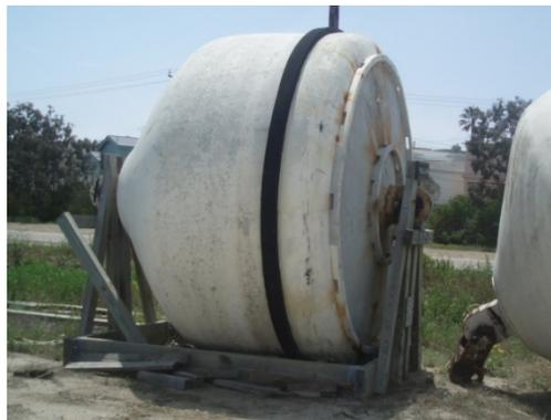
Foam buoys should be stored on specially designed wood buoy cradles to avoid a permanent flat spot.
