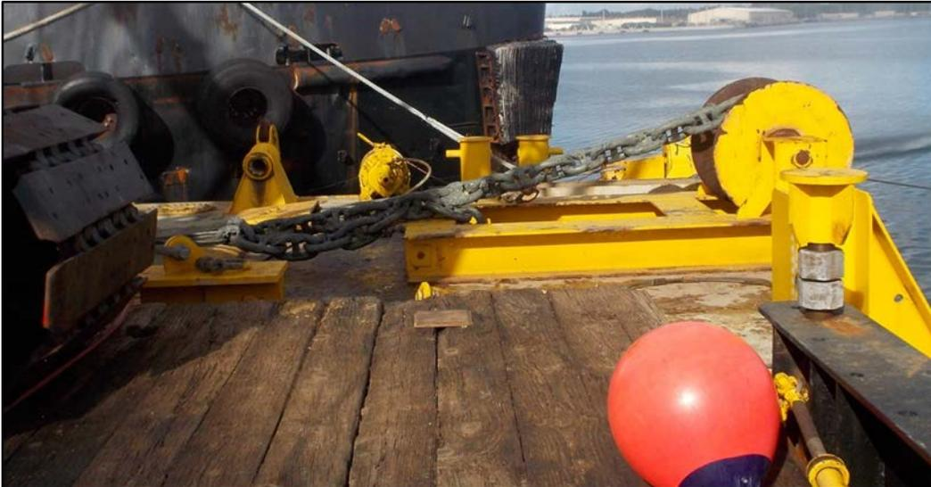
The repaired ground leg is placed back into the water using the double drum winch in a similar fashion, but in reverse, with the anchoring system, or tugboats, pulling the crane barge back toward the ground ring pick-up buoy.
