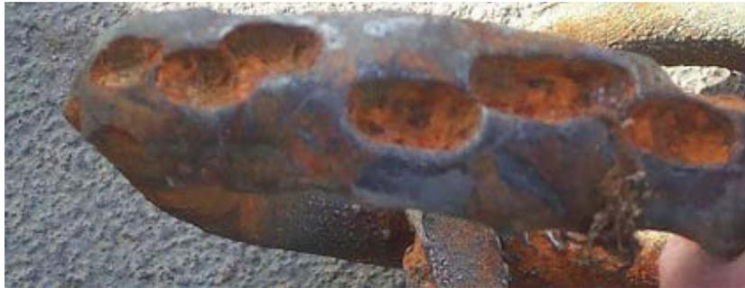
**Figure 3-41 Worn 3.5-inch Chain with Stud Missing**
