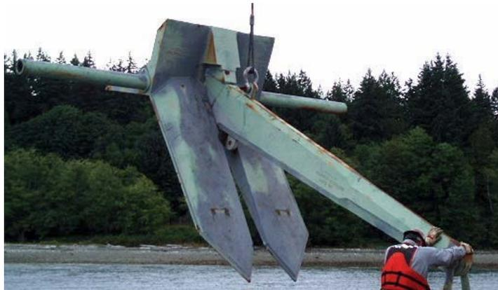
**Figure 5-8 Stockless Anchor Deployment**
