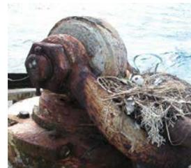
For mechanical wear at the pin and bale contact points, the buoy anchor bolt shackle is assessed as C1, C2 or C4 using similar criteria as done for chain measurements. Table 3-6 provides catalog dimensions for Fleet Mooring anchor bolt shackles and 90% and 80% levels. Rust products should be removed prior to performing caliper measurements to obtain accurate measurements at the wear points.
