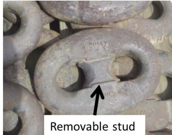
AJLs are used to connect chain to chain components with a larger diameter (ground rings, spider plates, shackles on anchors, etc.). It is larger on one end to accommodate the larger diameter wire of those components. Figure 2-25 and Figure 2-26 show the different types of AJLs.
