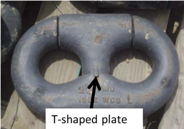
**Figure 2-24 Kenter Style Chain Joining Link**
