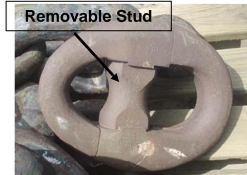
When a connecting link is reassembled, the pieces are secured with a pin which is held in place by a lead plug. Lead plugs are either pounded into place using a heavy hammer or the lead is melted into the hole from a long lead bar. All joining links should have a visible lead plug (some cleaning may be required for joining links that are below the waterline to locate the lead plug) in the large pin hole (see Figure 2-27). Figure 2-28 shows a missing lead plug.
