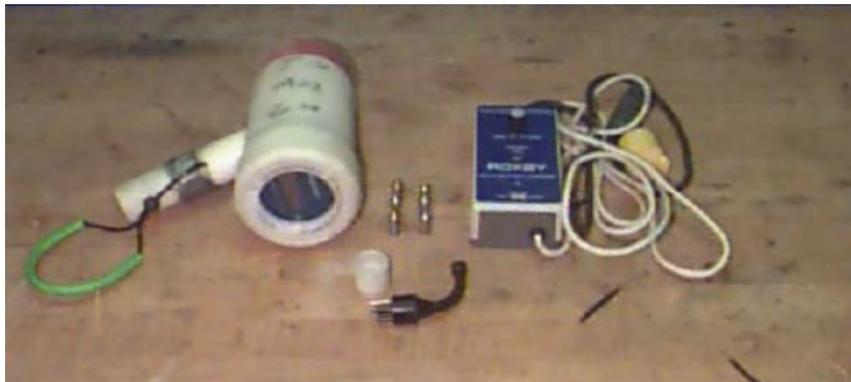
A diver held Bathyorrrometer consists of a silver/silver chloride reference electrode, a self-cell, a digital voltmeter and a probe. The unit operates by measuring the potential difference between the reference electrode and the material being measured. The potential reading is displayed on a liquid crystal display.
