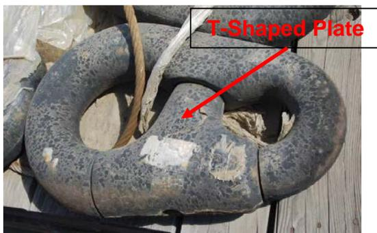
**Figure 2-26 Kenter Style Anchor Joining Link**
