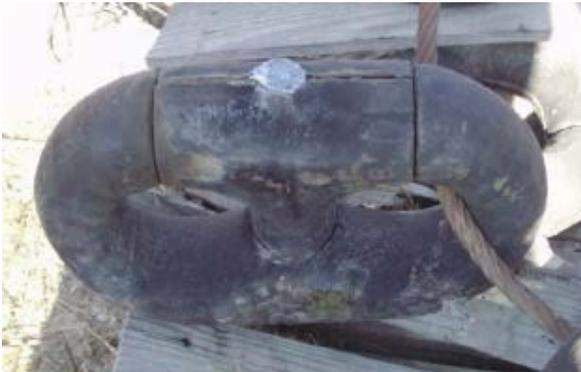
**Figure 2-28 Missing Lead Plug**
