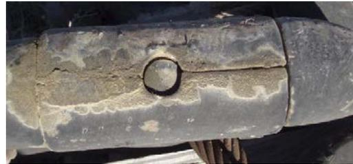
Disassembled joining links should not be mixed with parts from other disassembled links as the tracking of serial number data on the installed link would be interrupted and the mixing of parts may result in the joining link not being able to be reassembled due to fit interferences among the mixed parts.
