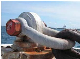
**Figure 3-23 Heavy Corrosion**
