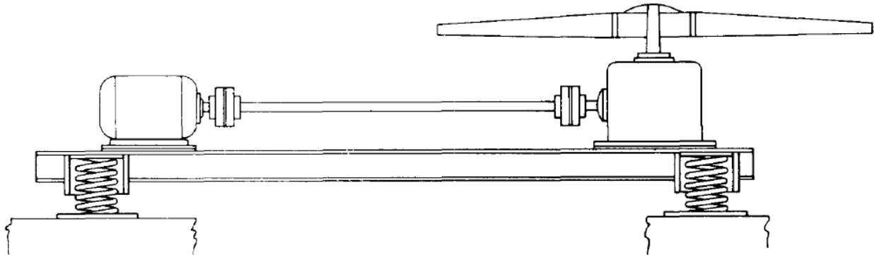
**Figure C-24 Schematic of a Resilient Clamping Arrangement With Ribbed Neoprene Pads**
