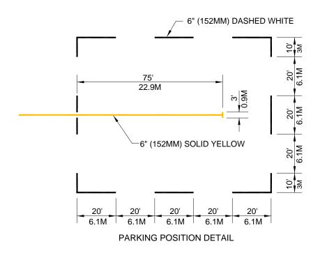
Figure 7-14. Type 2 Parking for Wheeled Rotary Wing Aircraft
