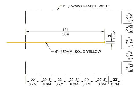
Figure 7-13. Type 1 Parking for all Rotary Wing Aircraft Except CH-47
