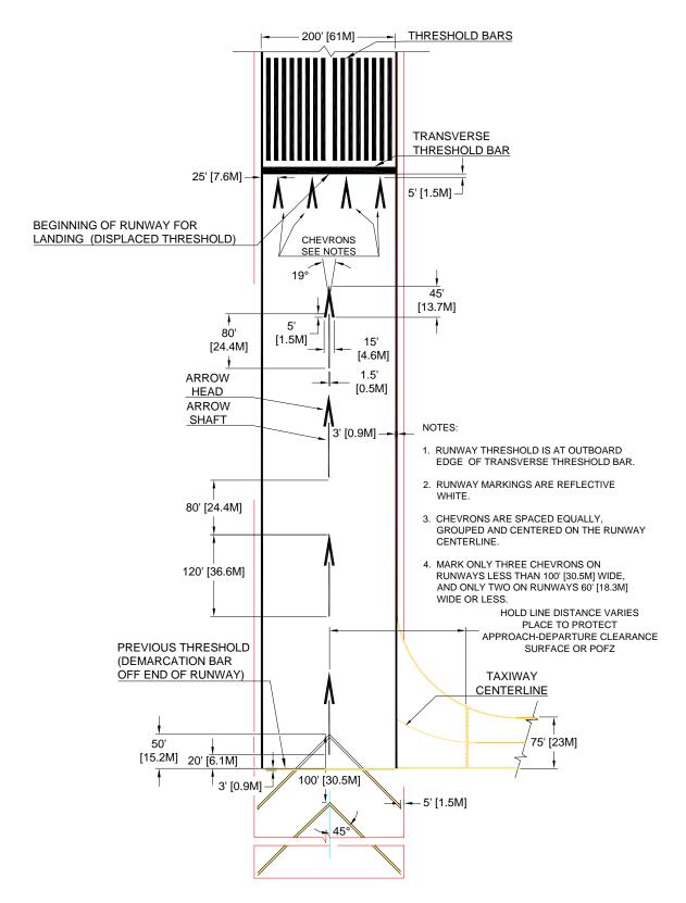
Figure 5-9. Permanently Displaced Threshold Where Preceding Pavement is Used as a Taxiway
