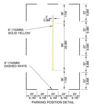
Figure 7-15. Type 2 Parking for Skid Rotary Wing Aircraft
