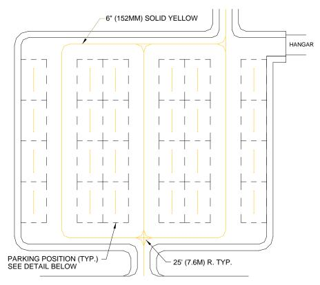
TYPE 2 PARKING FOR WHEELED ROTARY WING AIRCRAFT
