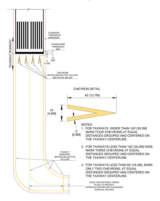
Figure 5-10. Permanently Displaced Threshold Where Displacement Area is Used as a Taxiway and for Take-Off and/or Landing Ground Roll
