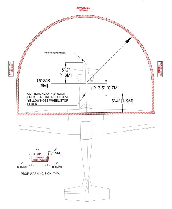
Figure 8-12. T-6 Propeller Hazard Area Pavement Markings
