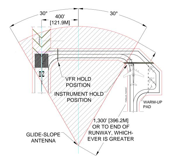
Figure 6-6. Locating Instrument Hold Positions to Protect Touchdown Zone Critical Area
