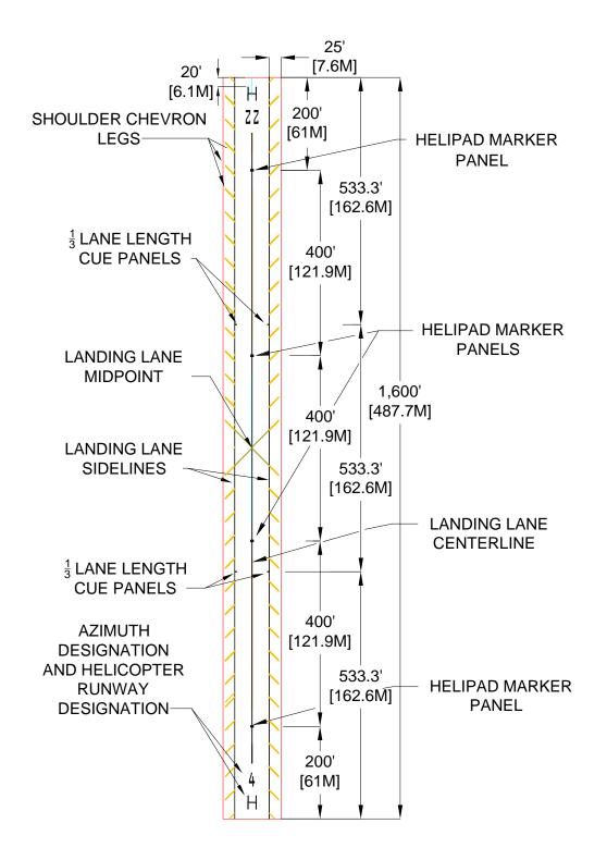
Figure 7-8. Landing Lane Helipad and 1/3rd Length Marker Panels
