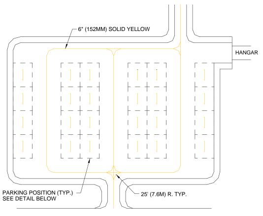
TYPE 2 PARKING FOR SKID ROTARY-WING AIRCRAFT
