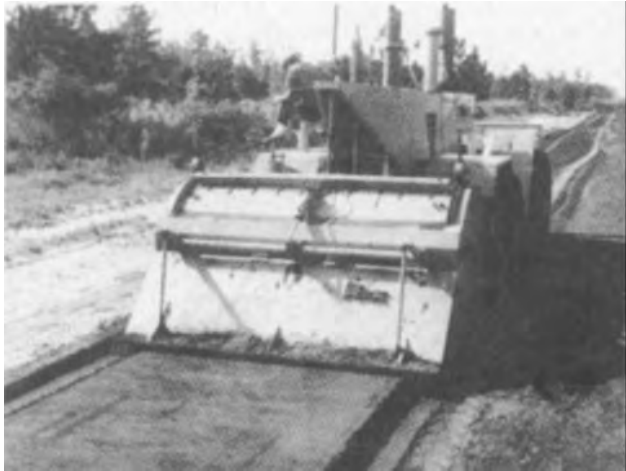
Figure 4-49. Single-shaft rotary mixer without asphalt.
