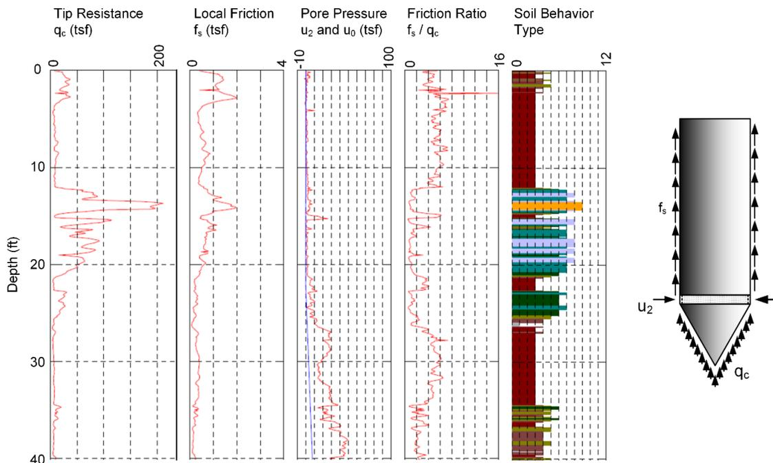
**Figure 2-8 CPT - Example Test Record and Equipment**
