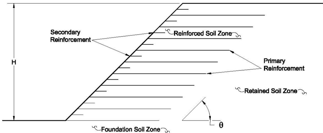
**Figure 7-11 Typical Cross-Section of an MSE Slope**
