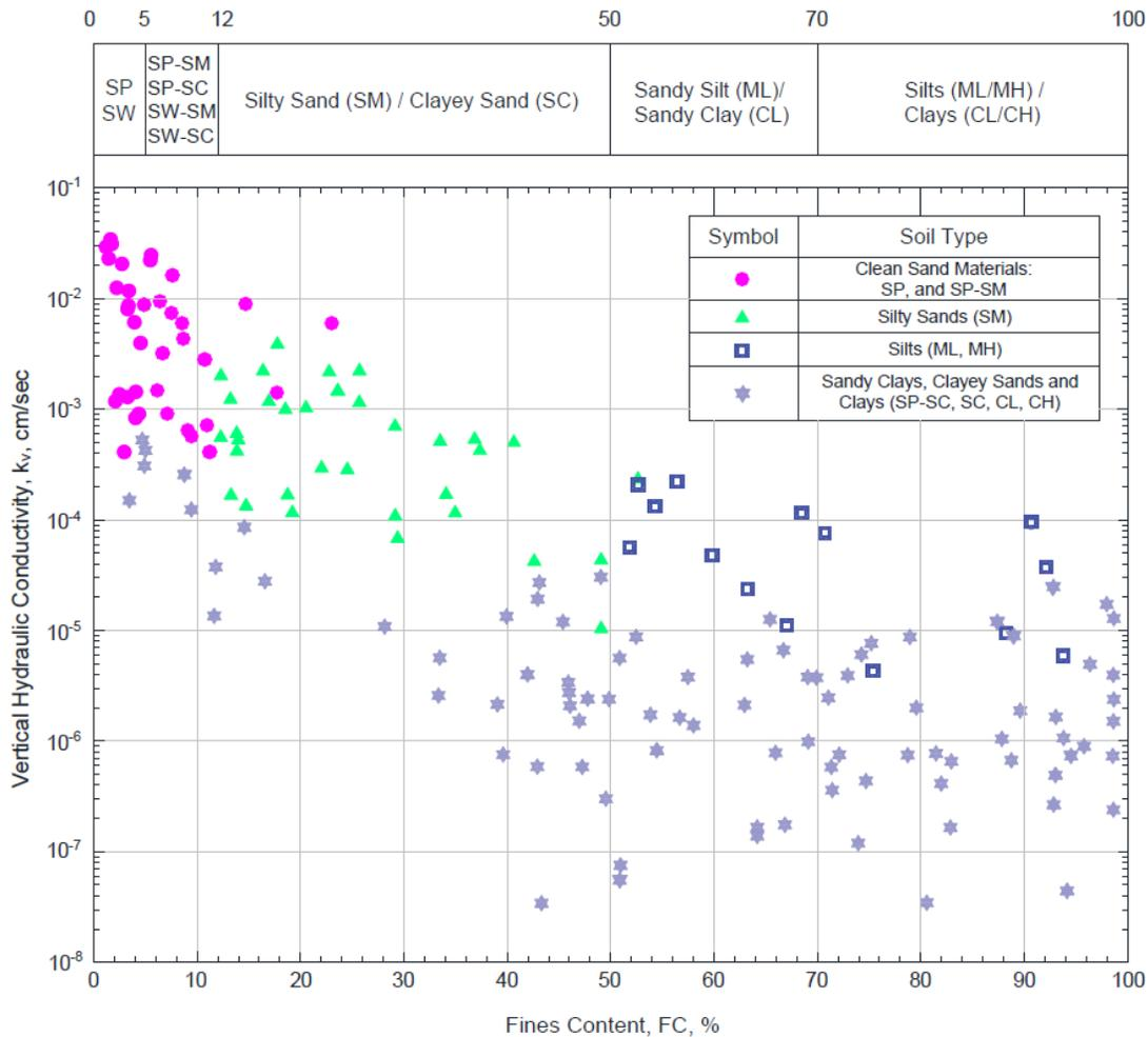
**Figure 6-7 Variation of Hydraulic Conductivity with Fines Content
