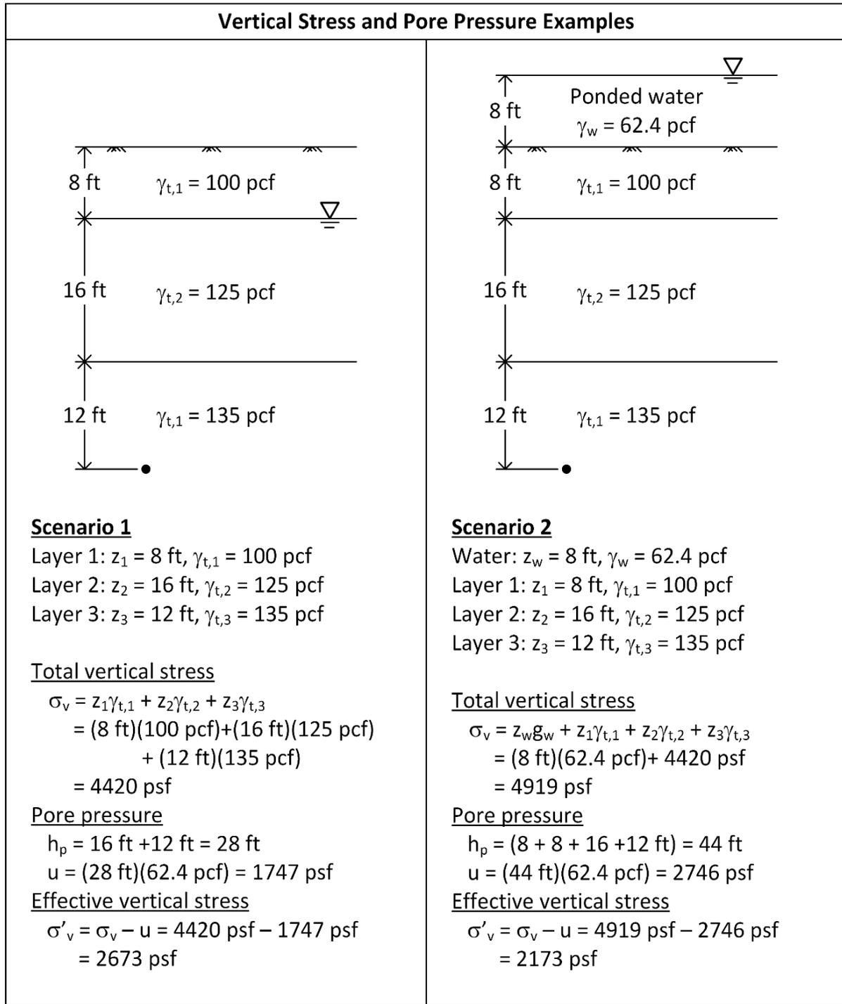
**Figure 4-1 Calculation of Vertical Stresses for Hydrostatic Conditions**
