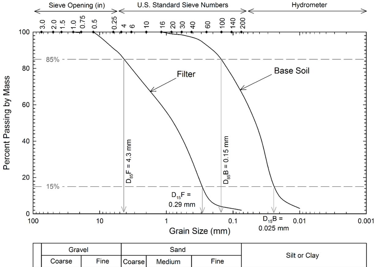
**Figure 6-15 Example Base Soil and Filter Gradations**
