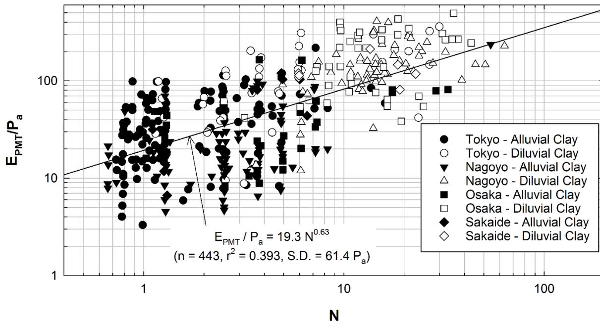
**Figure 8-52 Correlation between PMT Modulus for Clays and SPT  $N$**
