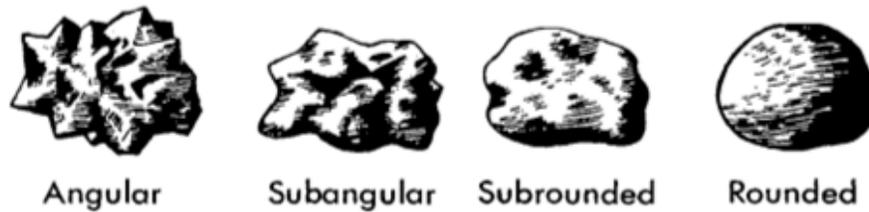
**Figure 1-1 Typical Angularity of Bulky Grains (after Sowers 1979)**
