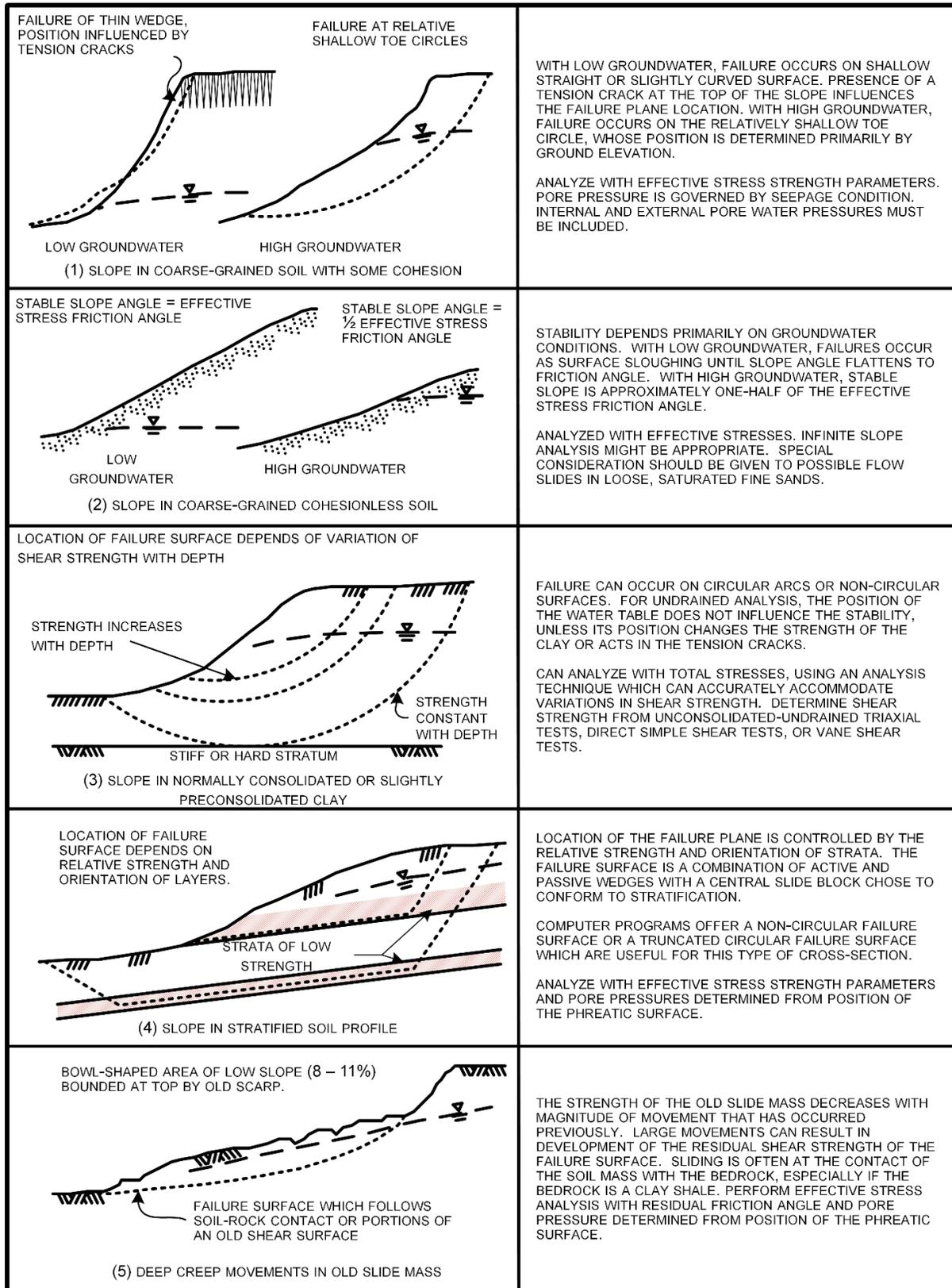
**Figure 7-1 Failure Conditions for Cross-sections through Natural Slopes**
