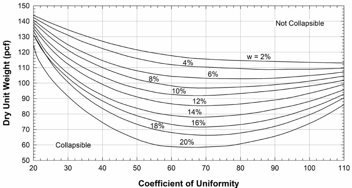
**Figure 1-10 Design Charts for Predicting Collapse Behavior of Soils**
