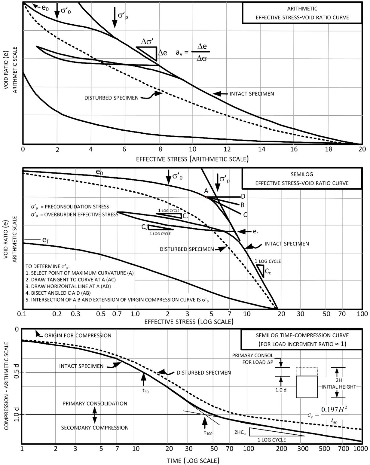
Figure 3-12 Basic Information Obtained from a Consolidation Test
