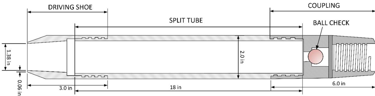
**Figure 2-2 Cross Section of Split Barrel Sampler**
