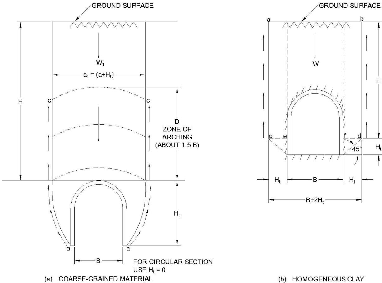
**Figure 4-11 Loading Mechanisms for Soft Ground Tunneling**
