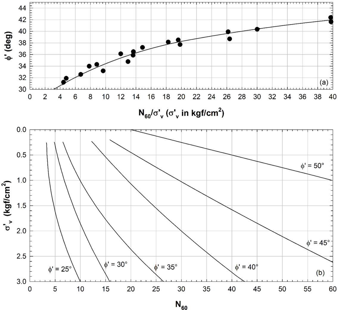
**Figure 8-3 Relationship between Peak Effective Stress Friction Angle, Overburden Pressure, and SPT Blow Count for Sands (top) after Parry (1977) and (bottom) after DeMello (1971) and Schmertmann (1975)**
