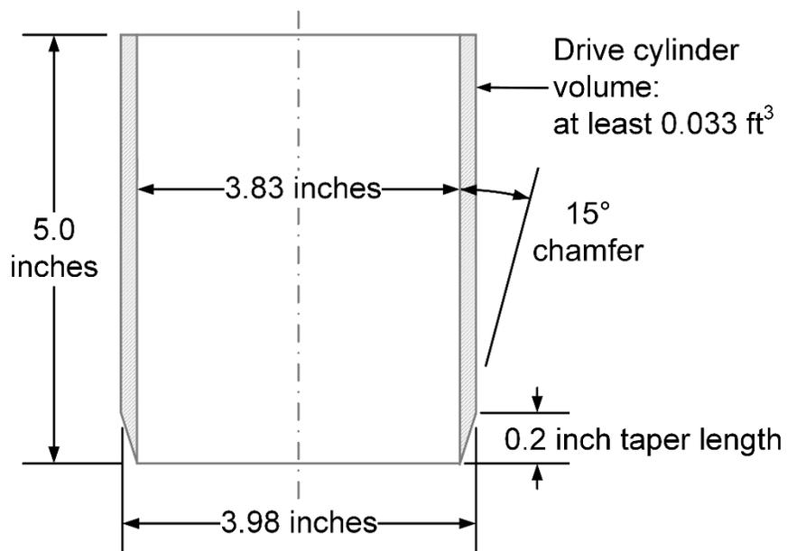
**Figure 2-20 Schematic of Drive Cylinder (after ASTM D2937)**
