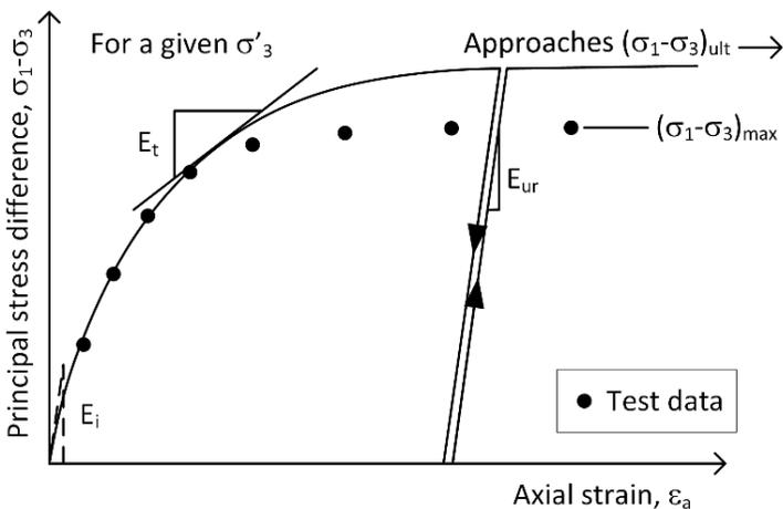
Calculate  $E_t$  using  $c'$  and  $\phi'$
