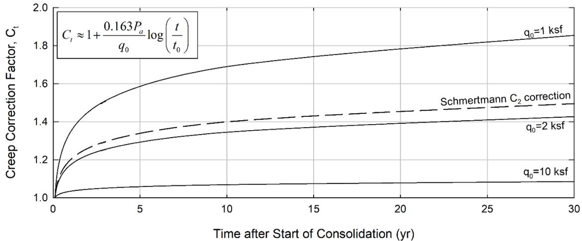
**Figure 5-9 Creep Factors for Settlement of Coarse-Grained Soils**
