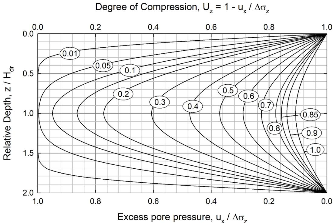
**Figure 5-17 Degree of Compression and Excess Pore Pressure
