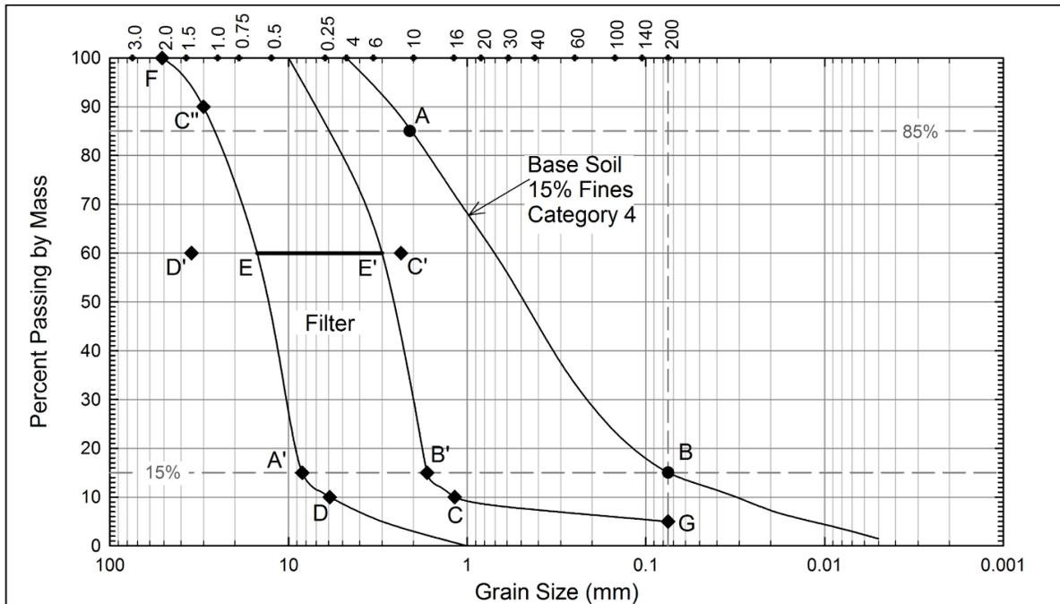
**Steps 1-3:** Plot the grain size distribution(s) for the base soil. If necessary, regrade the grain size distribution to include only the portion of the distribution finer than the No. 4 sieve.
