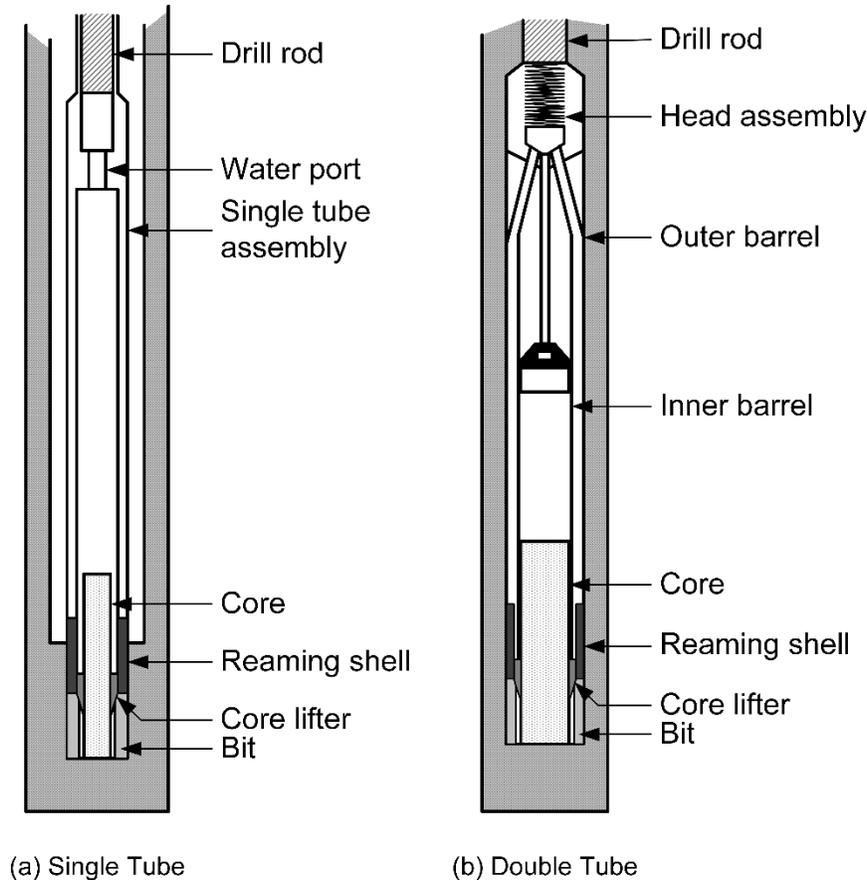
**Figure 2-5 Rock Core Samplers (after NCHRP 2018)**
