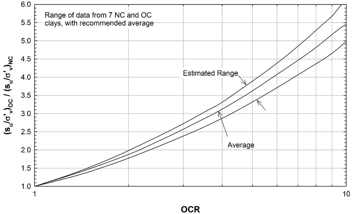
**Figure 8-30 Normalized Undrained Strength Ratio vs. *OCR***
