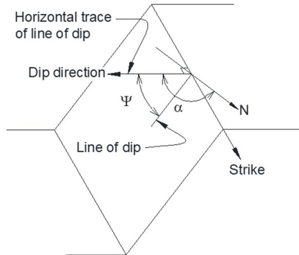
**Figure 7-16 Definition of Sloped Surface Orientation Terms**
