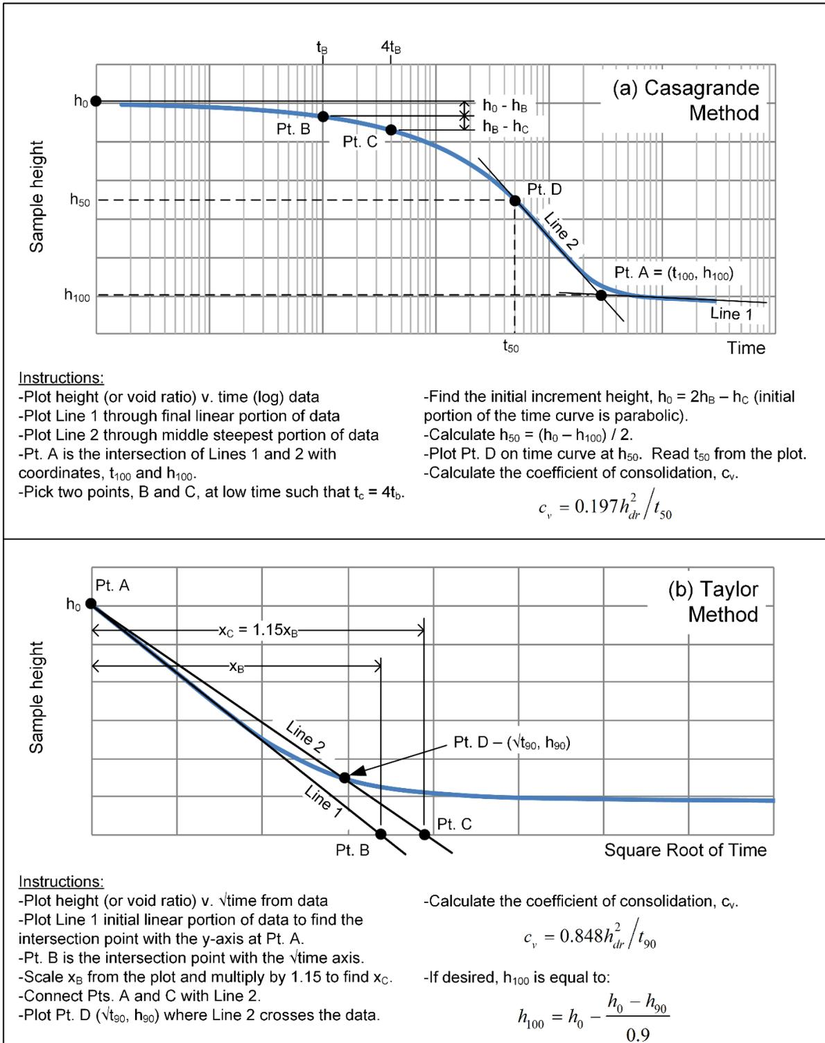
**Figure 5-21 Determination of Coefficient of Consolidation from Laboratory Data**
