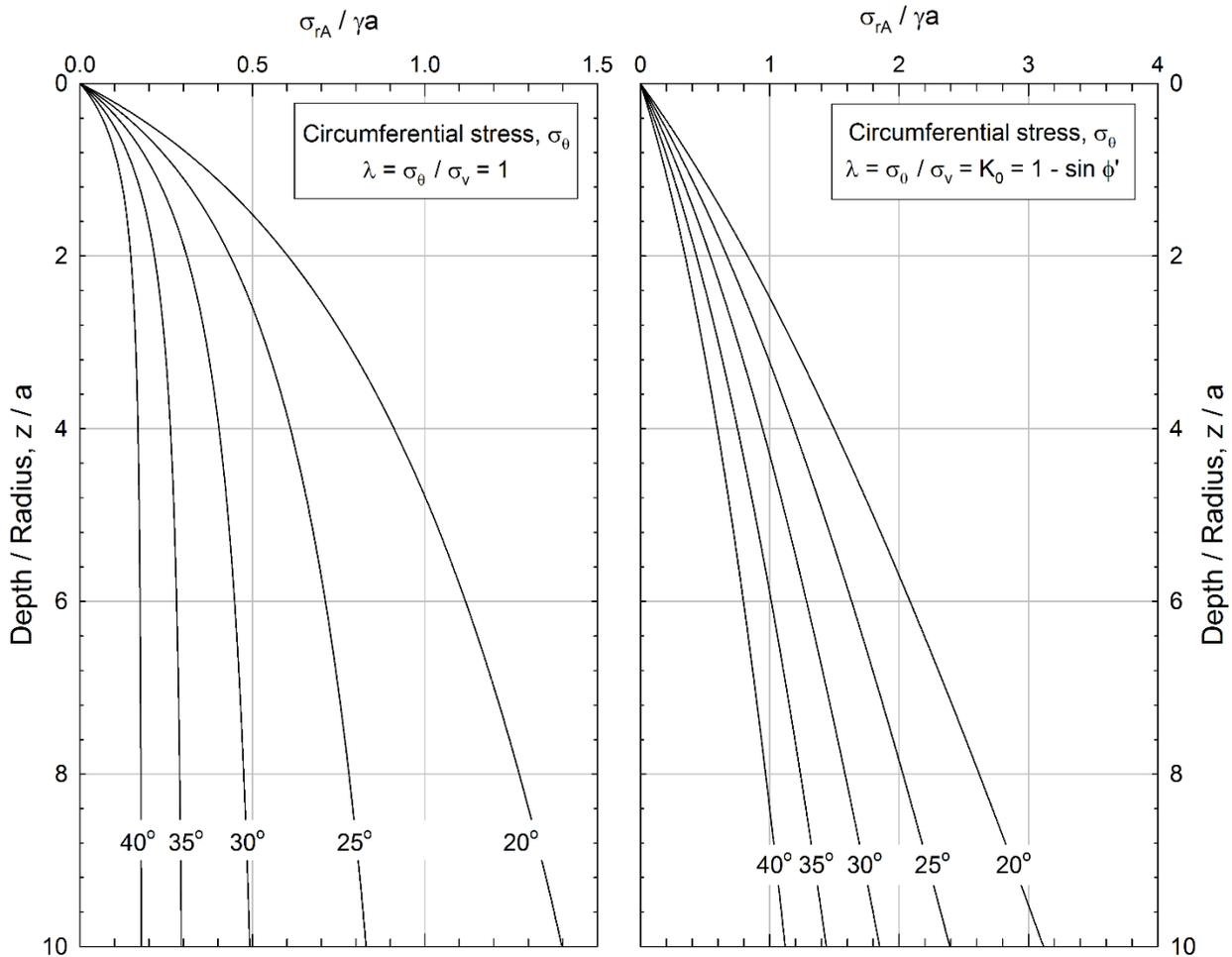
**Figure 4-12 Radial Stress at the Sides of a Vertical Shaft in Sand
