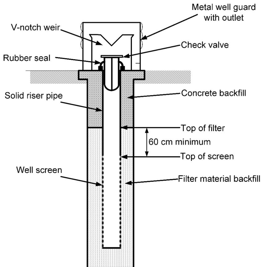
**Figure 6-29 Typical Relief Well Construction**
