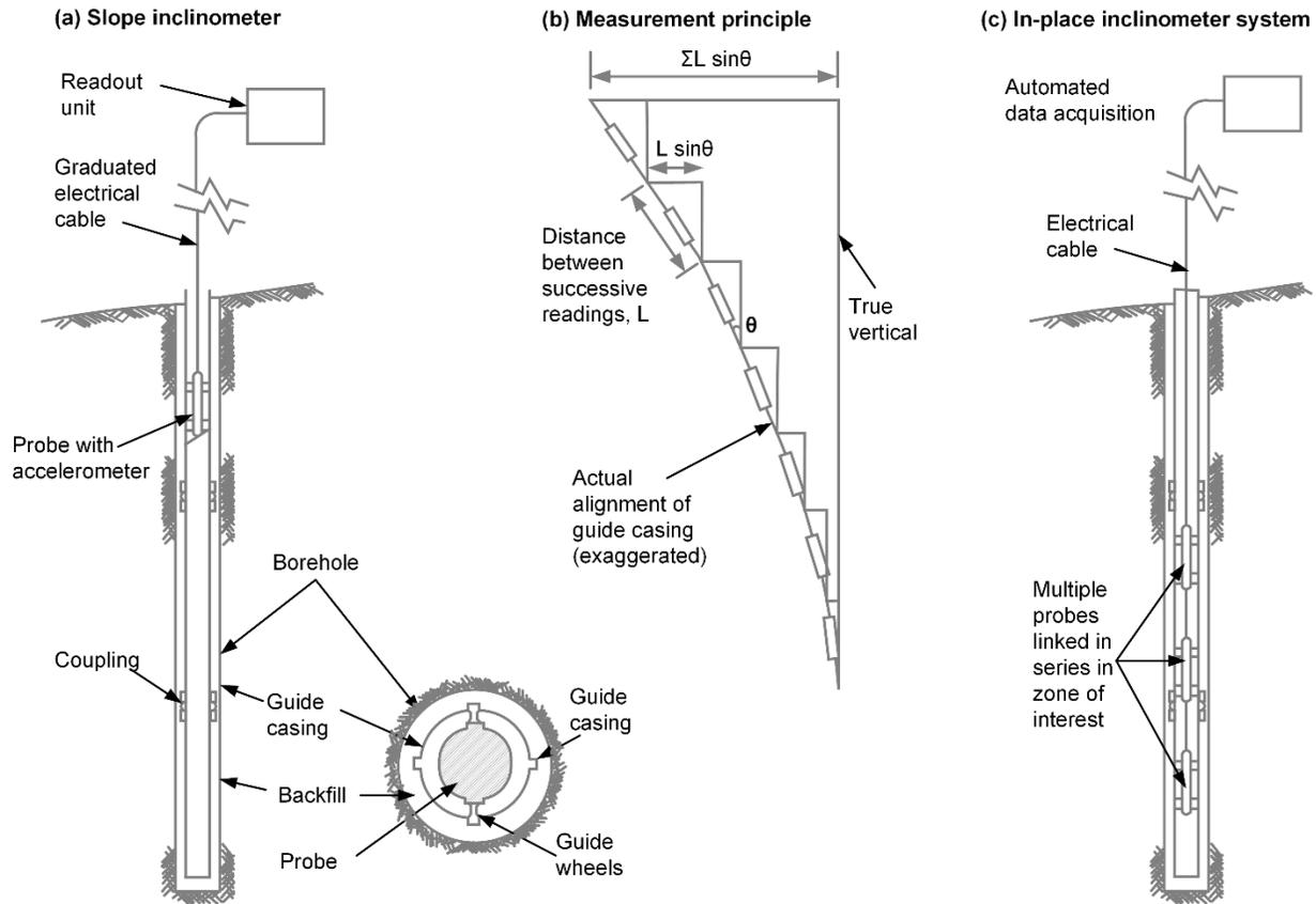
**Figure 2-28 Slope Inclinerometers – (a) Manual System, (b) Measurement Principle, and (c) In-Place Inclinerometer System (after Dunicliff 1993)**
