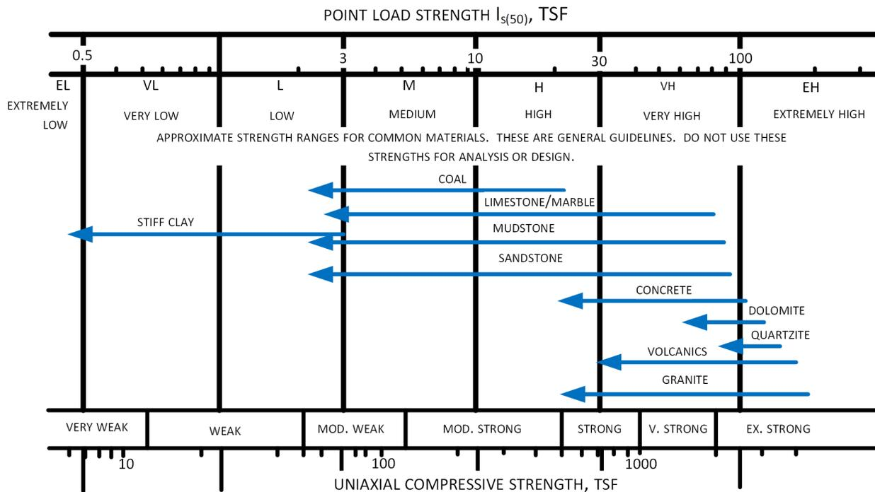
**Figure 1-4 Rock Strength Characterization (after Broch and Franklin 1972)**
