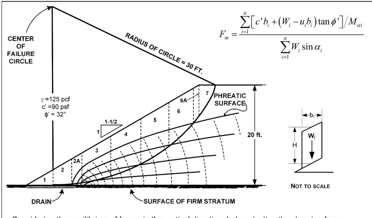
Considering the equilibrium of forces in the vertical direction, but neglecting the shearing forces between slices, the factor of safety for moment equilibrium can be calculated as indicated above. This equation can be solved by iteration using a spreadsheet. Values of  $M_{\alpha_i}$  can be obtained from the chart below.
