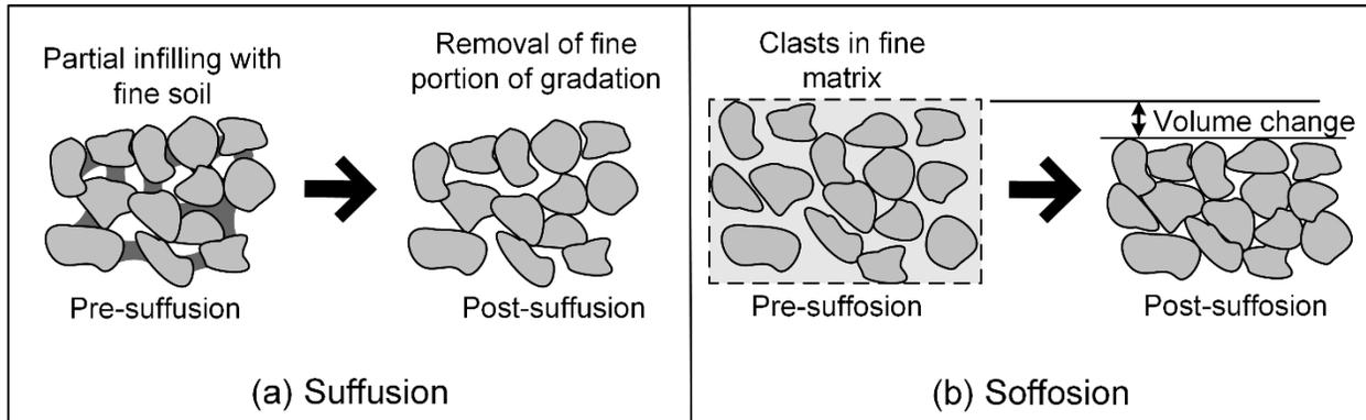
**Figure 6-10 Internal Instability – (a) Suffusion and (b) Suffosion**
