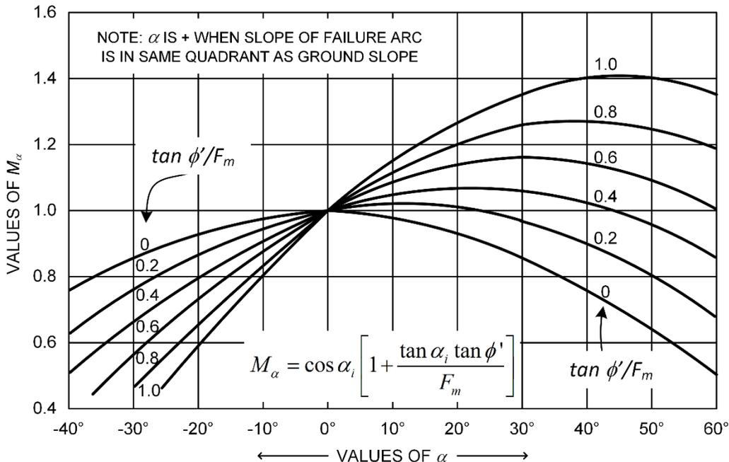
Figure 7-4 Example Slope Stability Analysis using Bishop's Simplified Method for an Effective Stress Analysis
