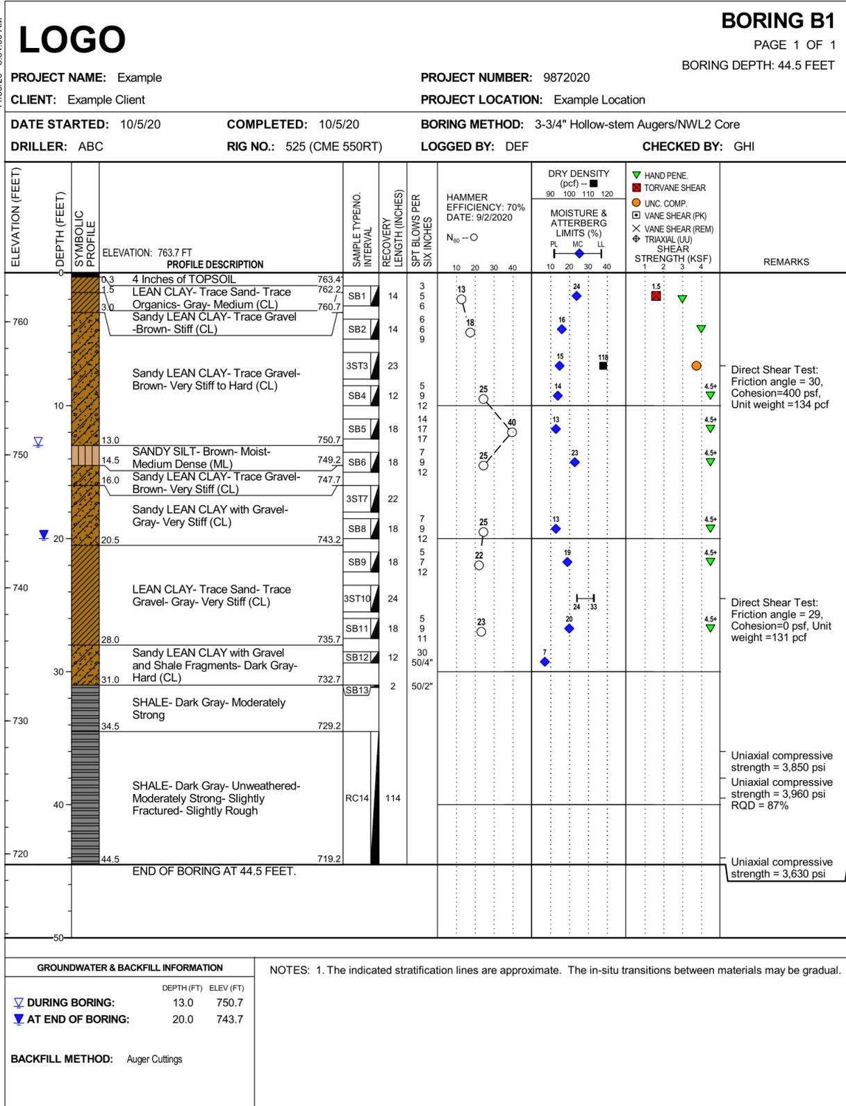
**Figure 2-6 Example Geotechnical Boring Log**
