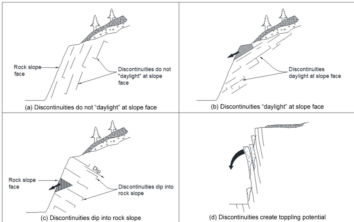
**Figure 7-13 Rock Discontinuity Conditions (after FHWA 1998)**
