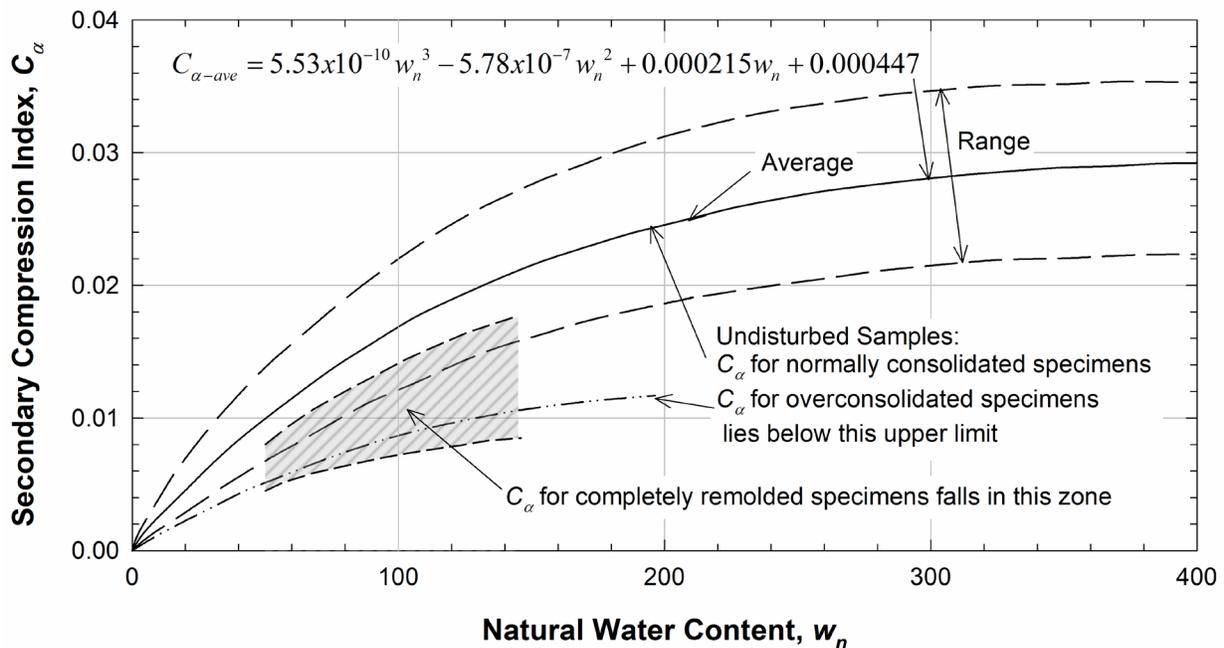
**Figure 8-49 Secondary Compression Index for Silts and Clays**
