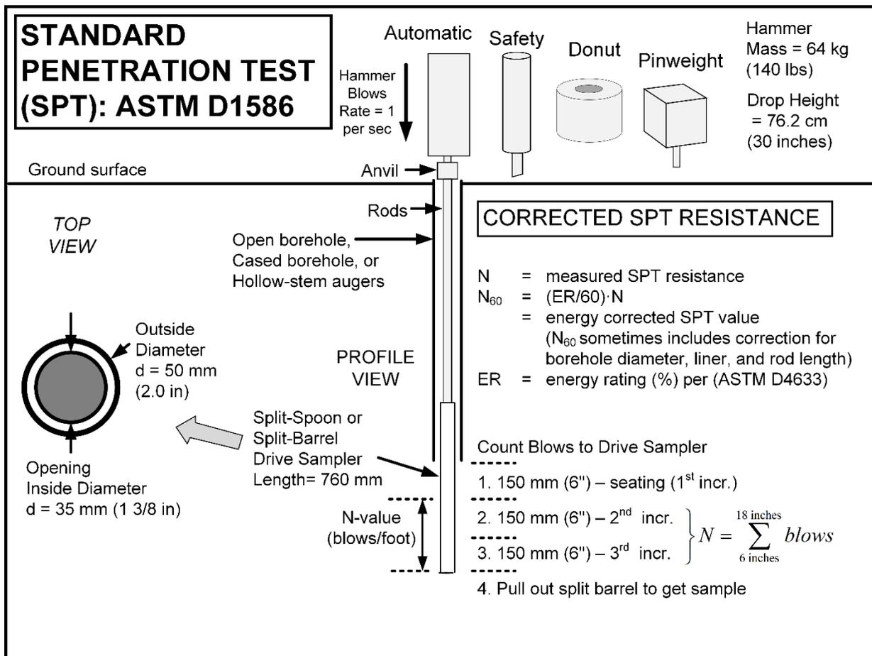
**Figure 2-7 Standard Penetration Test (after NCHRP 2018 and Mayne 2012)**
