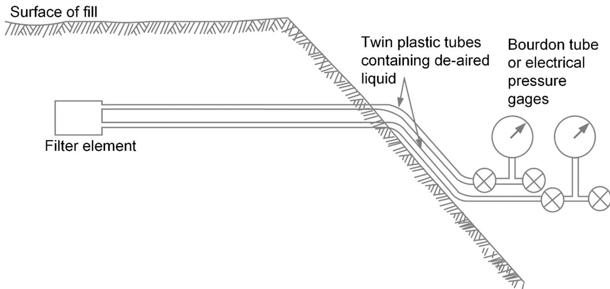
**Figure 2-29 Dual-tube Hydraulic Piezometer in Embankment Dam
