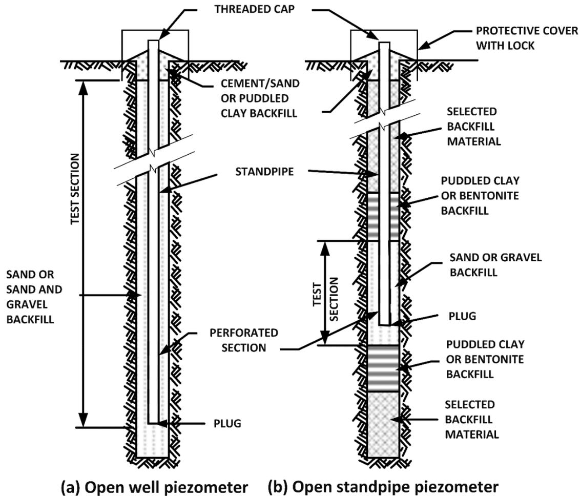
Figure 2-13 Open Piezometers
