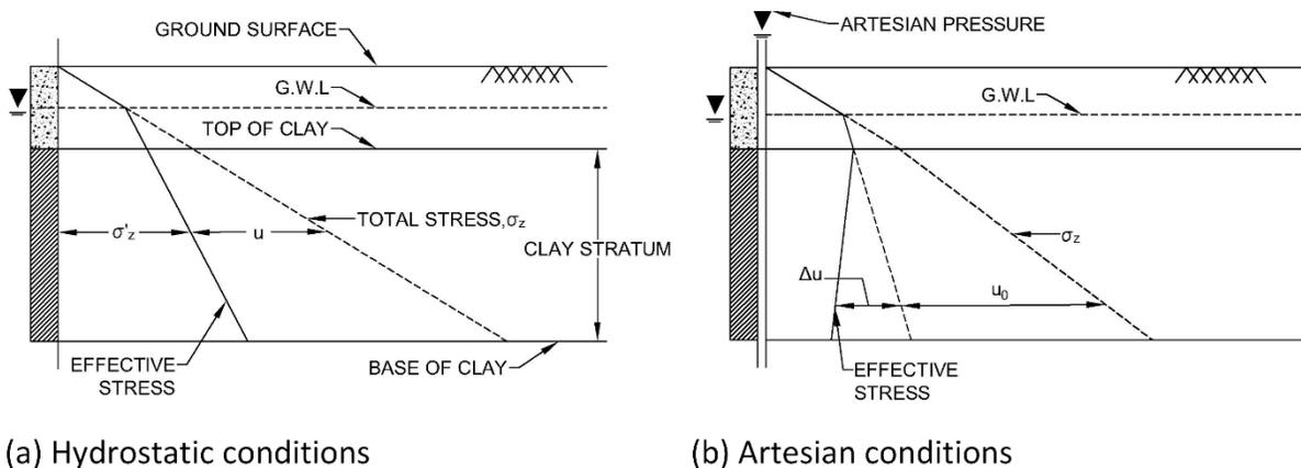
**Figure 5-1 Initial Vertical Stresses for a) Hydrostatic and b) Artesian Pore Water Pressure Conditions**
