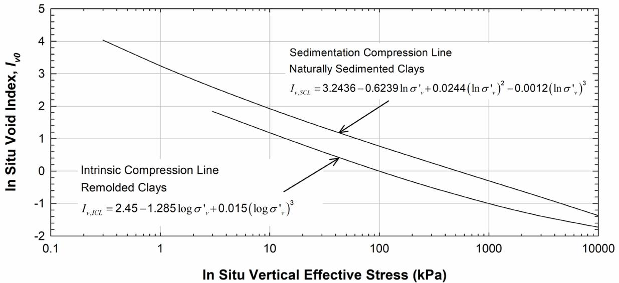
**Figure 8-41 Sedimentation and Intrinsic Compression Lines (after Burland 1990)**
