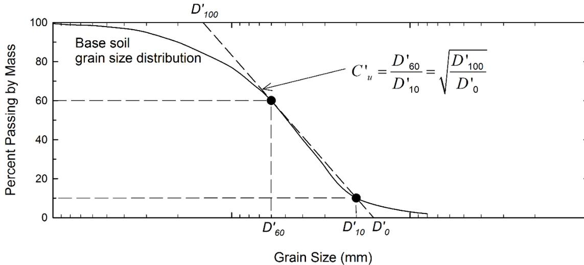
**Figure 6-18 Linear Coefficient of Uniformity (after Giroud 2010)**
