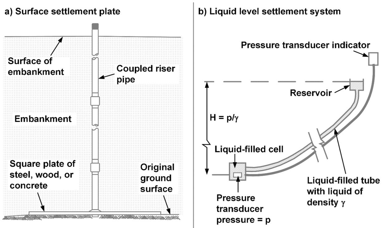
Figure 2-25 Surface Settlement (a) Plate or (b) Platform (after Dunicliff 1993)
