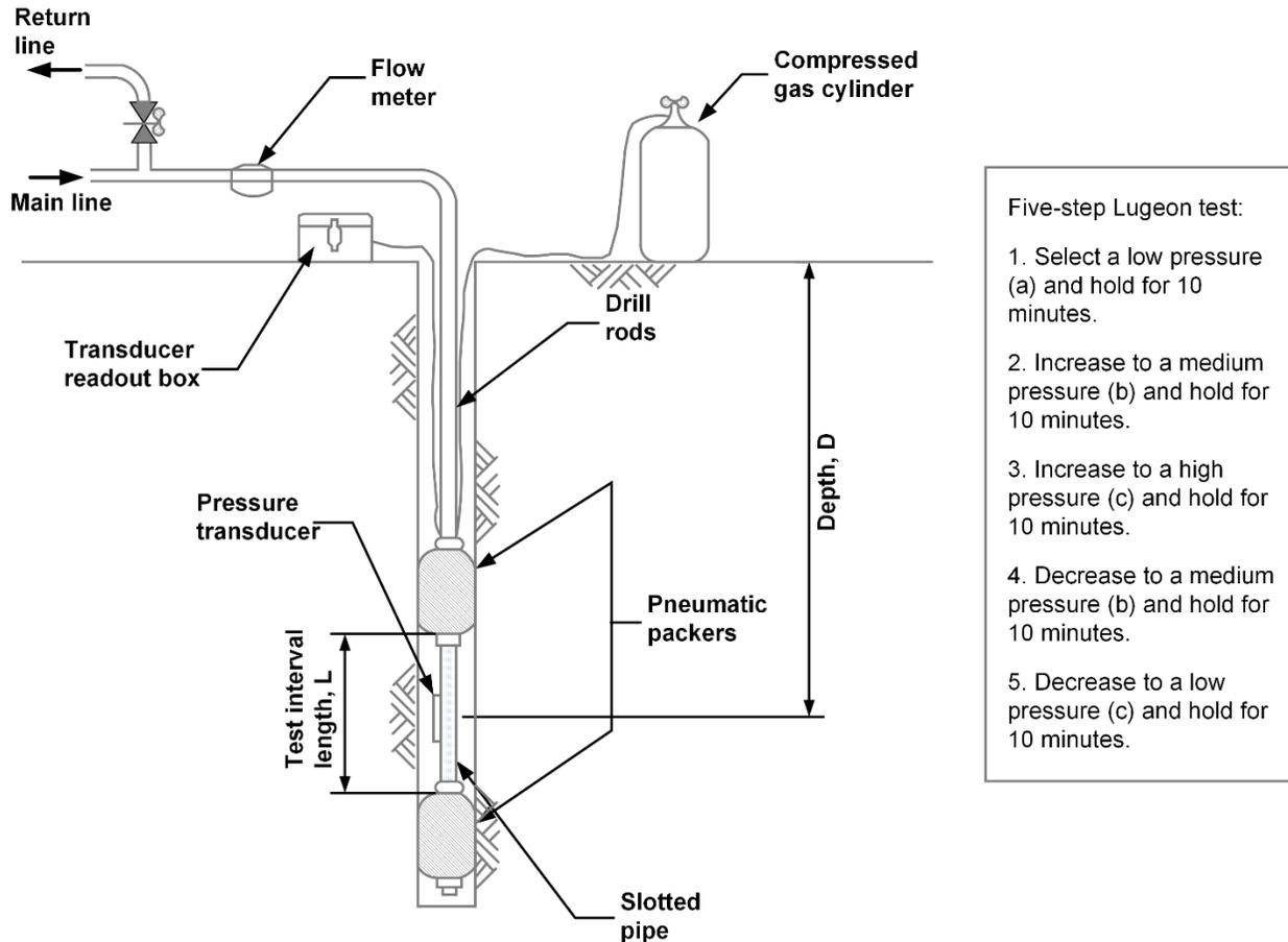
**Figure 2-23 Double Packer Set-up to Conduct Five-step Lugeon test
