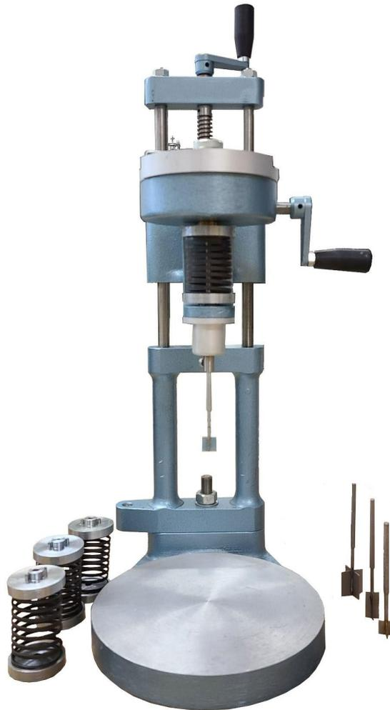
**Figure 3-9 Laboratory Miniature Vane Shear Apparatus**
