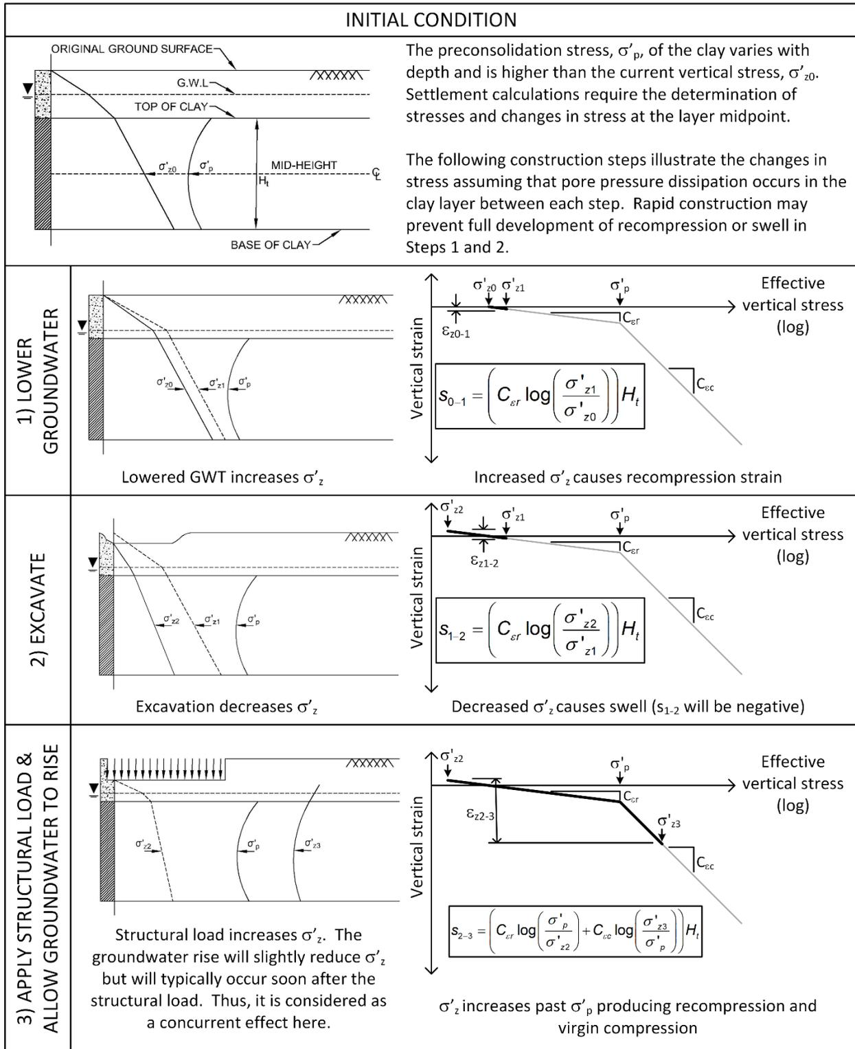
**Figure 5-14 Vertical Movements during a Typical Construction Process**
