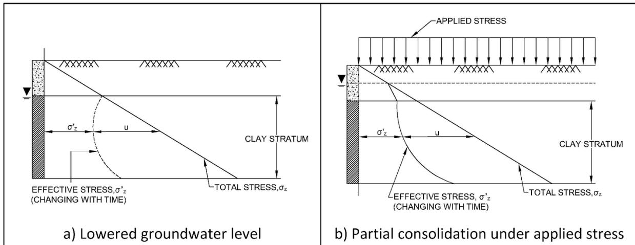
**Figure 5-3 Vertical Stress Profile Cases – Transient**
