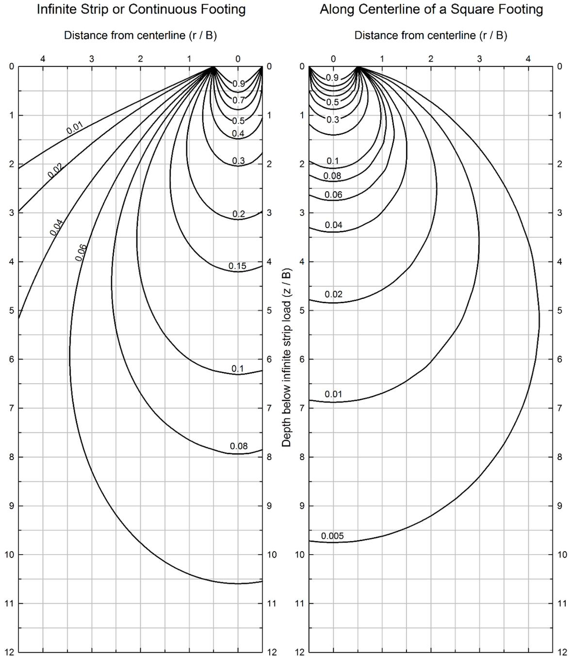
Variables: B = foundation width, r = horizontal distance from centerline of foundation, and z = depth below the applied load.
