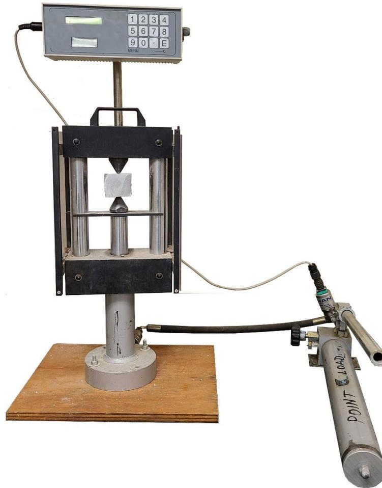
**Figure 3-18 Point Load Apparatus for Rock Index Testing**
