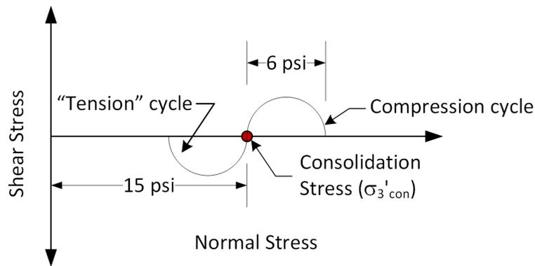
**Figure 3-11 Loading Function and Stresses Applied for a Cycle of Loading in a Cyclic Triaxial Test for a Cyclic Stress Ratio of 0.2**
