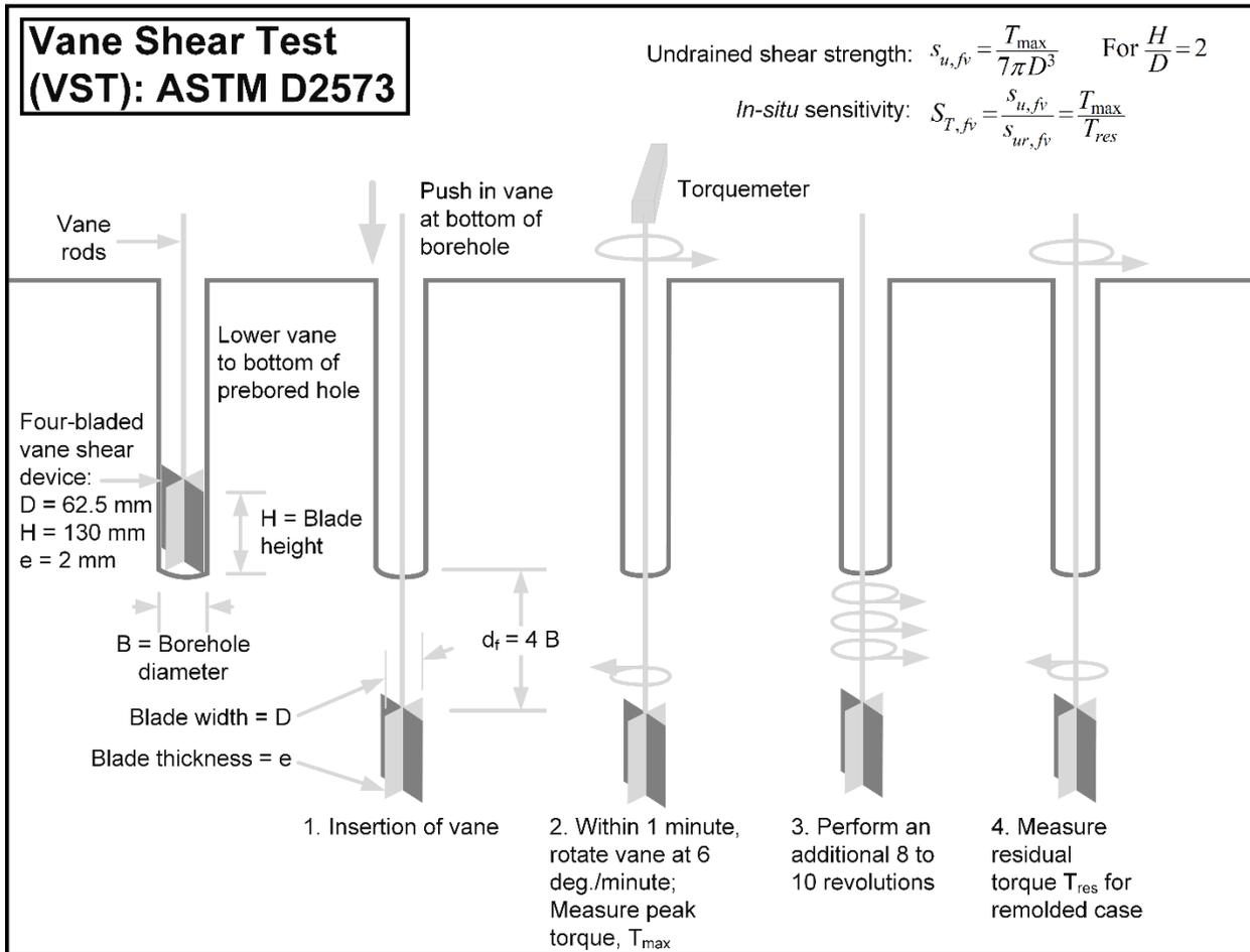
**Figure 2-17 Schematic of Vane Shear Test (after Mayne 2012)**
