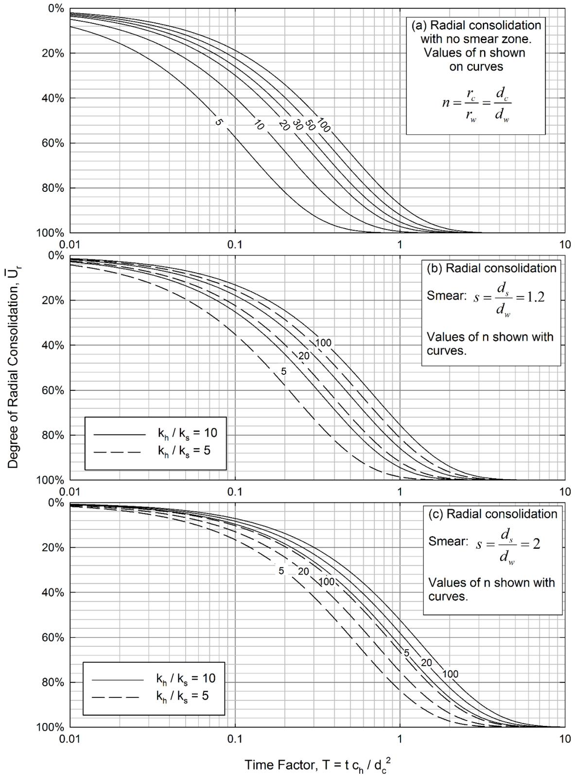
Figure 5-30 Degree of Radial Consolidation
