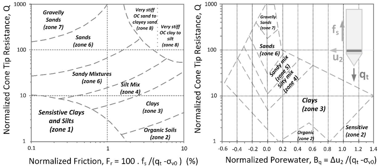
**Figure 2-9 Nine Zone (Normalized) Soil Behavioral Chart for CPT
