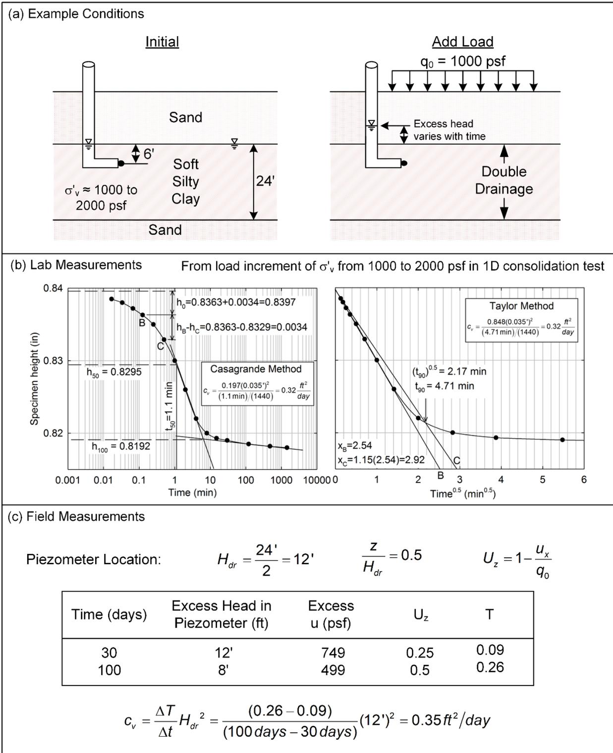
**Figure 5-22 Determination of  $c_v$  from Lab and Field Data**
