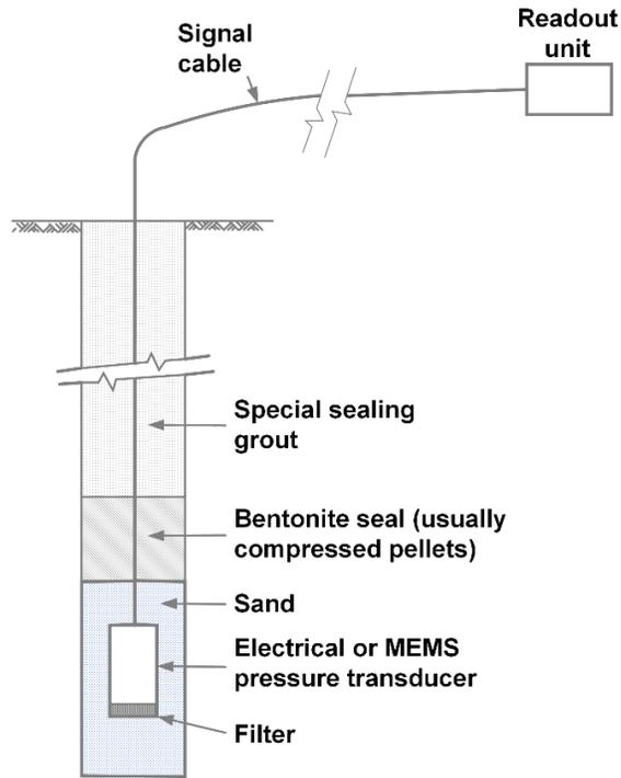
Figure 2-30 Example of Electrical Diaphragm Piezometer Transducer (after Dunnycliff 1993)
