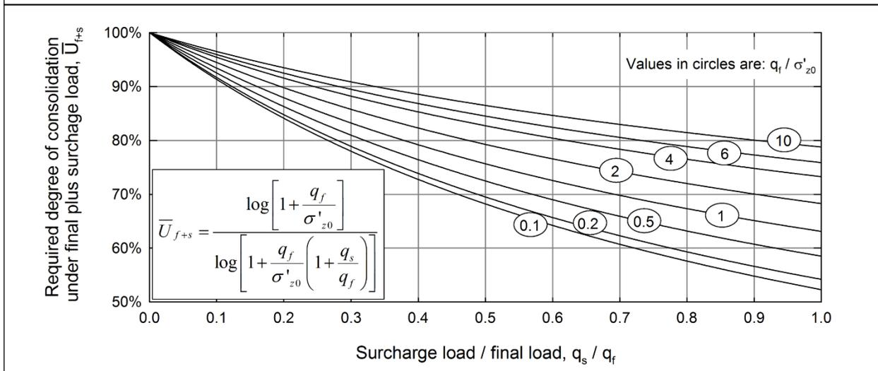
**Figure 5-27 Surcharge Load and Consolidation Required to Eliminate Settlement under Final Load**
