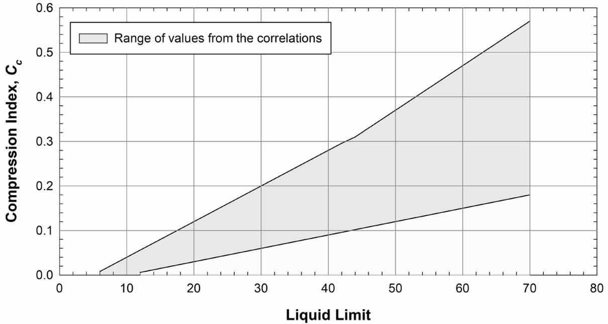
Figure 8-33 Range of Compression Index based on Liquid Limit Predicted by Correlations
