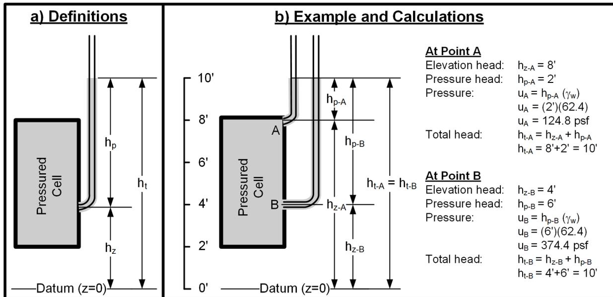
**Figure 6-1 Example of the Components of Hydraulic Head**
