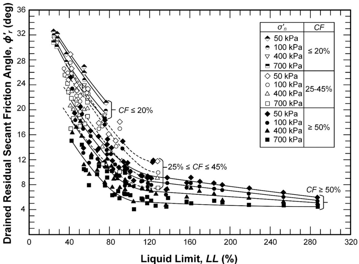
**Figure 8-22 Drained Residual Secant Friction Angle as a Function of  $LL$  and  $CF$**
