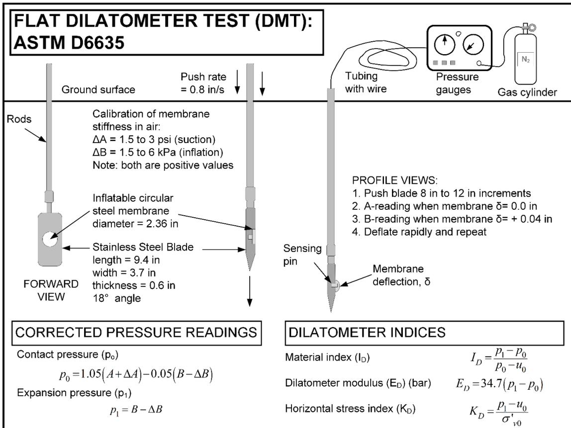
**Figure 2-10 Flat Plate Dilatometer Test Schematic
