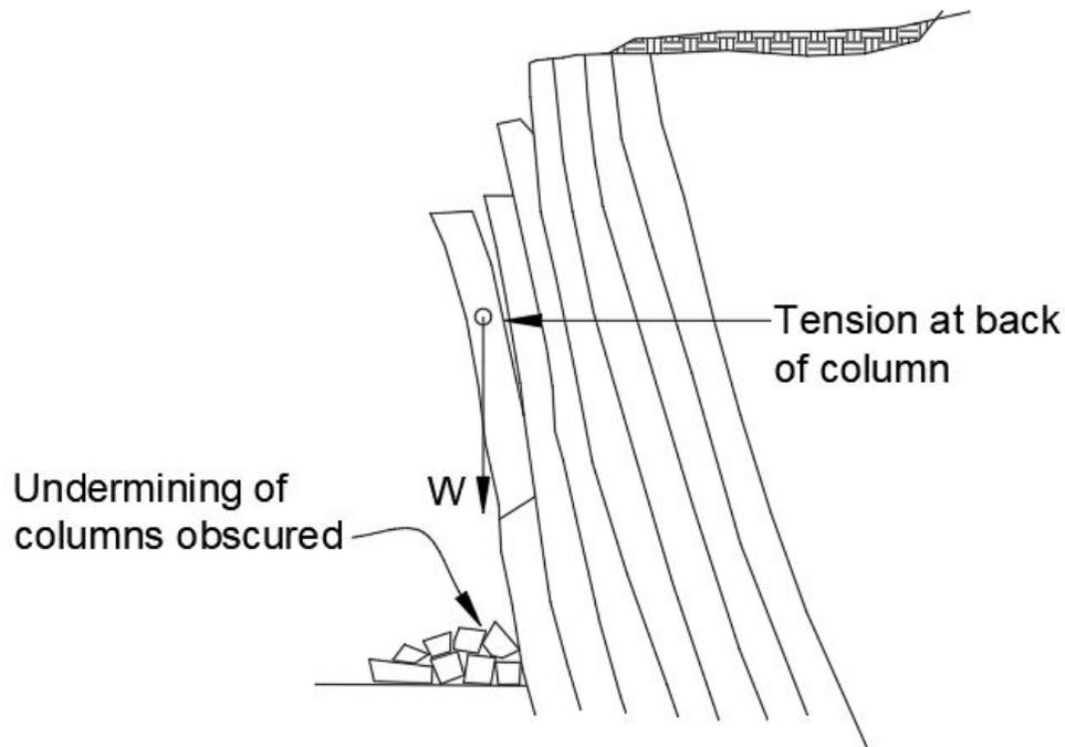
**Figure 7-21 Rock Slope Subject to Toppling Failure**
