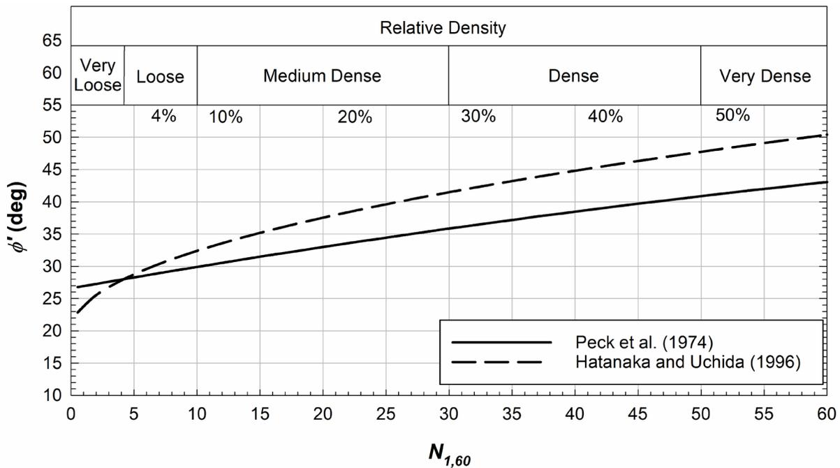
**Figure 8-4 Variation of Effective Stress Friction Angle with  $N_{1,60}$
