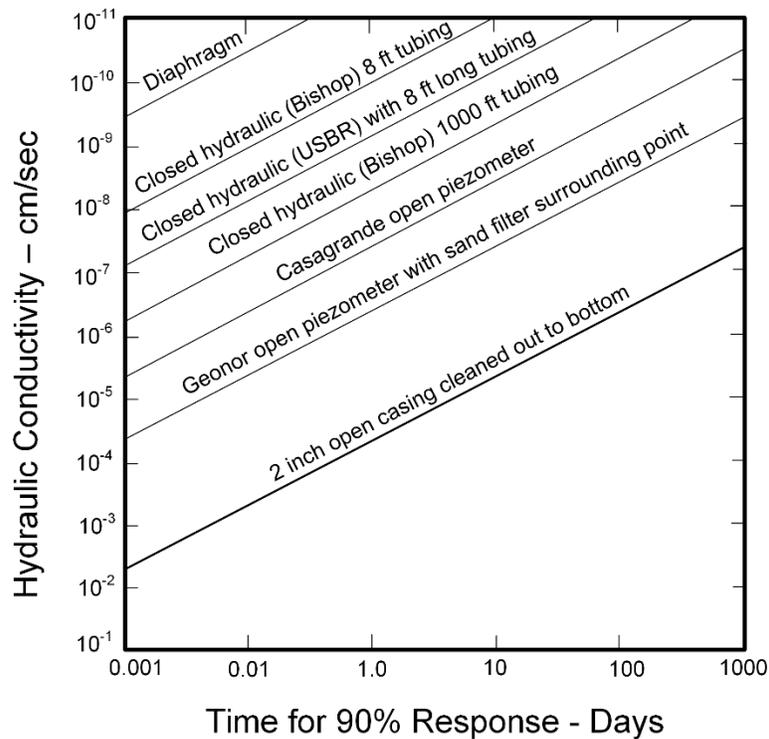
Figure 2-31 Estimated Hydrodynamic Lag Time for Various Piezometers and Wells (after Dunnycliff 1993)
