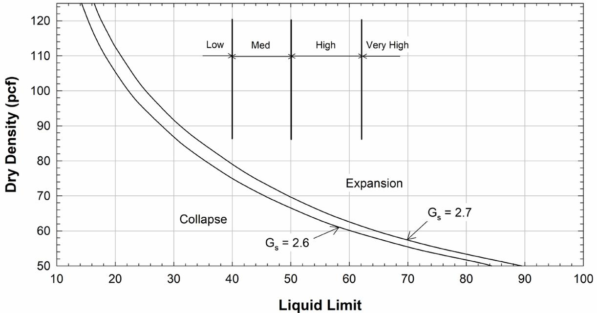
**Figure 1-9 Collapsibility Based on *In situ* Dry Density and Liquid Limit**
