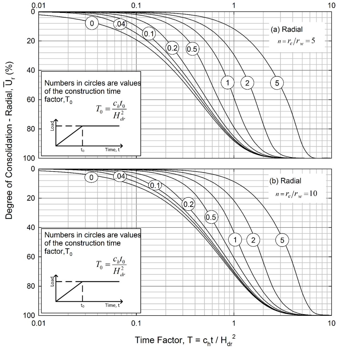
Figure 5-31 Radial Consolidation with Gradual Loading (after Olson 1977)
