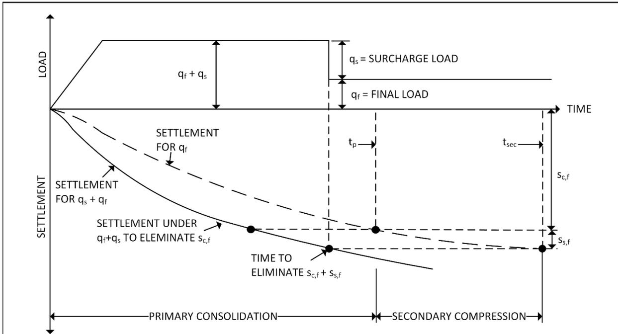
BY SELECTING AN APPROPRIATE SURCHARGE LOAD & DURATION OF SURCHARGE LOADING, ALL OR PART OF THE SETTLEMENT UNDER FINAL LOADING CAN BE ELIMINATED
