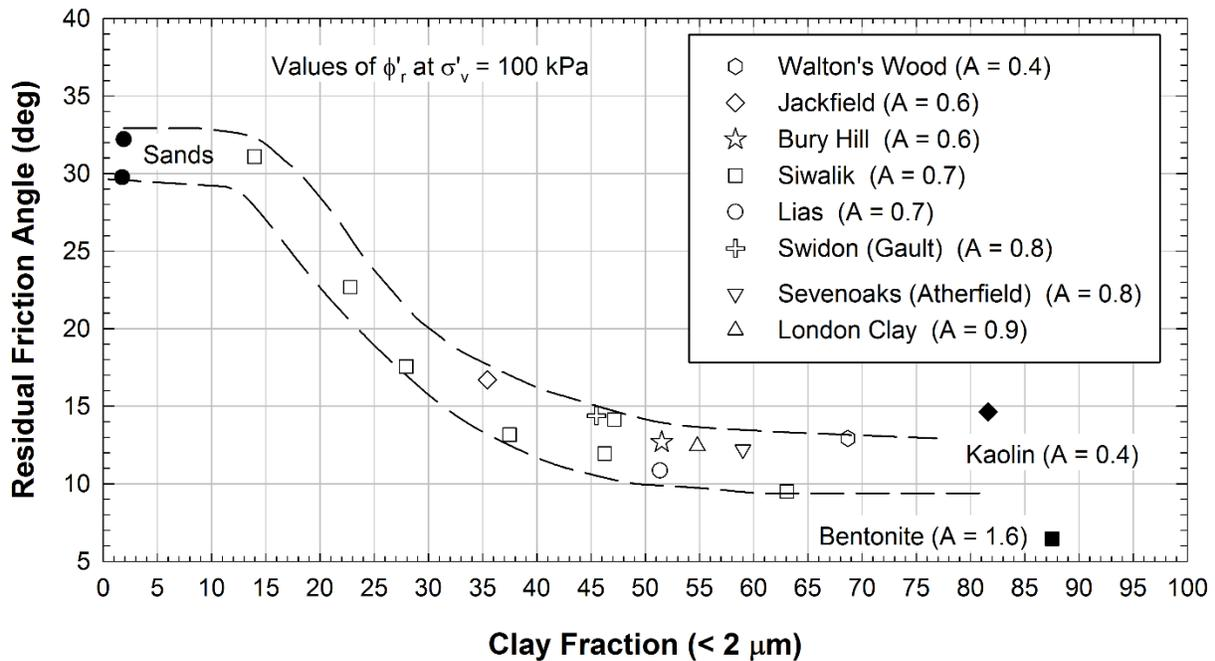
**Figure 8-20 Correlation between the Residual Friction Angle and Clay-sized Fraction (after Skempton 1964, 1985)**
