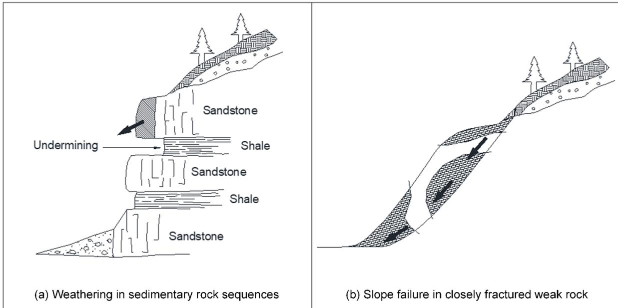
**Figure 7-14 Weathering and Weak Rock Conditions (after FHWA 1998)**
