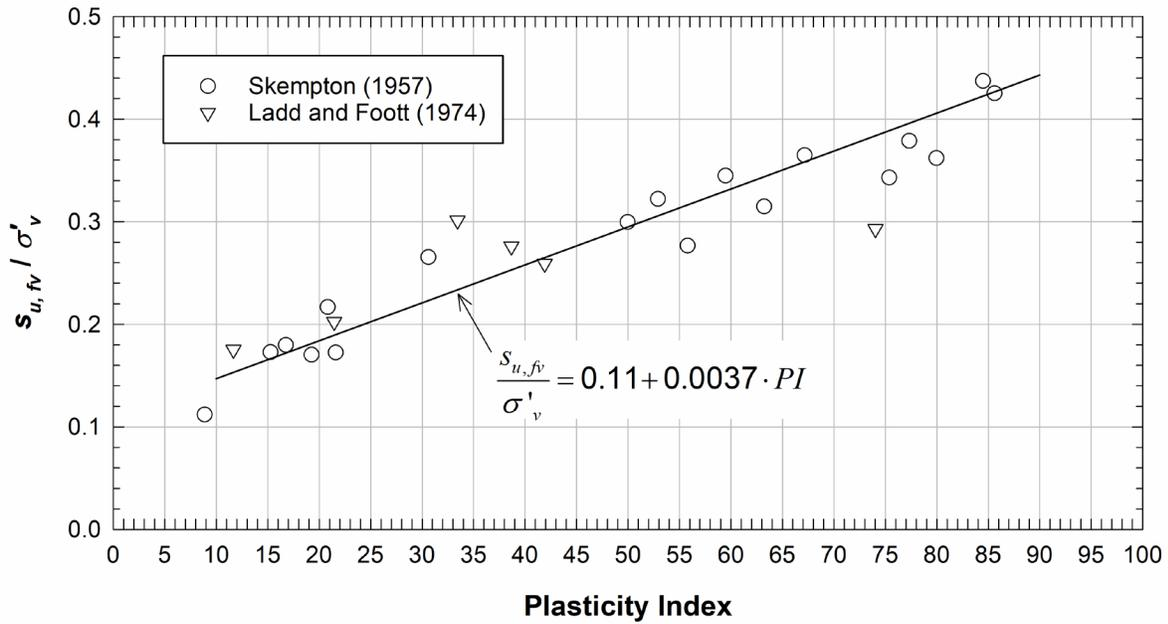
Figure 8-27 Correlation between Undrained Strength Ratio and Plasticity Index – Field Vane (after Robertson and Campanella 1984)
