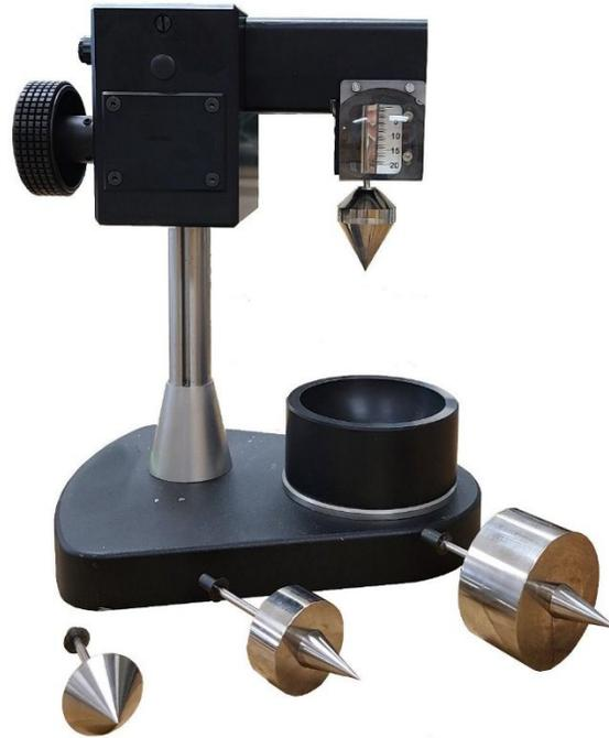
**Figure 3-10 Fall Cone Apparatus**
