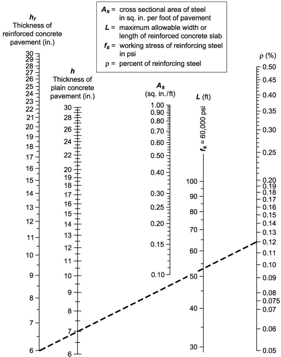
*Reinforced concrete pavement design*
