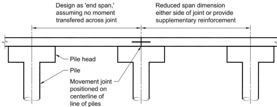
Figure 5-25 Joint Offset from Centerline of Pile within 1/6-1/3 Slab Span
