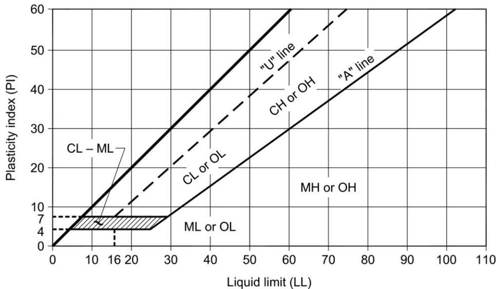
NOTE: The "U" line in Figure 3-1 has been empirically determined and represents the approximate "upper limit" for natural soils. Any test results that fall above or to the left of the "U" line should be verified.
