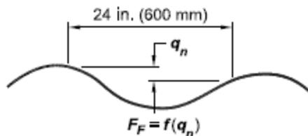
(a) Floor flatness is calculated from elevation readings over 24 inch (600 millimeter) meter) increments
