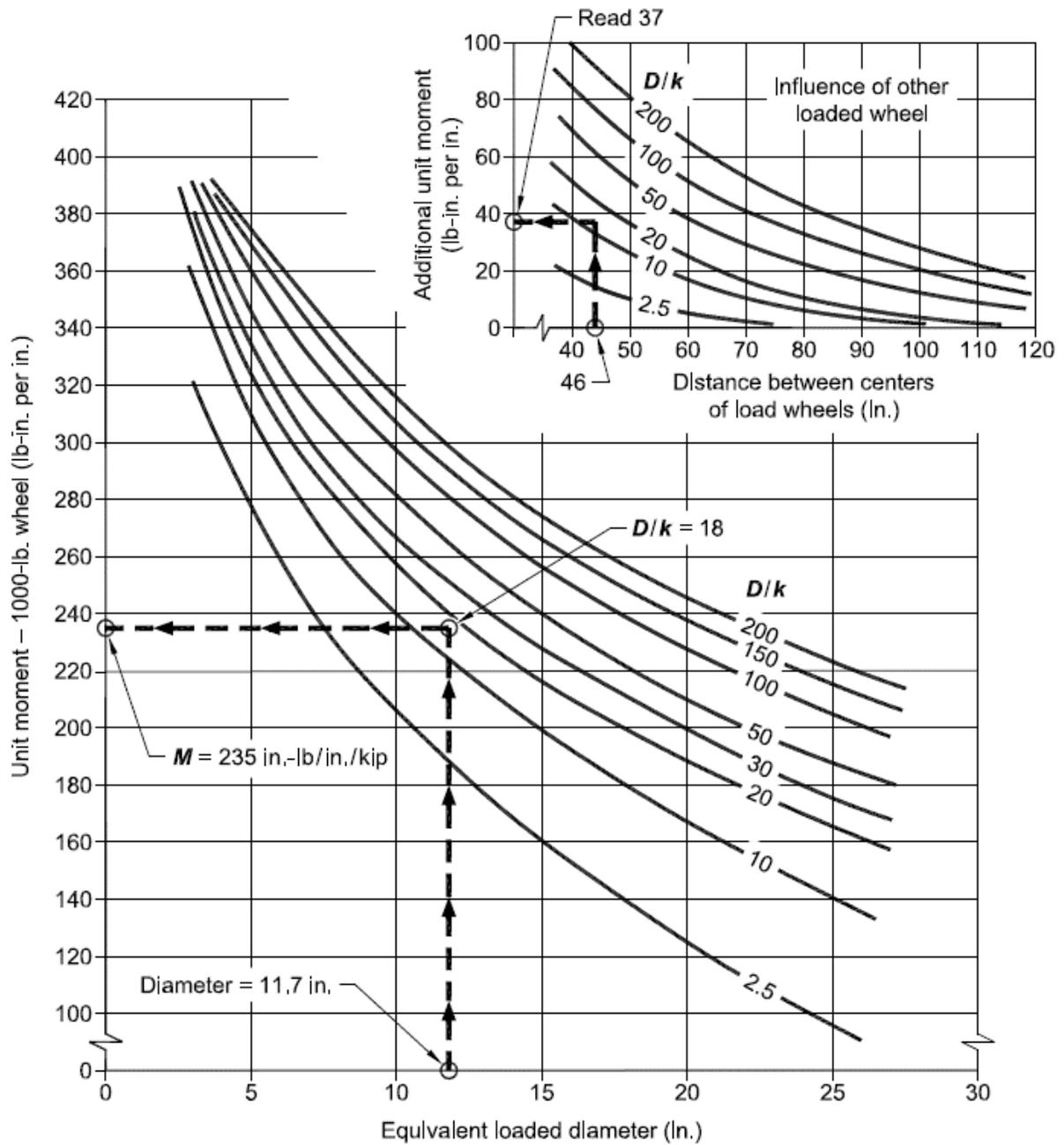
Figure B-3.1c Slab Tensile Stress Charts used with WRI Design Procedure
