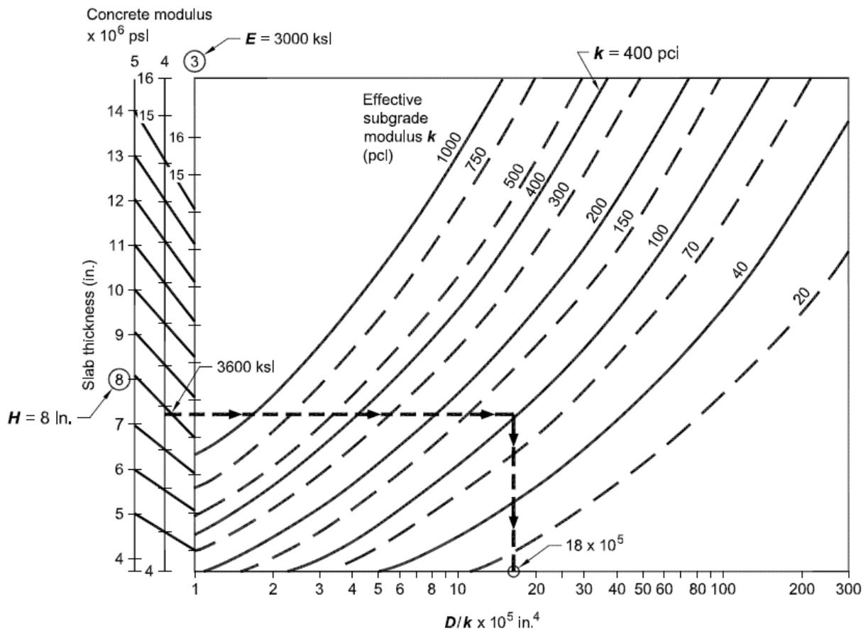
Figure B-3.1b Wheel Loading Design Chart used with WRI Procedure
