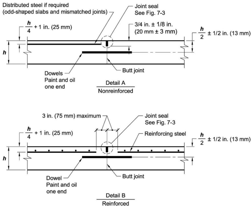
Figure 6-11 **Keyed Construction Joints for Concrete Floor Slabs**
