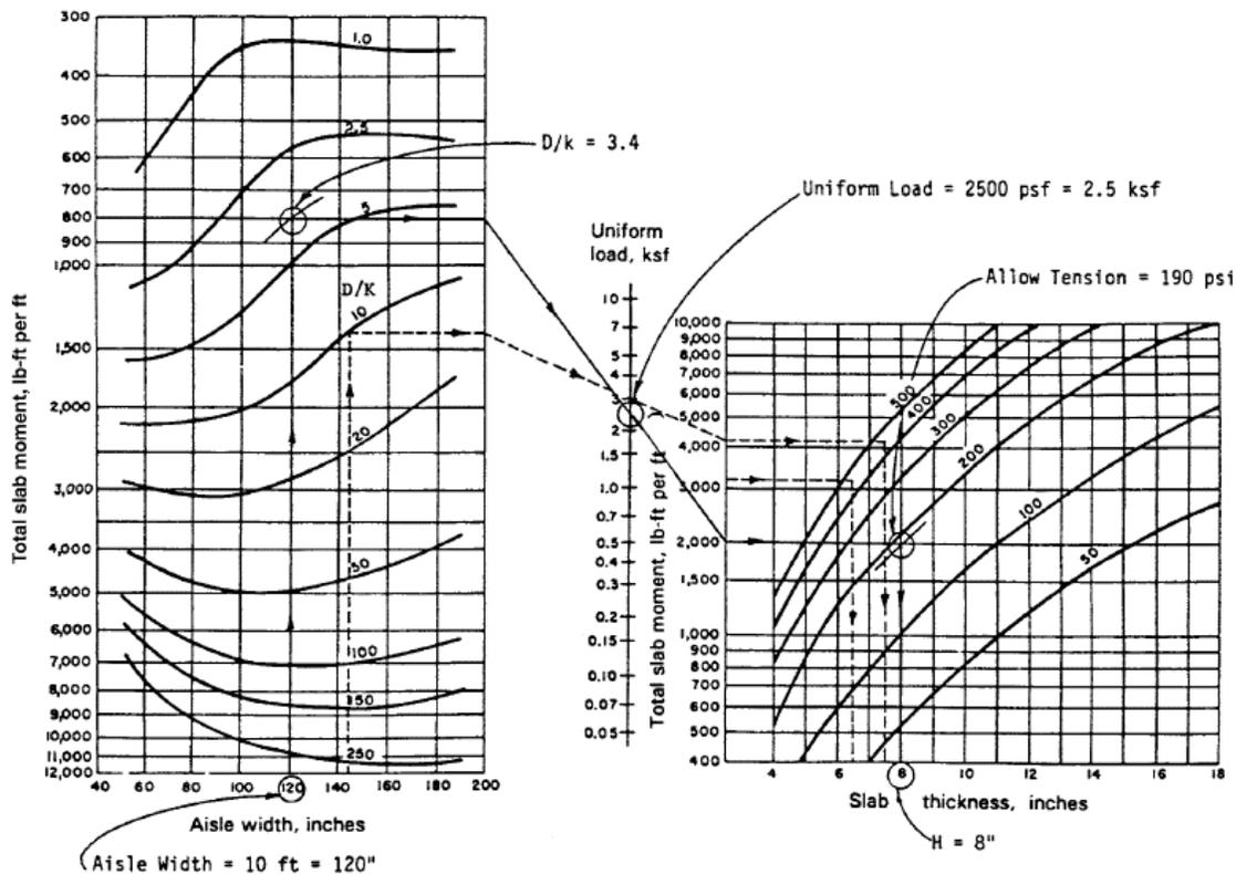
(a) Calculation of slab-on-ground stiffness,  $D/k$       (b) Calculation of slab-on-ground thickness
