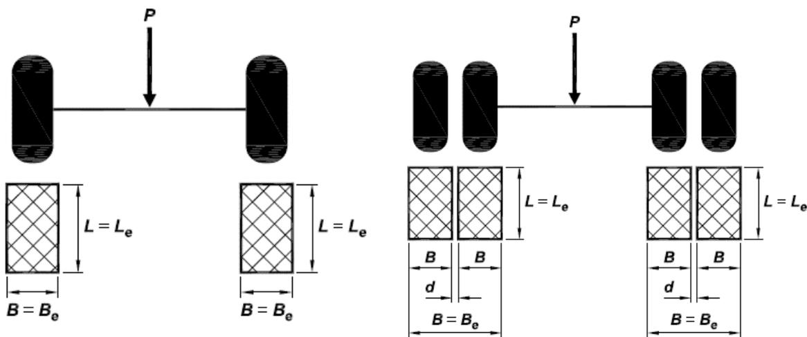
(a) Single tire contact area approximation      (b) Dual tire contact area approximation
