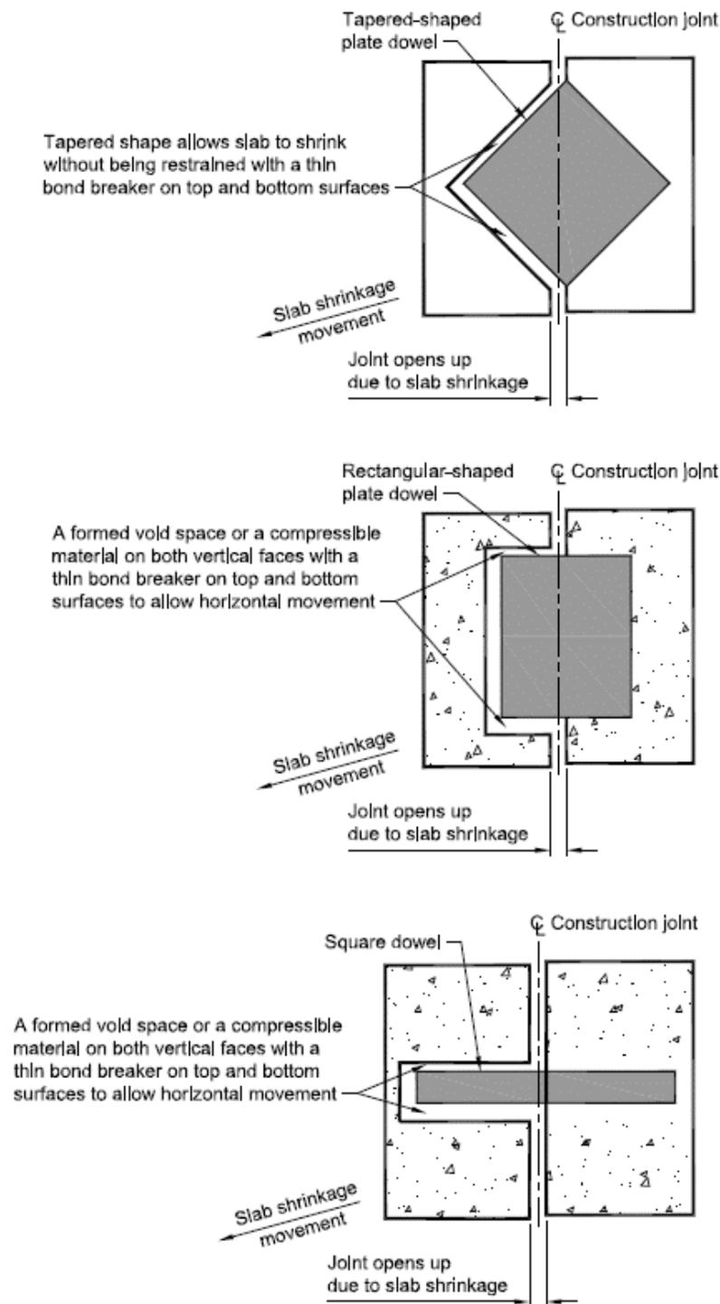
Figure 6-22 Isometric View Indicating Provisions for Longitudinal Movement at Doweled Construction Joints
