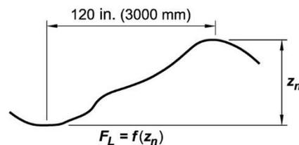
(b) Floor levelness is calculated from elevation readings over 10 foot (3 increments)
