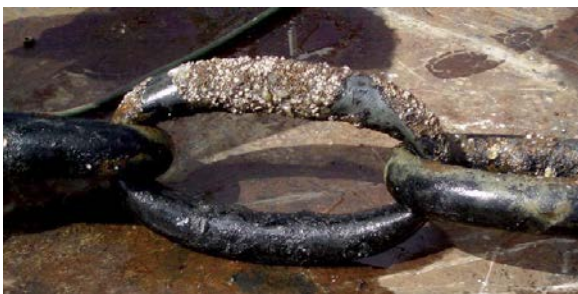
Figure 3-41 Worn 3.5-inch Chain with Stud Missing
