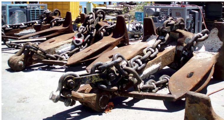
Figure 2-40 Navy Stockless Anchor Rigged as a Sinkers
