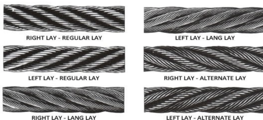
Figure 2-55 Wire Rope Lays
