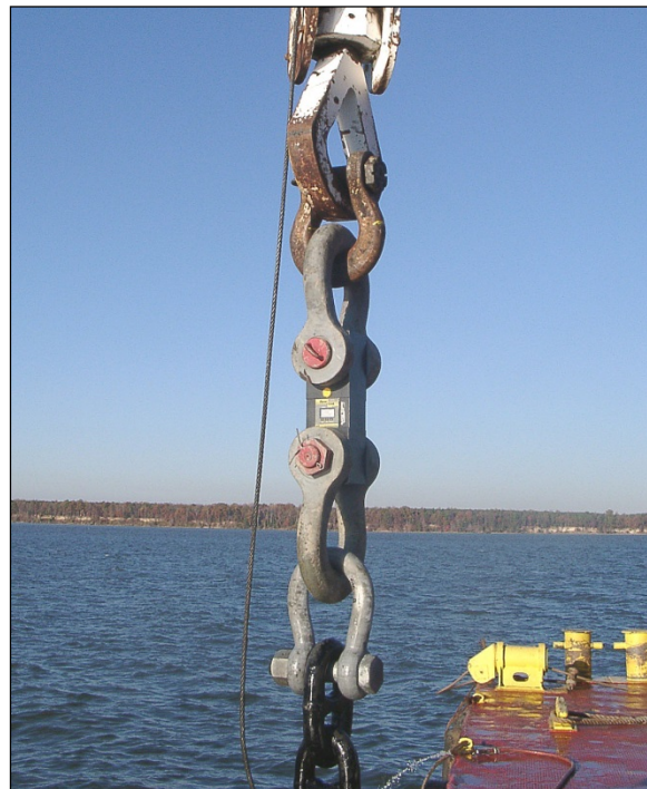
Figure 5-16 Vertical Pull Test Load Cell Positioning
