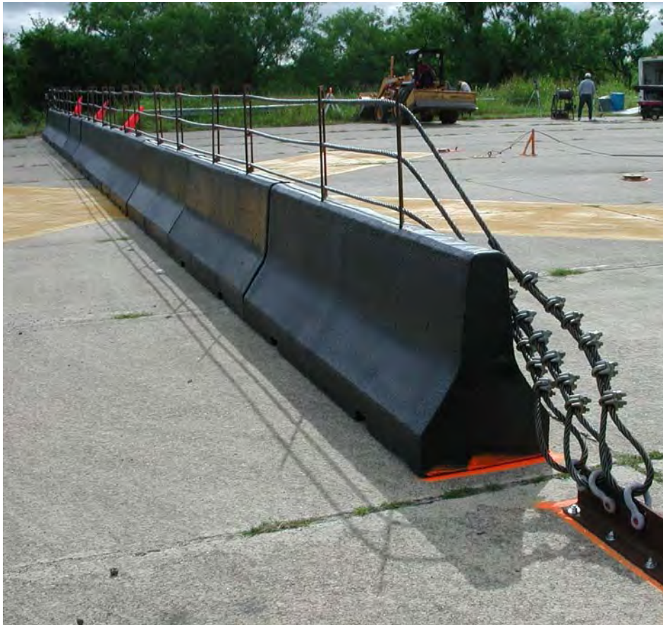
Figure E-4 Polymer-Coated, Lightweight Concrete Barrier System
