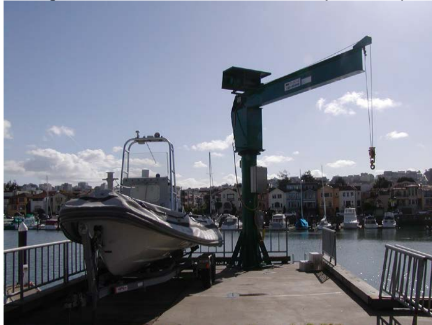
Figure 8-2, Small Craft Crane Access (Jib-boom)
