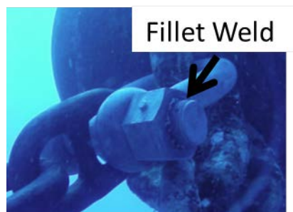
Figure 2-36 Anchor Shackle for Underwater Use
