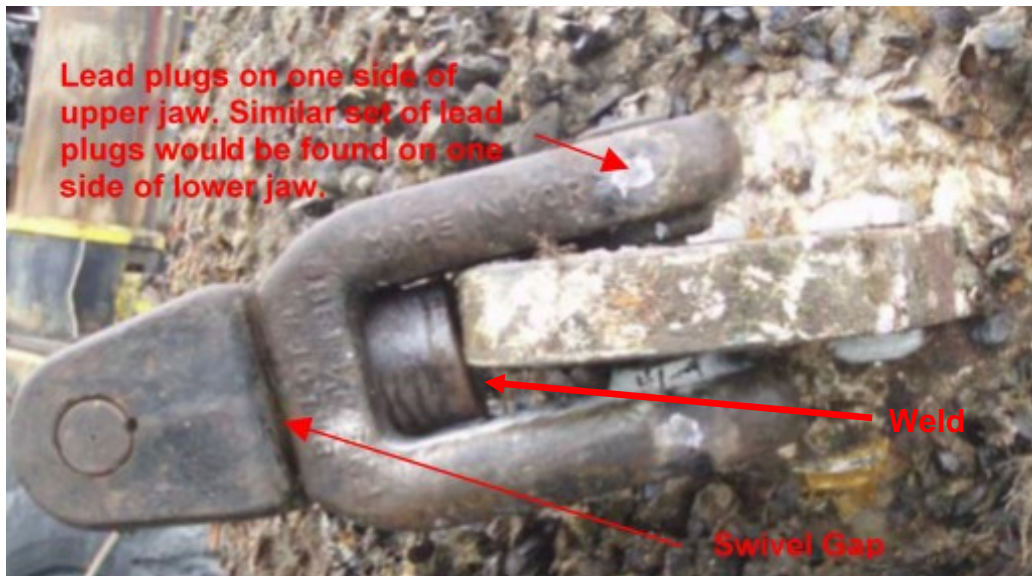
Figure 3-32 Riser Swivel Shackle Inspection Points
