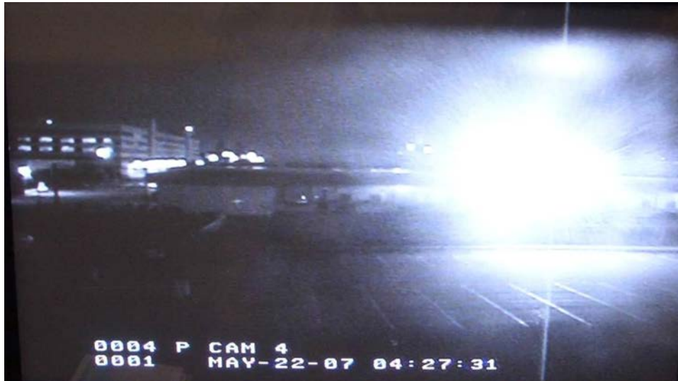
Figure 4-3. Effect of Glare on CCTV Camera Image Quality.
