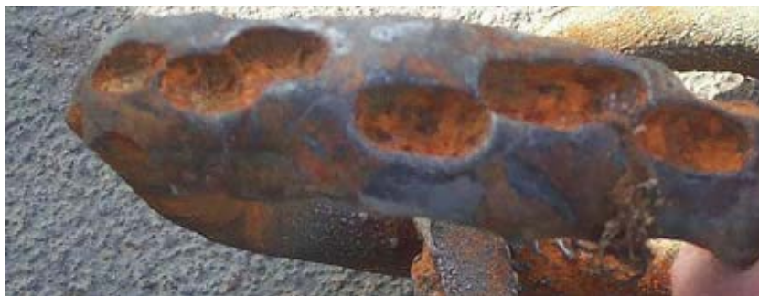
Figure 3-41 Worn 3.5-inch Chain with Stud Missing
