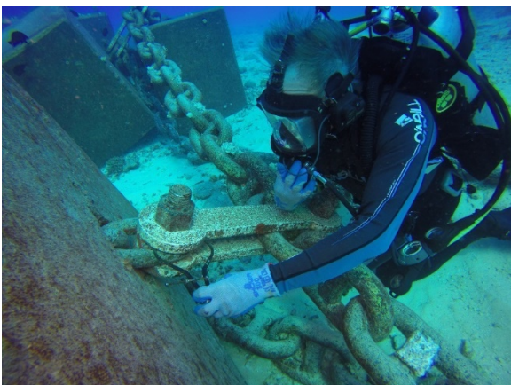
Figure 3-1 Diver Using Tear Drop Calipers
