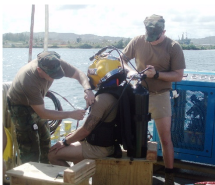
Figure 3-4 Inspection Diver using SCUBA with Diver/Topside Communications Equipment
