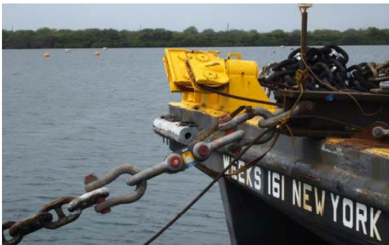
Figure 5-17 Horizontal Pull Test Load Cell Positioning
