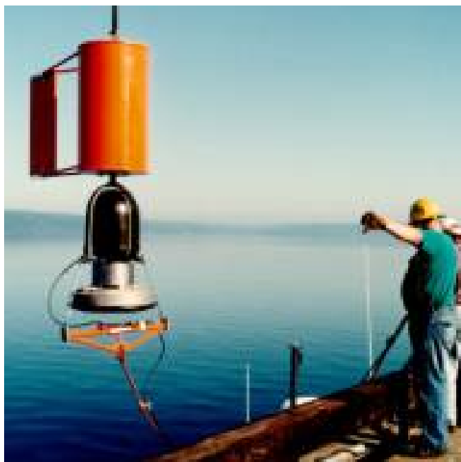
Figure 5-5 Sound Transducer Being Lowered into the Water
