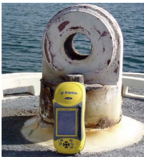
Figure 3-3 Using a Handheld GPS to Survey a Mooring
