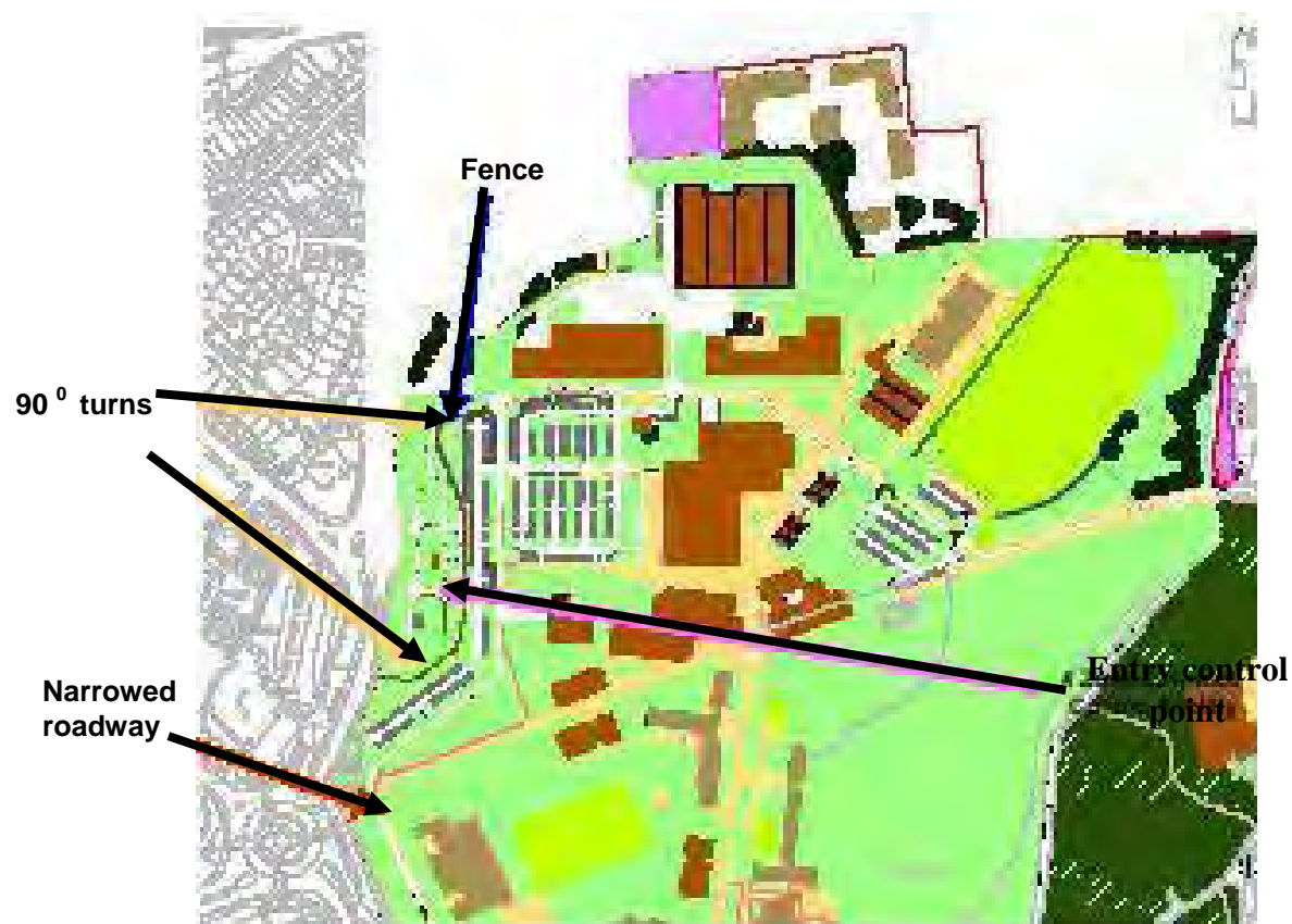
Figure 5-3. Road Modifications to Reduce Speed
