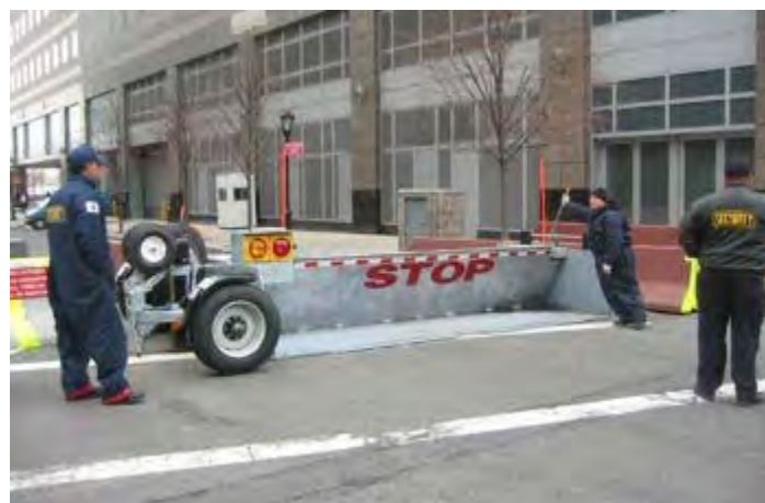
Figure 6-4 Maximum Security Vehicle Arrest Barrier (Example 4)
