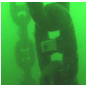
Figure 2-50 Chain Stud Anode Installed
