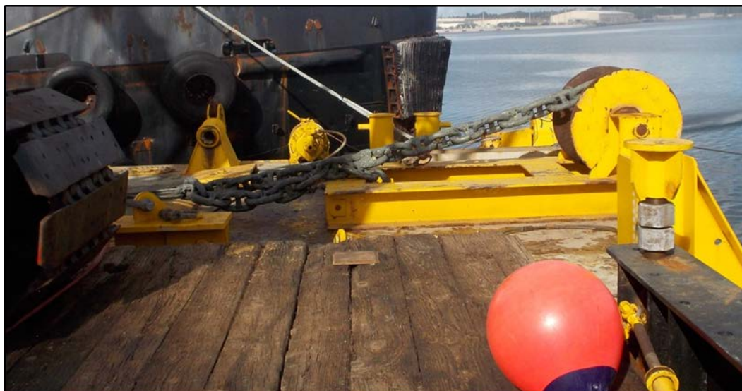
Figure 5-3 Recovery of a Ground Leg over a Roller
