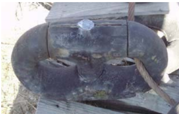
Figure 2-27 Lead Plug in CJL
