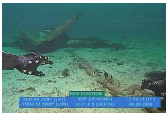
Figure 3-49 Upside Down Anchor and Incorrect Alignment
