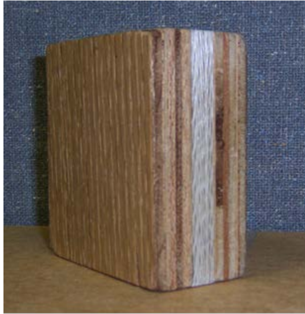
Figure 5-9. Bullet Resistant Fiberglass Door Core
