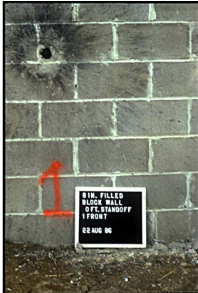
Figure 2-3. Shaped Charge Penetration of Masonry
