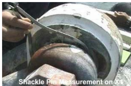
Figure 3-17 Measure Pin Diameter Close to Tension Bar Padeye
