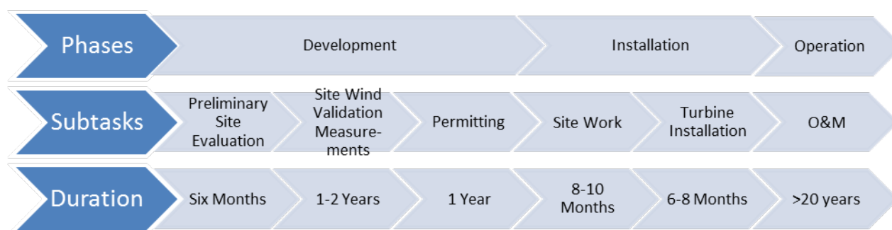
Figure 4-1 Wind Turbine Typical Project Timeline
