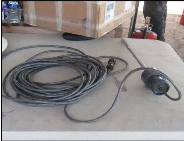
Figure B-16 Probe with Encapsulated Connector.
