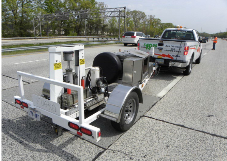
Figure 16-2 Falling Weight Deflectometer
