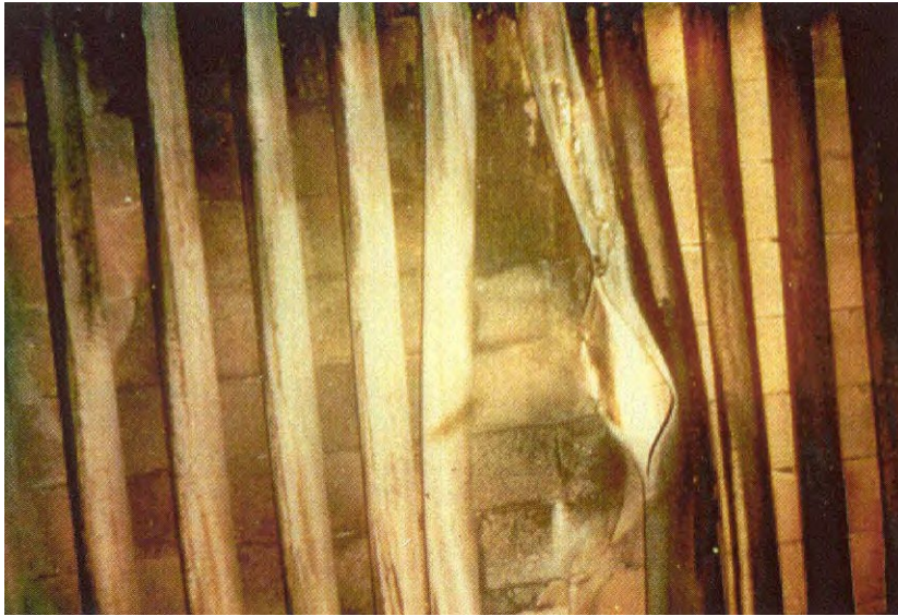
Figure 4-9 Failed Boiler Tube
