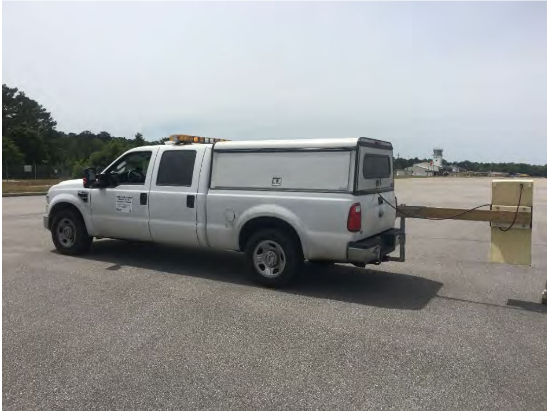
Figure 3-7 Air Coupled GPR
