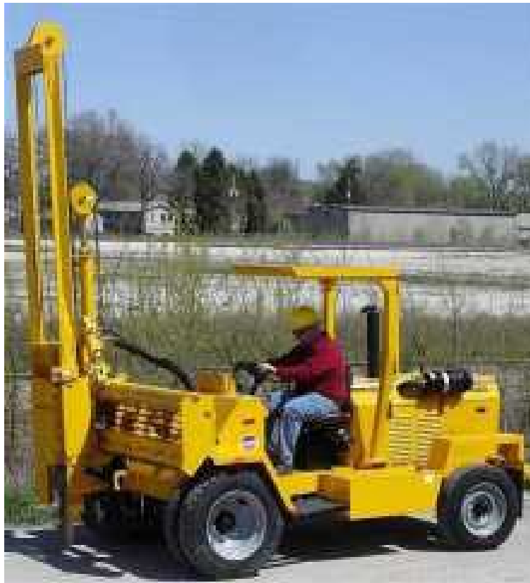
Figure 6-3 Single-Head Hydraulic Drop Hammer*
