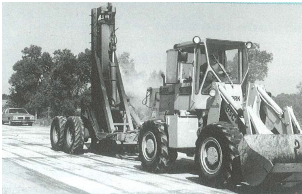
Figure 6-5 Trailer-Mounted Pile Hammer*
