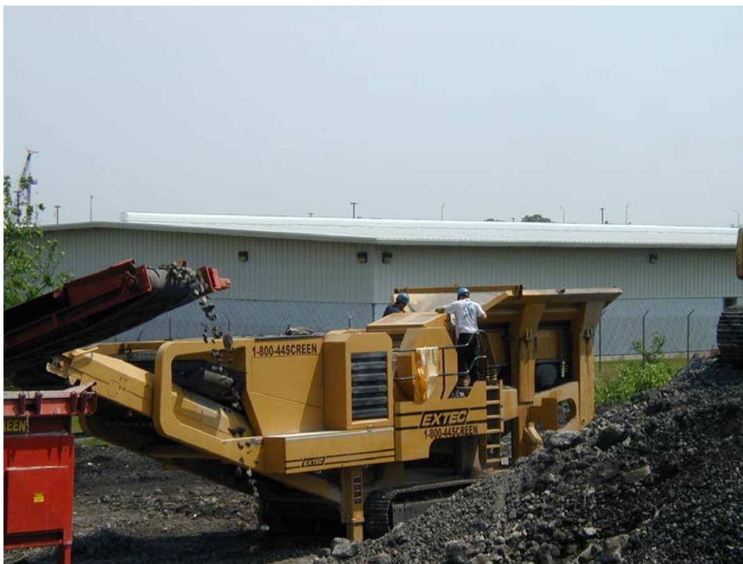
Figure 6-14 Jaw-Type Compression Crusher
