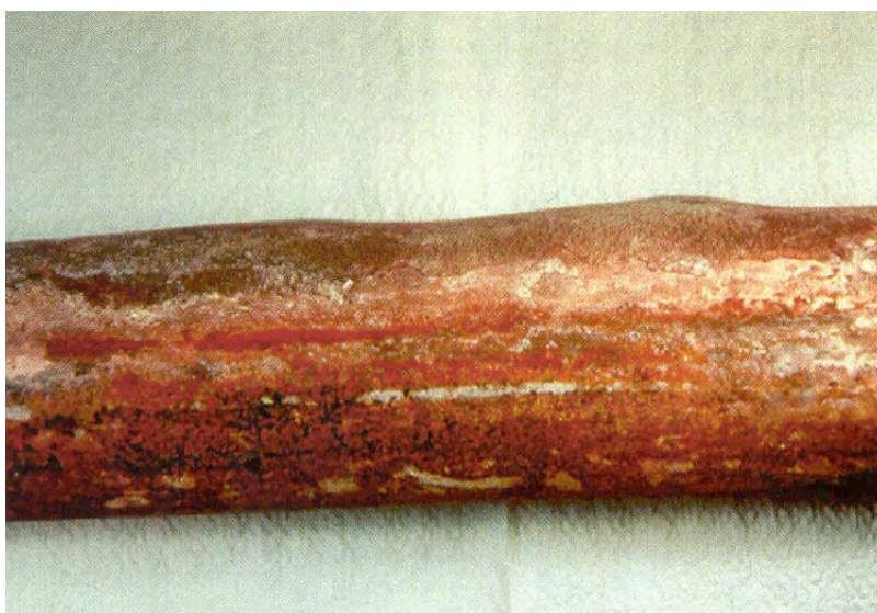
Figure 4-8 Metal Fatigue on Boiler Tube
