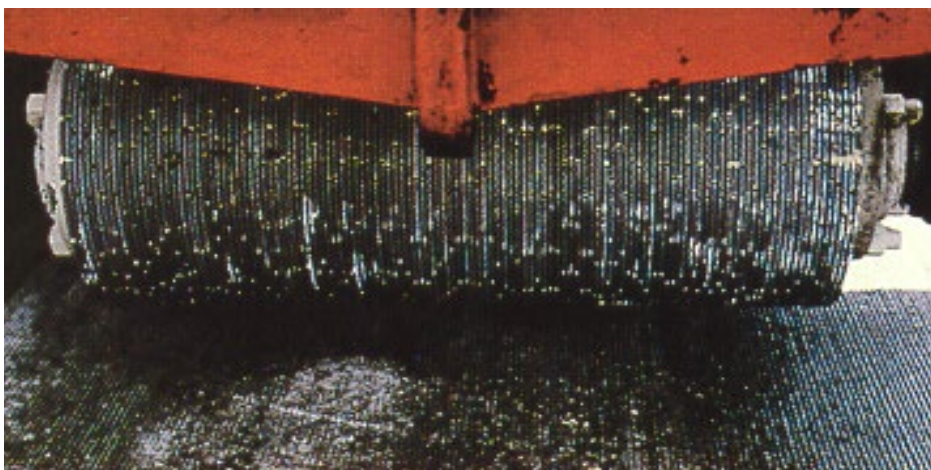
Figure 17-2 Gang-mounted Diamond Saw Blades
