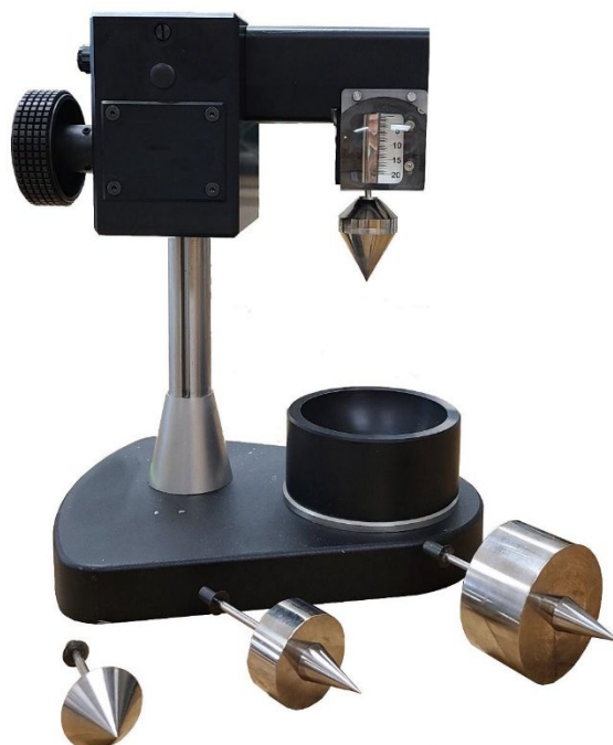
Figure 3-10 Fall Cone Apparatus
