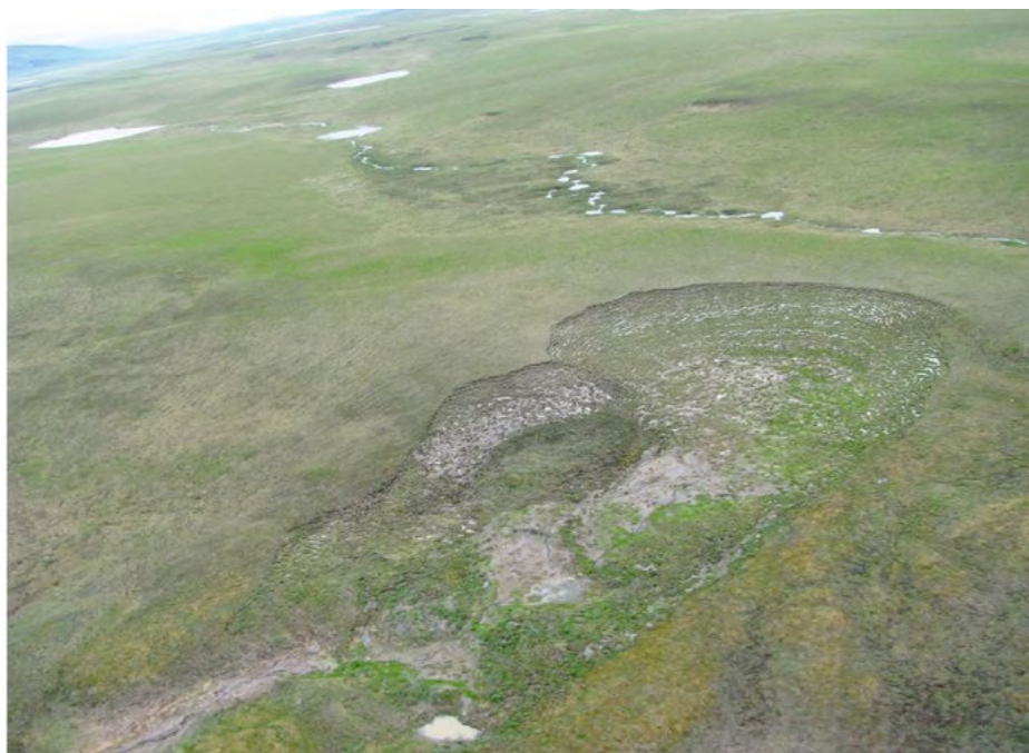
Figure A-4 Retrogressive Thaw Slump (Mackenzie River, Canada)
