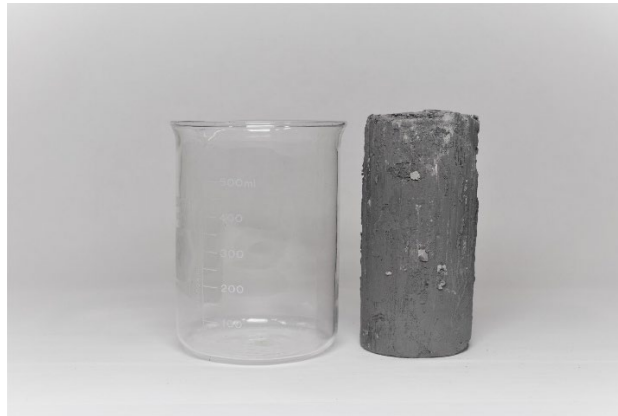
Figure 2-4 After Thawing (Settlement and Strength Loss)
