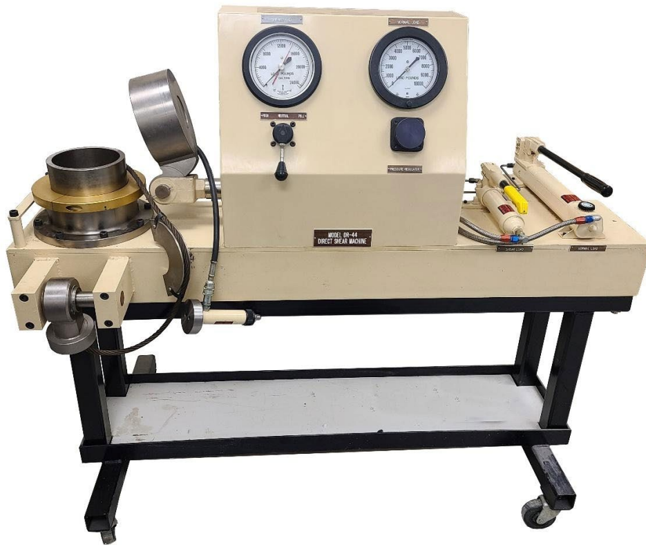
Figure 3-17 Rock Direct Shear Apparatus for High Normal and Shear Loads
