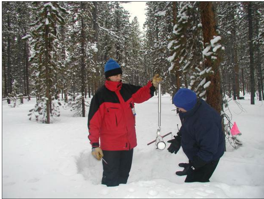
Figure A-1 Weighing a Snow Sample in the Field to Measure SWE
