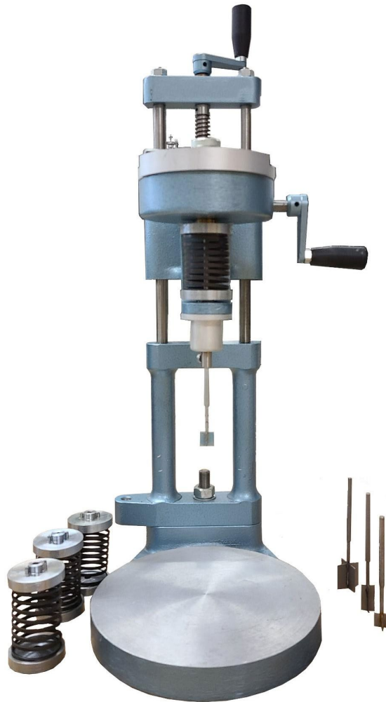
Figure 3-9 Laboratory Miniature Vane Shear Apparatus
