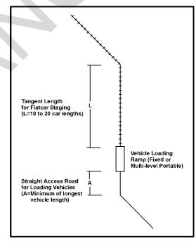
Figure 8-3. Track and Approach Road Lengths for Vehicle Loading
