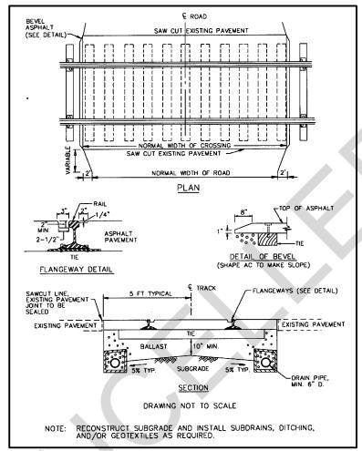
Figure 7-3. Typical Type 3A Asphalt Crossing
