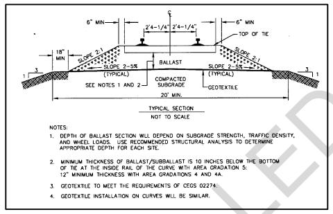
Figure 6-6. Typical Cross Section - Track with Geotextile
