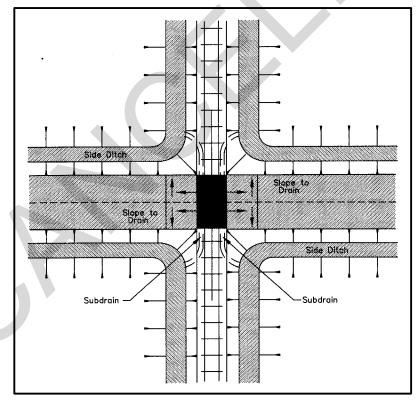
Figure 7-14. Typical Drainage at Road Crossings.
