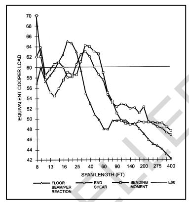
Figure 7-20. Variation in Cooper E Value with Span Length
