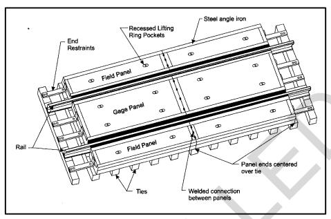
Figure 7-12. Lagless Concrete Panel Crossing
