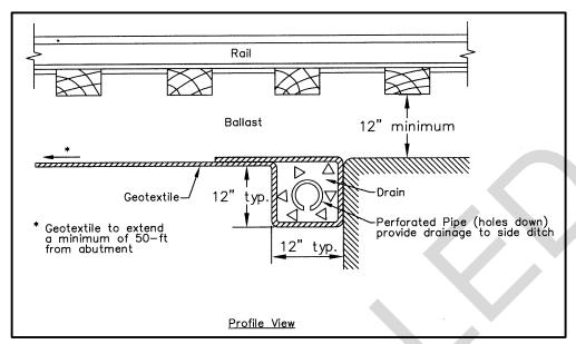
Figure 6-19. Geotextile Installation at a Bridge Abutment
