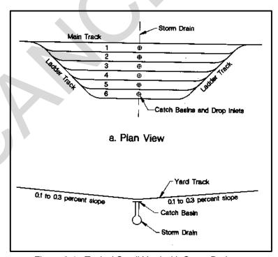
Figure 8-1. Typical Small Yard with Storm Drainage
