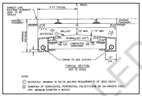
Figure 7-13. Typical Geotextile/Subdrain installation for Vehicle Road Crossings
