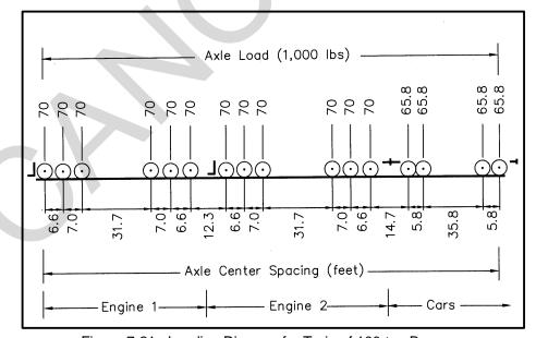
Figure 7-21. Loading Diagram for Train of 100-ton Boxcars.
