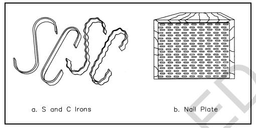
Figure 6-20. Anti-Splitting Devices for Tie Ends
