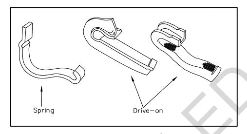
Figure 6-23. Rail Anchors
