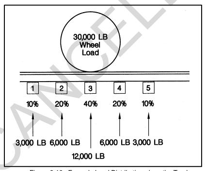
Figure 6-10. Example Load Distribution along the Track
