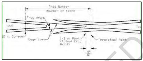
Figure 6-27. Determining Frog Number (Turnout Size)
