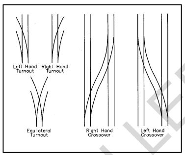
Figure 6-25. General Arrangement of Turnouts and Crossovers
