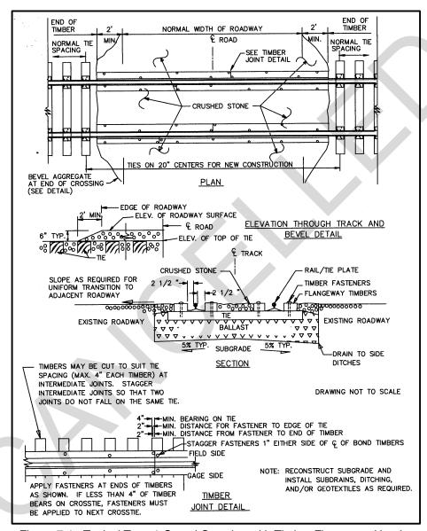
Figure 7-1. Typical Type 1 Gravel Crossing with Timber Flangeway Header
