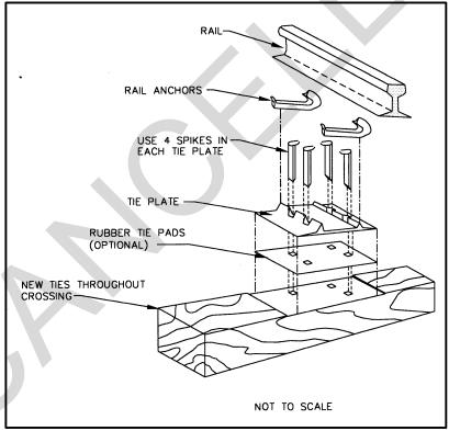
Figure 7-15. Recommended Track Construction for Road Crossings
