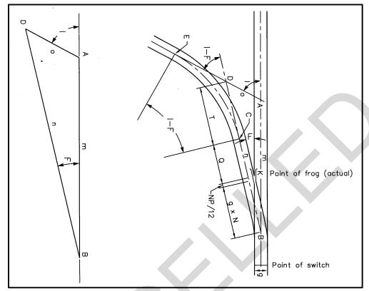
Figure 6-29. Diverging Route Connection
