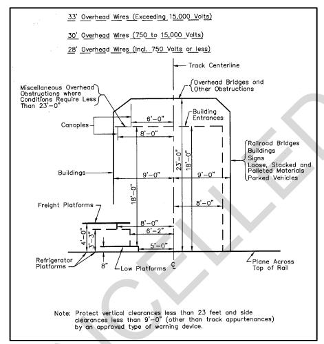
Figure 6-8. Clearance Diagram for Tangent Track
