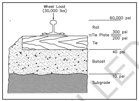
Figure 6-11. Example Vertical Pressure Reduction through the Track
