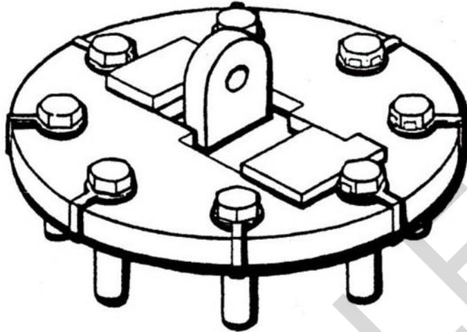
Figure 5-5 Restraint Fitting Type F2, Aircraft Run-up
