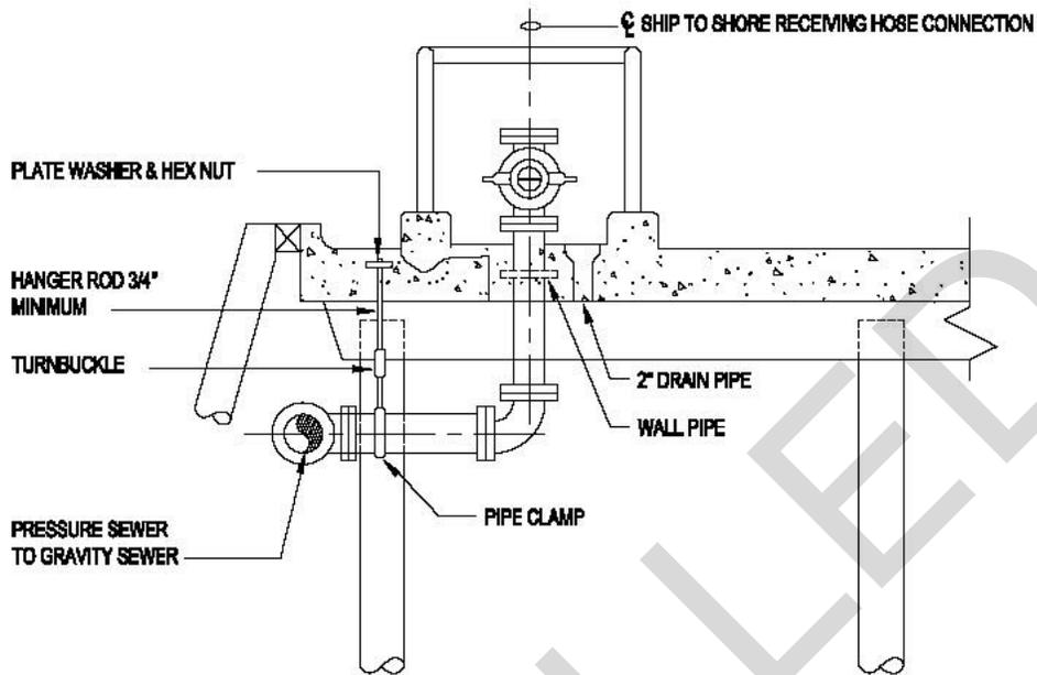
**ALTERNATE PIER SEWER ASSEMBLY**
