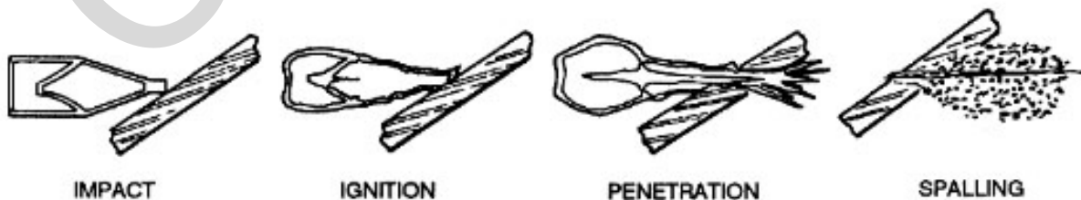
Figure 2-2. Shaped Charge Penetration
