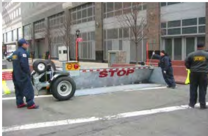
Figure 6-4 Maximum Security Vehicle Arrest Barrier (Example 4)
