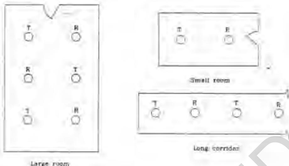
Figure 4-13. Placement of Ultrasonic Transmitters and Receivers.
