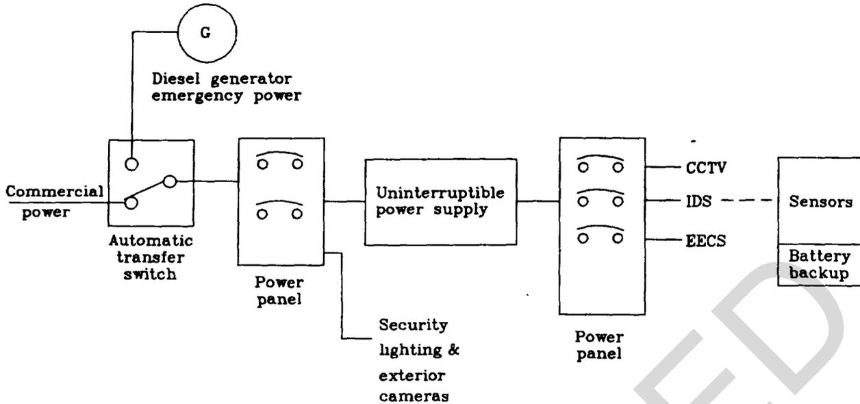
Figure 10-1 Electronic Security System Electrical Power Block Diagram
