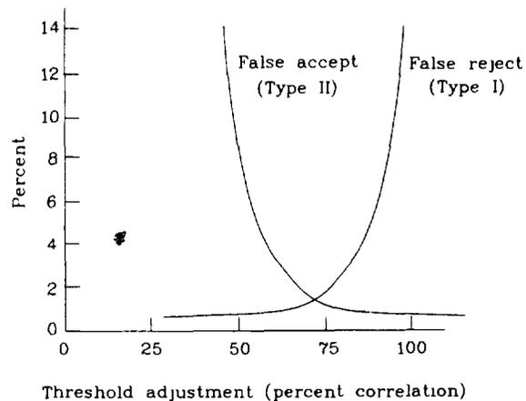
Figure 7-3 Biometric Device Error Rate Curves
