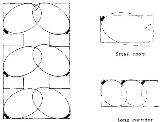
Figure 4-12. Placement of Ultrasonic Transceivers.
