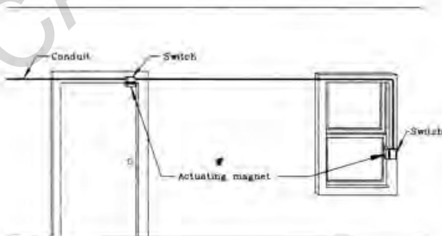
Figure 4-11. Typical Balanced Magnetic Switch Installation.
