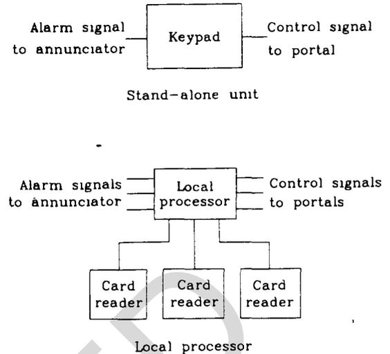
Figure 7-4. Local Equipment Configurations
