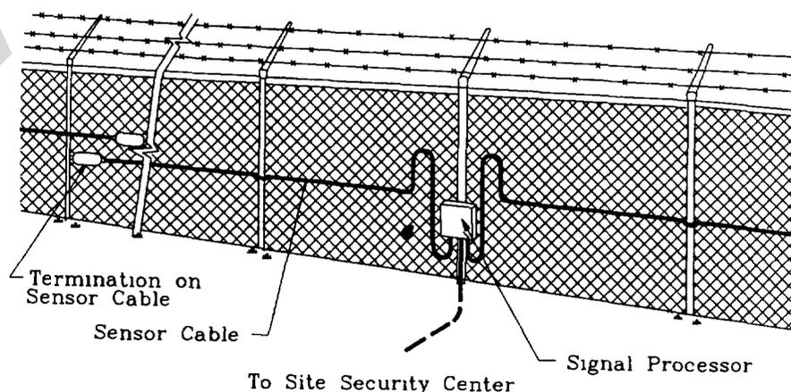
Figure 5-2. Typical Strain Sensor Cable Installation.
