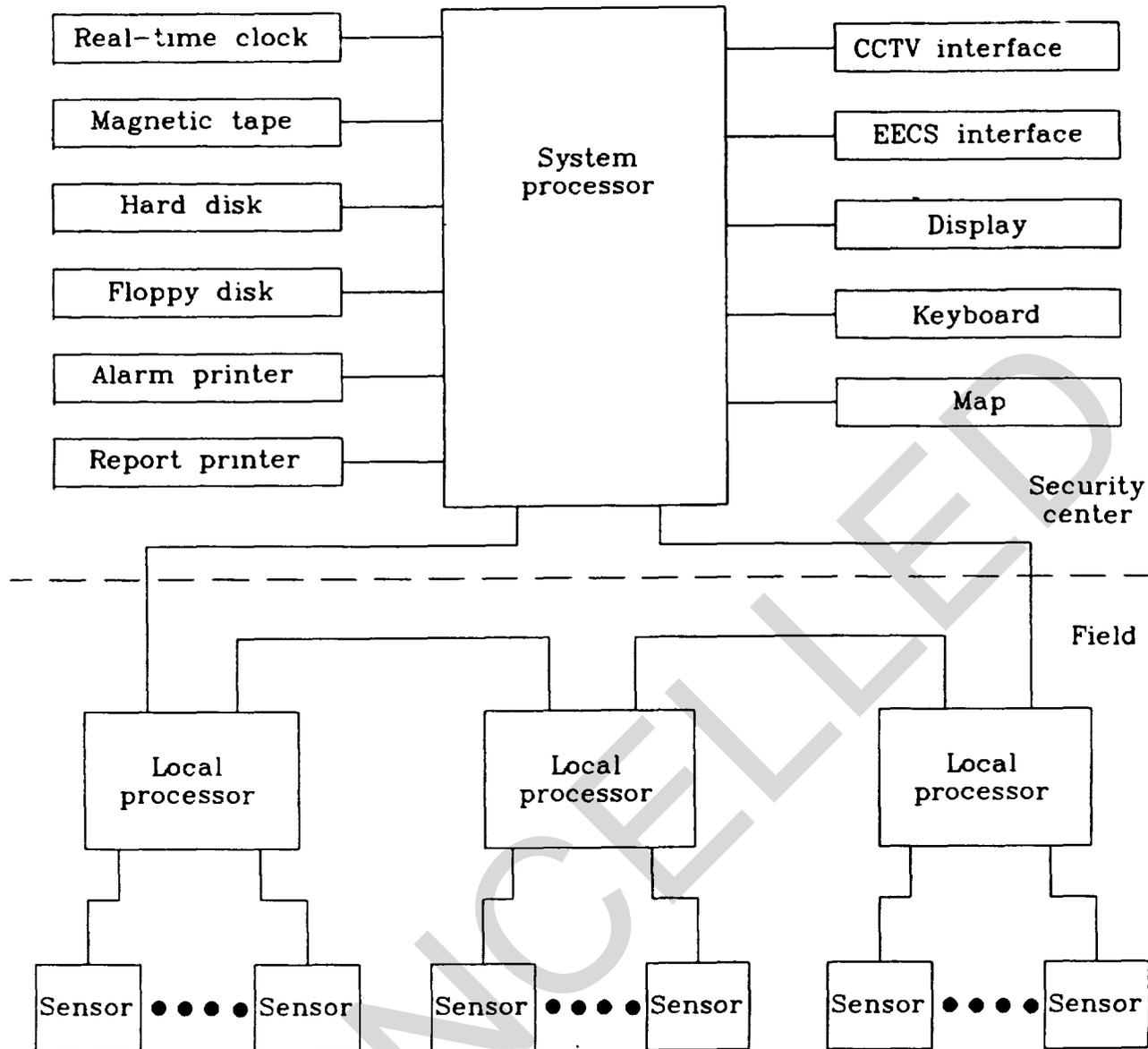
Figure 3-1 Typical IDS Configuration.
