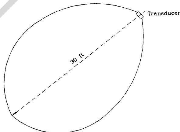
Figure 4-2. Typical Passive Ultrasonic Sensor Detection Pattern
