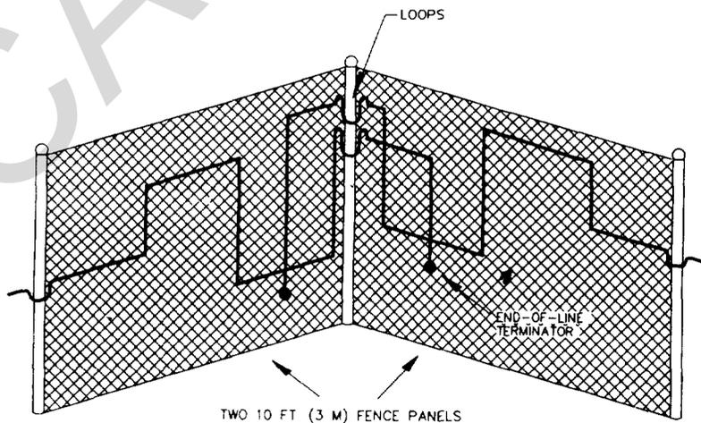
Figure 5-11 Use of Strain-Sensitive Cable Around Corners
