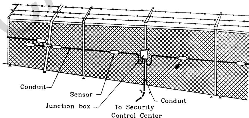
Figure 5-1. Example of Mechanical Fence Sensor Installation
