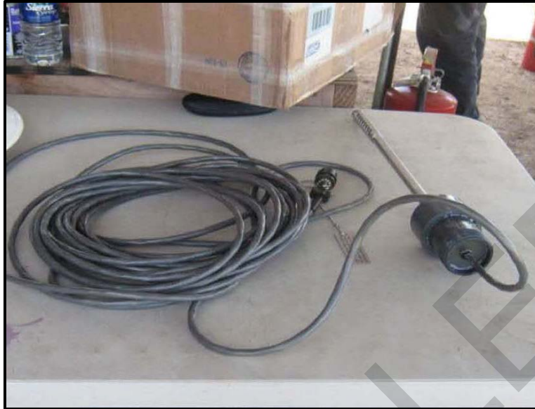
Figure B-16 Probe with Encapsulated Connector.
