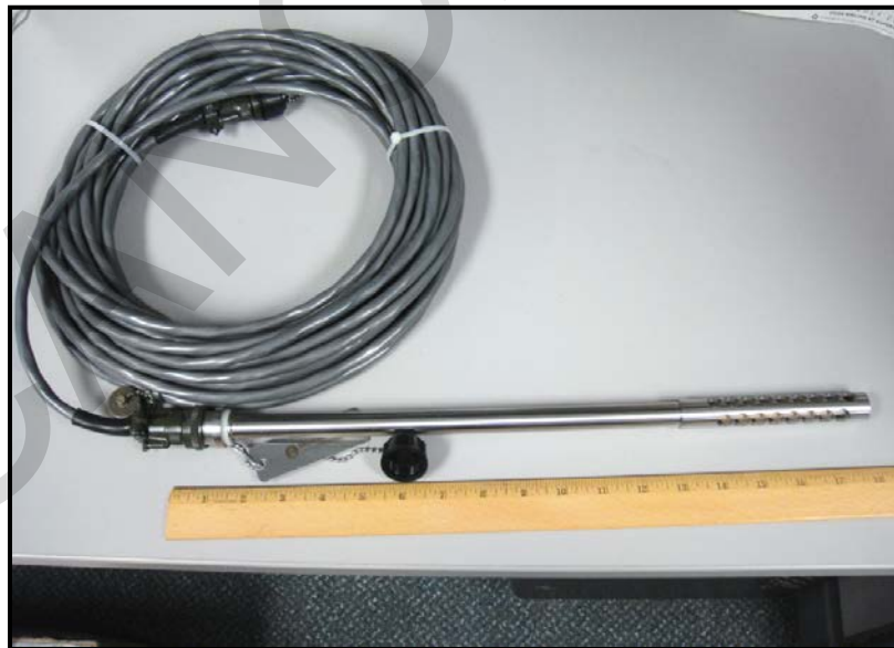
Figure B-15 Example of an ER Probe
