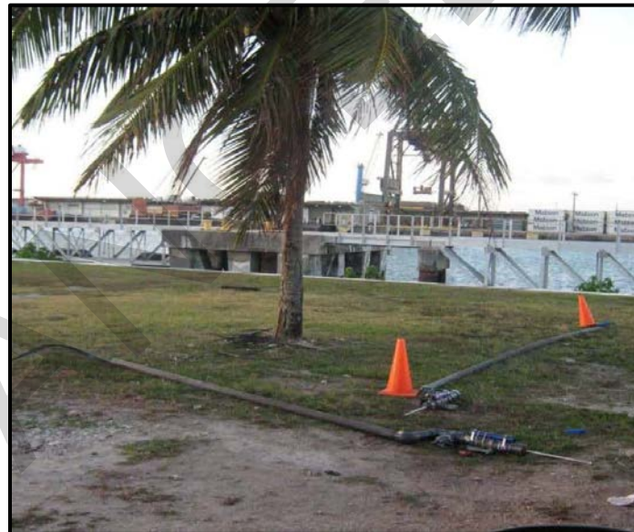
Figure B-17 Pre-Assembled Conduit System, Probe, and PRC for Submerged Use.
