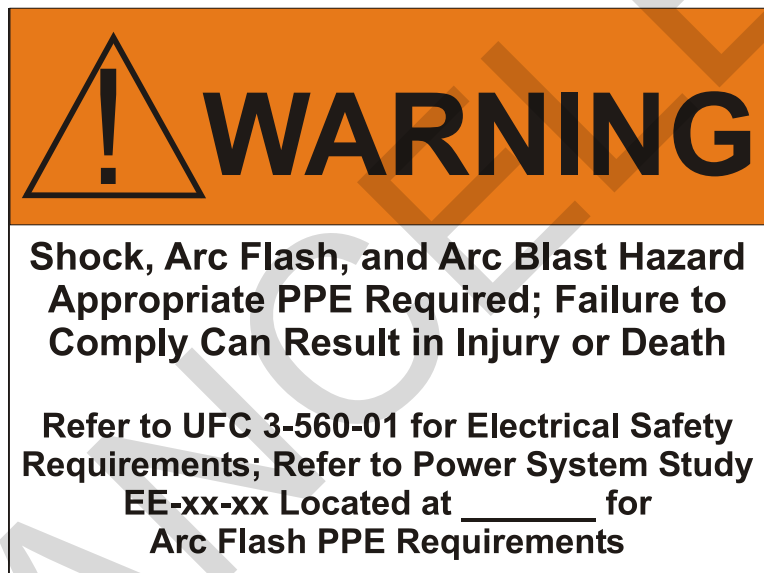
Figure 1-9 Arc Flash Warning Label Referring to a Separate Calculation
