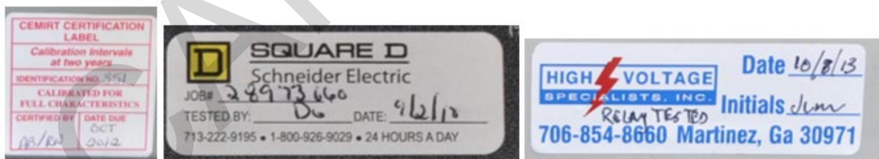
Figure 1-5 Typical Calibration or Maintenance Stickers
