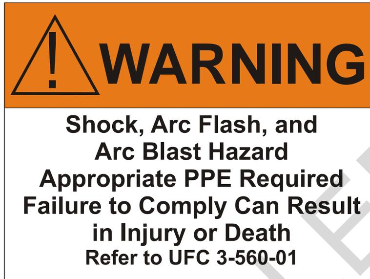
*Note: As part of the original development of UFC 3-501-01, Electrical Engineering, and UFC 3-560-01, Operation and Maintenance: Electrical Safety, the Tri-Service Electrical Working Group (TSEWG) deliberately specified general arc flash warning labels rather than the detailed arc flash warning labels specified by NFPA 70E. The detailed label information specified by NFPA 70E was considered inappropriate for the following reasons:*
