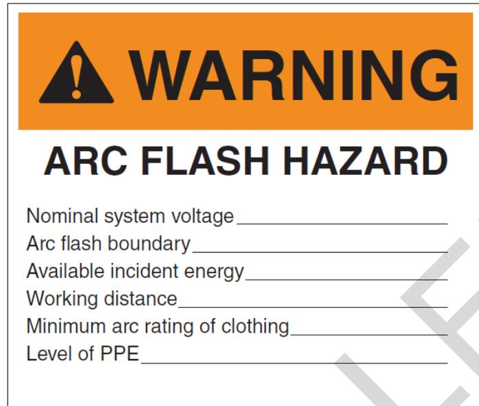
Figure 1-7 Typical Detailed Arc Flash Warning Label
