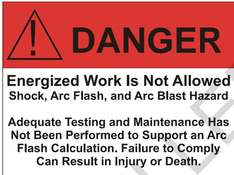
1-10.6 Arc Flash Label for Locations Identified to Be Greater Than 40 cal/cm<sup>2</sup>.
