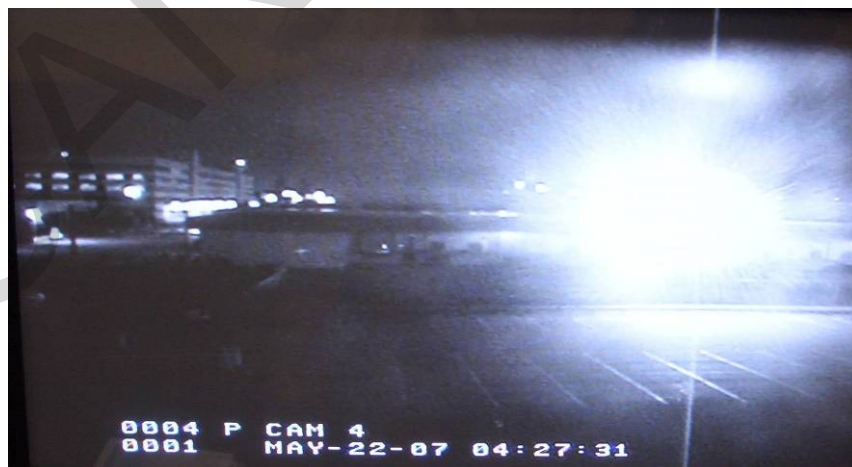
Figure 6-6. CCTV camera's view of scene with excessive glare.
