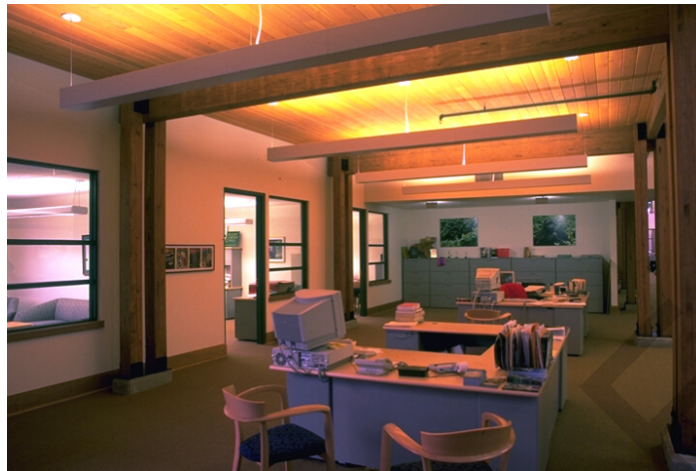
Figure 2-3. Minimize direct glare with indirect lighting.
