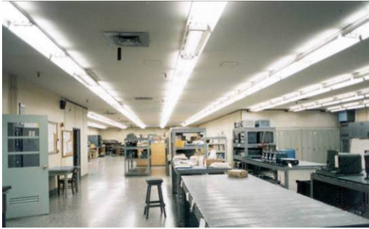
Figure 2-1. Examples of direct glare.
