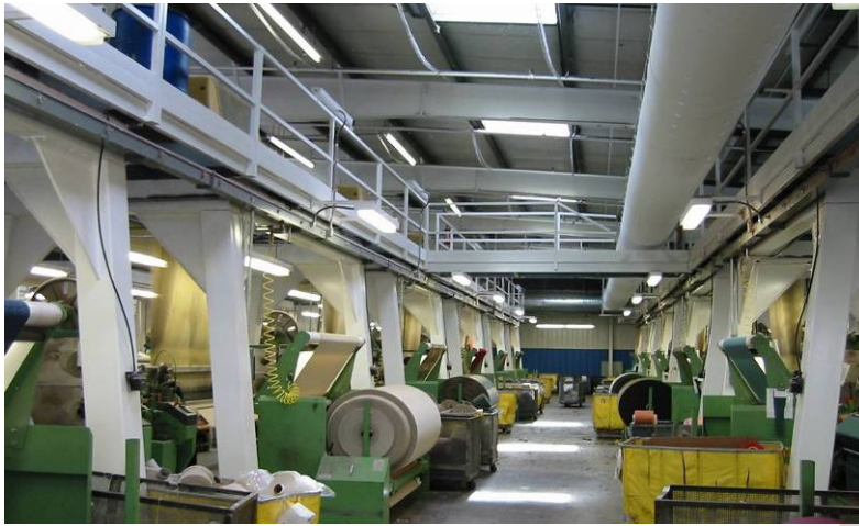
Figure 4-6 Examples of Toplighting Applications.
