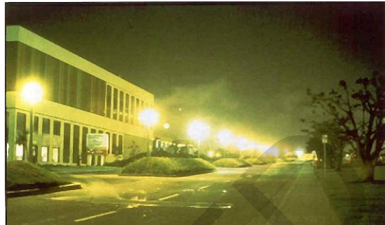
Figure 2-1. Examples of direct glare.
