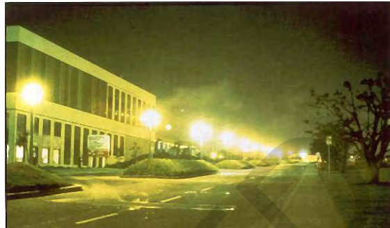
Figure 2-1. Examples of direct glare.
