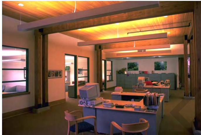
Figure 2-3. Minimize direct glare with indirect lighting.
