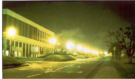
Figure 2-1. Examples of direct glare.
