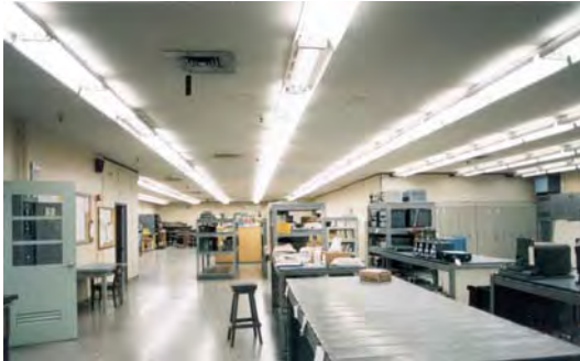
Figure 2-1. Examples of direct glare.
