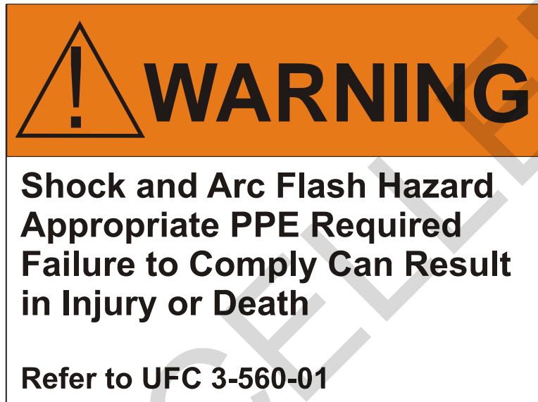
Figure 2-1 Typical Arc Flash Warning Label
